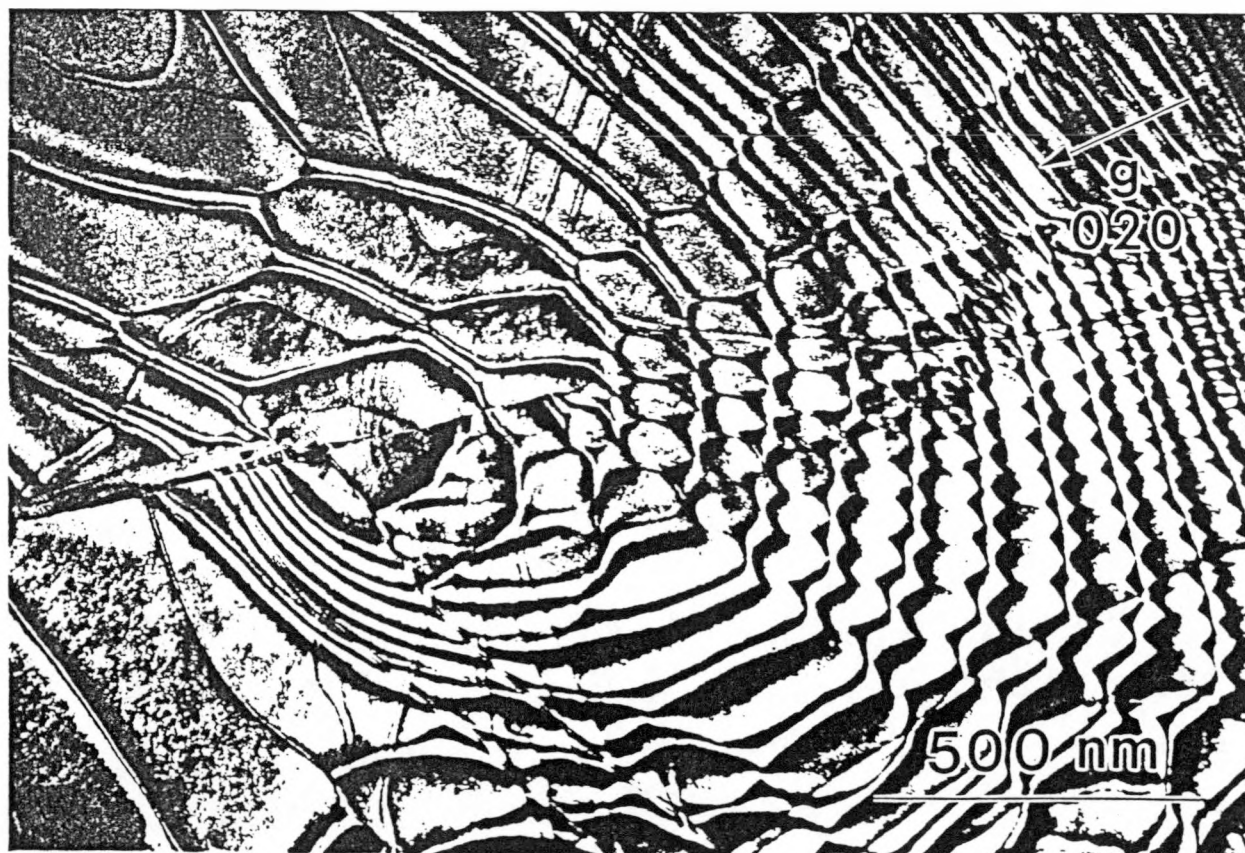
Figure 2. TEM micrograph of dislocations introduced into a 2212 single crystal by bending.
