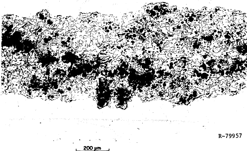
Fig. 23. Meat Microstructure of Plate CSI-202, at 97% Bu.
