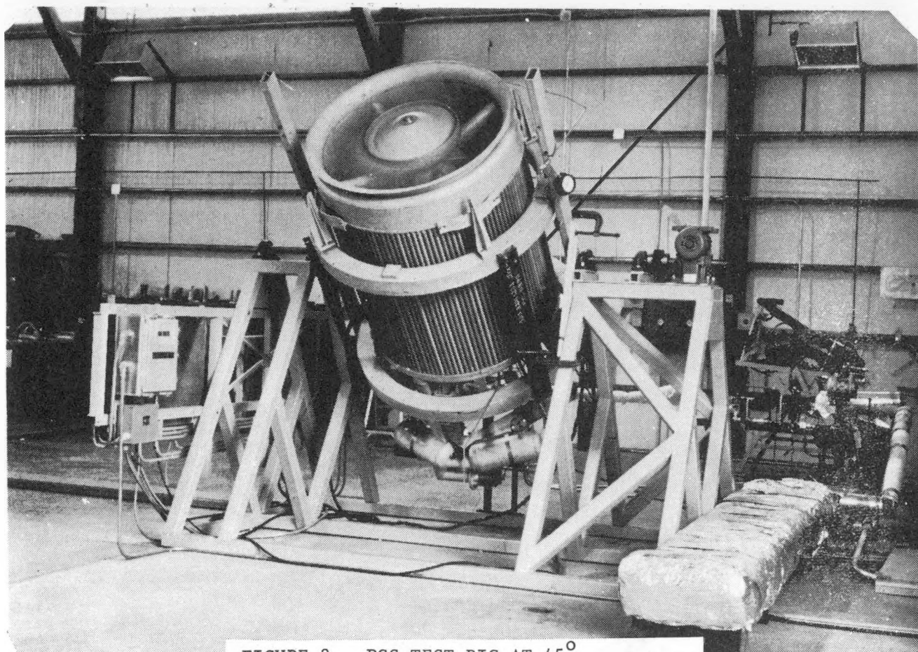
FIGURE 3. PCS TEST RIG AT 45^{\circ} ELEVATION ANGLE
