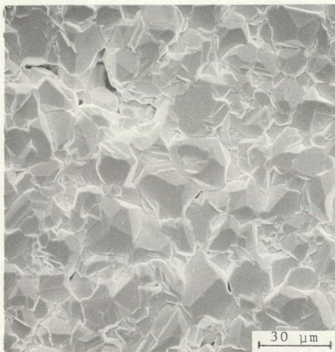
Figure 2 As-deposited surface of a cadmium telluride film of about 20 \mu\text{m} thickness on a tungsten/graphite substrate showing pinholes in the film.
