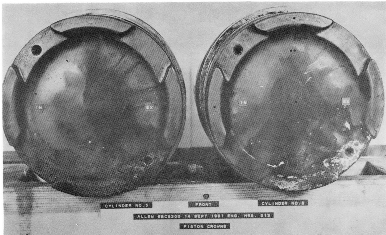
Figure 5-18. Condition of Piston Crowns After Endurance Tests
