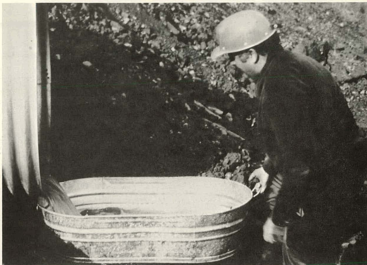
Fig. 7. Measuring Flow Rate at Sampling Site 4
