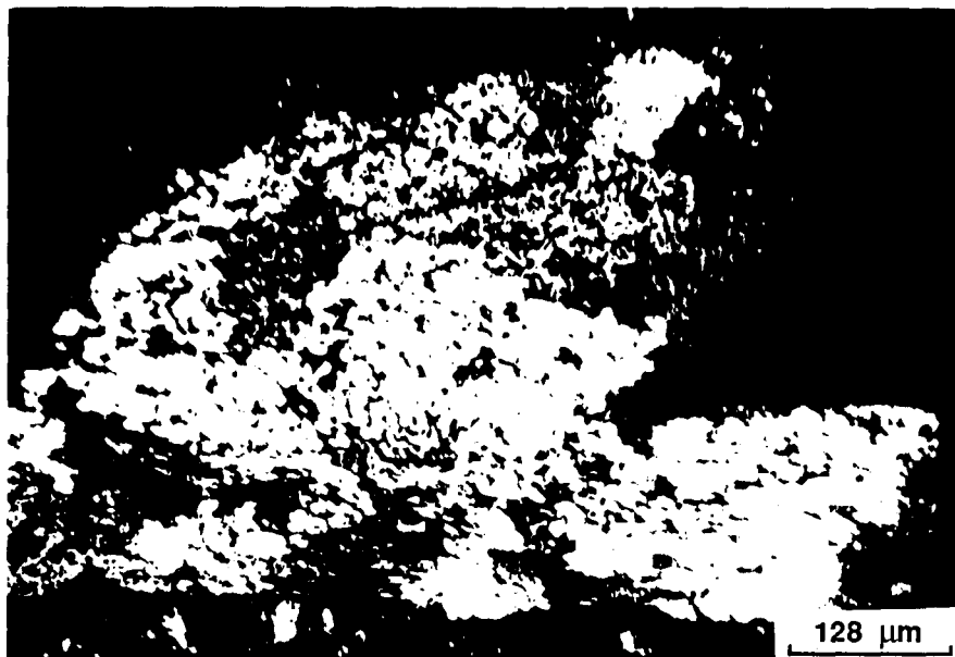
Figure 4.6 - Same Phase III particle as Figure 4.5, but under crossed nicols to demonstrate anisotropy.
