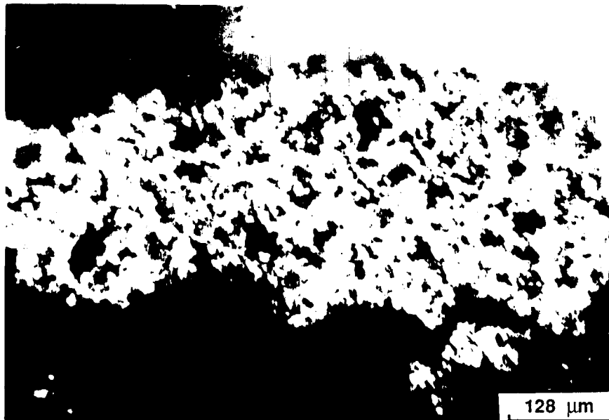
Figure C.1 - Matrix material found in the P71-2 residue is observed in negative relief in contrast to the high-reflecting Phase II material.
