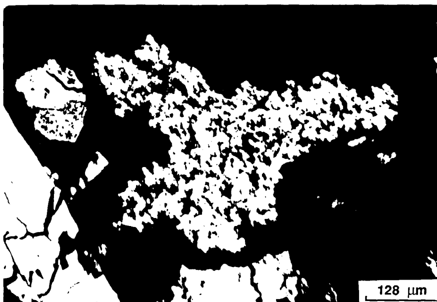
Figure 4.4 - Phase II material observed in P71-1 is a highly reflecting aggregate of 1-5 micron diameter spheres which form in loose, open clusters.
