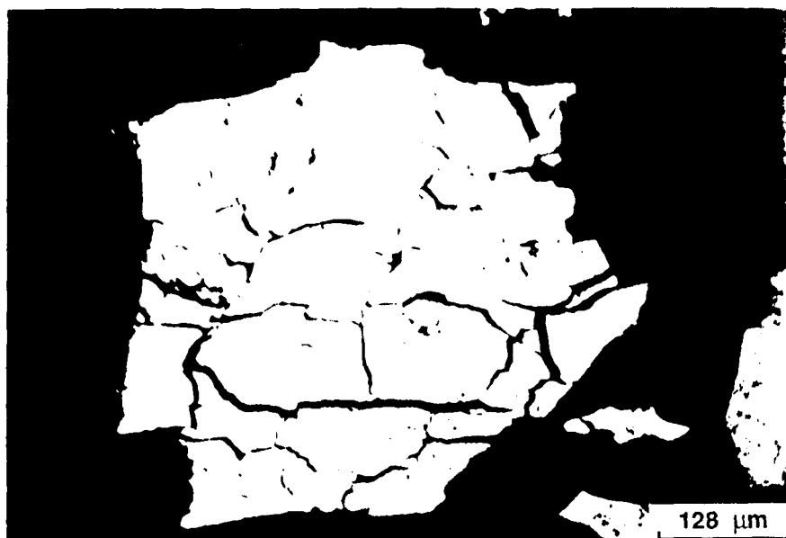
Figure 4.3 - A dominant component of P71-1 residue, Phase I occurs as a broad, angular particle of relatively low reflectance.
