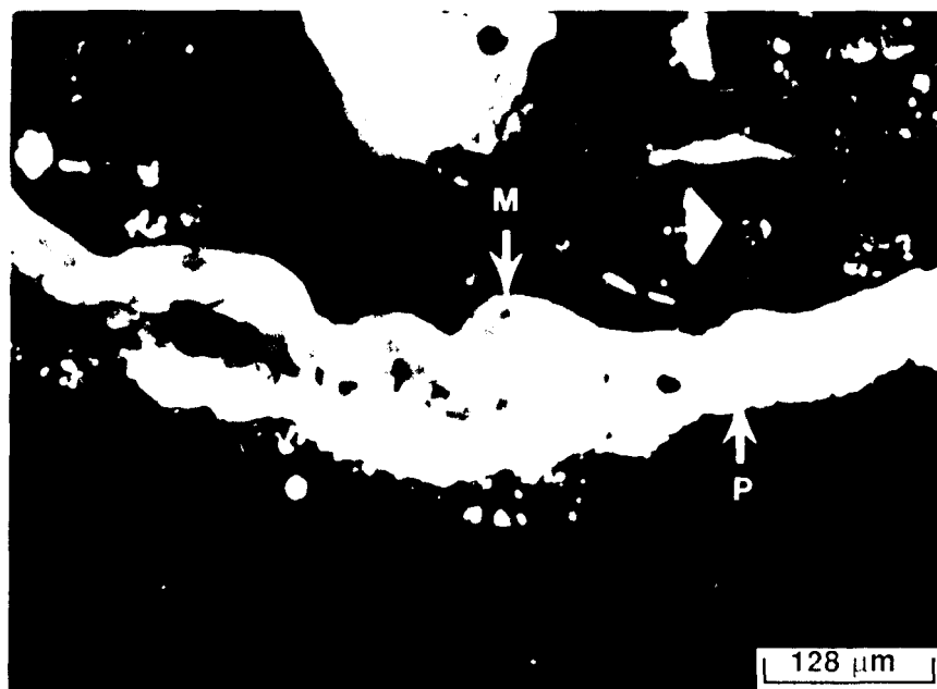
Figure 4.16 - Reflected-light photomicrograph of mesophase-derived carbon (M) on coarse pyrrhotite (P) in P73-G2-R2.
