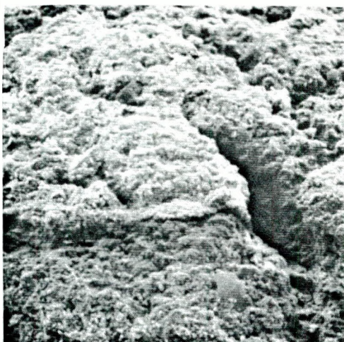
Figure 4.1. Scanning Electron Micrograph Showing the Rough and Fissured Exterior of a Zeocarb Granule (magnification 70 times)
