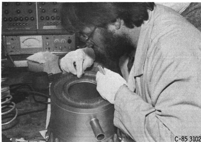
Figure 9. - Assembly of SPDE molten salt heat exchanger.
