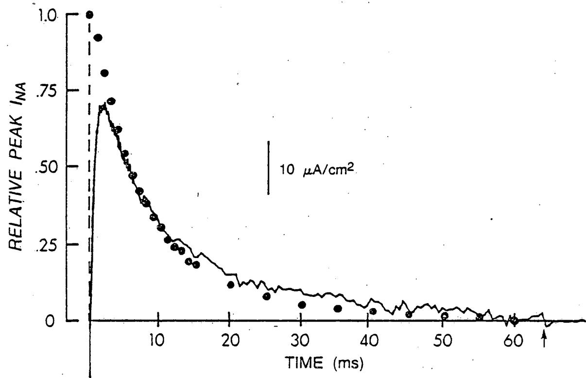
Figure 12. Collected double pulse inactivation and current decay data for three axons. Time constants were obtained from exponential fits to the decay phases of the currents and to the double pulse inactivation curves after the initial lag. 1/4 Na, 1/2 K, 1 mM 4-AP for all axons. Experiments performed at 3.2 - 3.6<sup>0</sup>C.
