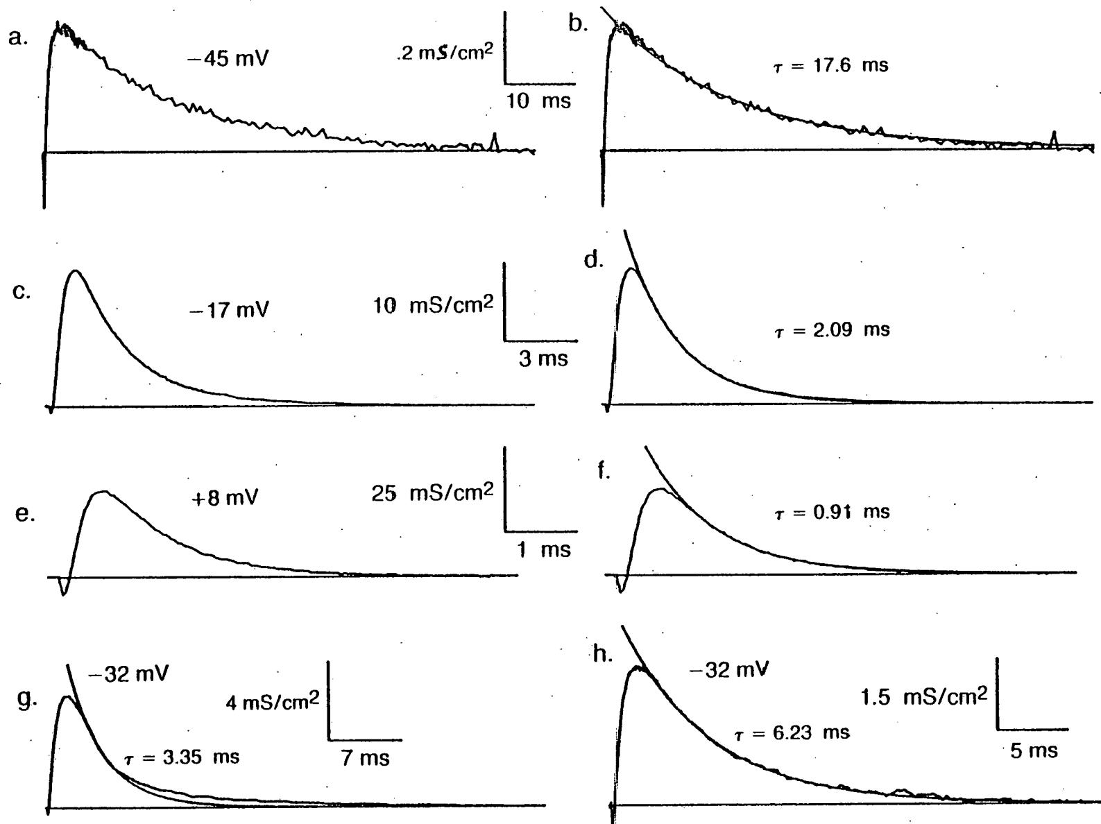
and -30 mV exhibited biphasic decay. Figure 8g shows a relatively severe example. However, the degree of deviation from a single exponential varied from axon to axon and in axons with the best spatial uniformity characteristics the deviation was usually quite small. An example is shown in Figure 8h. It seems likely, therefore, that the deviation usually seen is due to spatial variations in membrane currents and is not an intrinsic property of the sodium channels.
