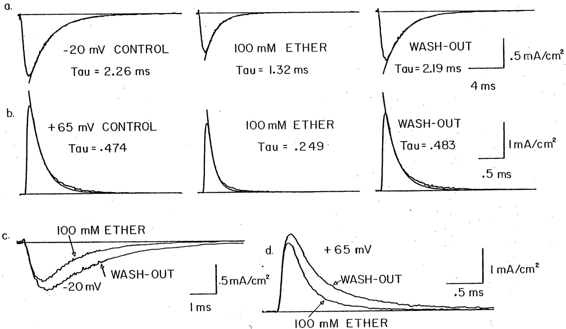
Figure 3. Decay time constant as a function of membrane potential before, during, and after 100 mM ether. Ether was applied for 9 minutes and rinsed for 18 minutes. 1/4 Na, 1/2 K, 1 mM 4-AP. Differential current electrode. Holding potential -80 mV. Temperatures: Control, 3.1-3.5°C; 100 mM ether, 3.0-3.8°C; wash-out, 3.3-3.6°C. At most potentials, control, ether, and wash-out temperatures are matched to within .2-.3°C.
