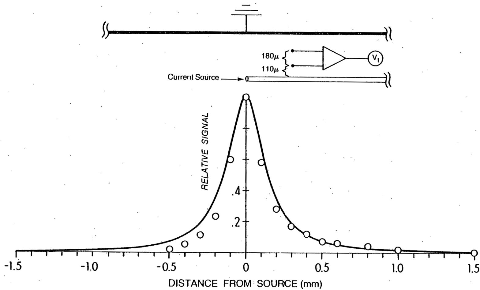
Figure 2. Spatial resolution of the differential electrode. The pipette current source was in the chamber in the position normally occupied by the axon, about 3 mm from the ground electrode and about  $100 \mu$  up from the floor of the chamber. Points give the recorded voltage signals normalized with respect to that recorded opposite the mouth of the pipette. The solid line is drawn according to
