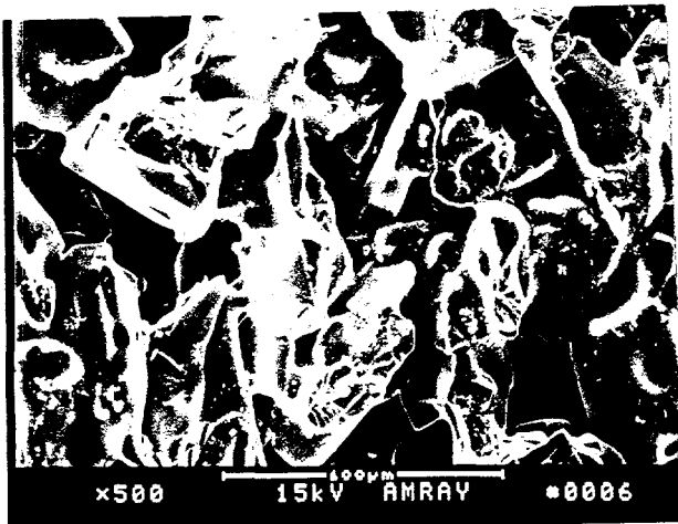
Figure 18 SEM micrographs of (a) outer and (b) inner layers of the unused ceramic filters showing microstructural features: particle's and pore's shape and size.
