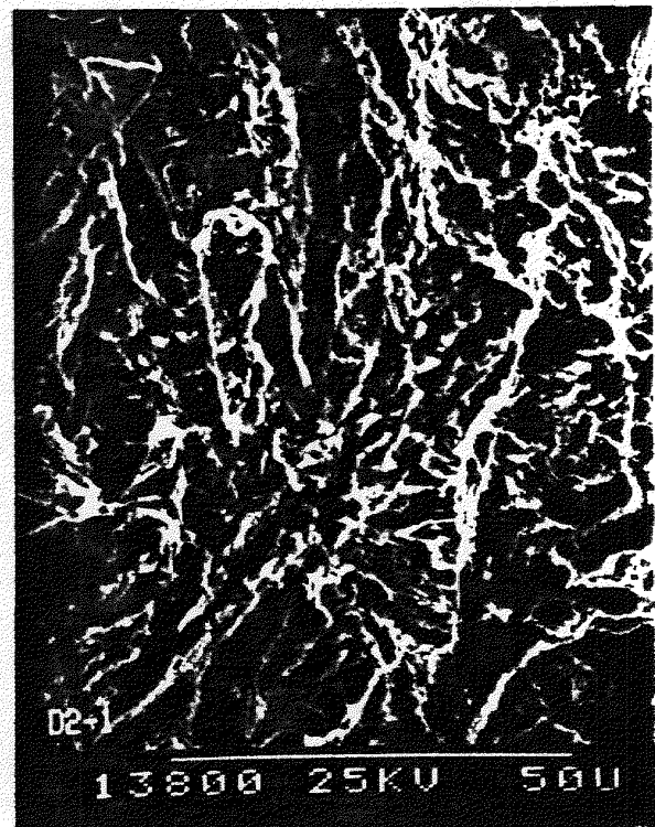
Figure 5. Secondary electron micrograph of transgranular fracture surface for PH 13-8 Mo modified with 1% Pd (H-1050) after slow strain rate testing.
