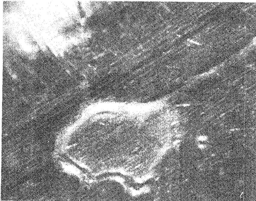
Figure 8. Flaw in contact surface could provide a leak path
