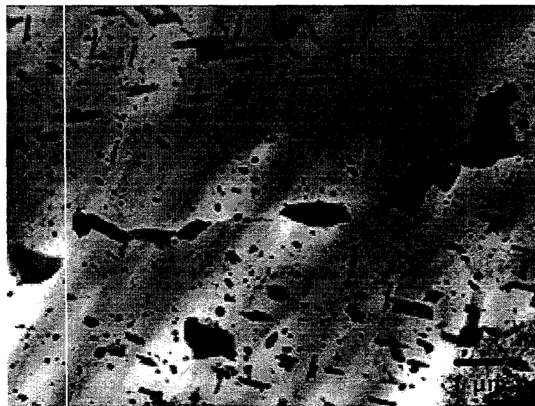
Figure 5. Bright field TEM micrograph of Al 2024 subjected to treatment 2.
