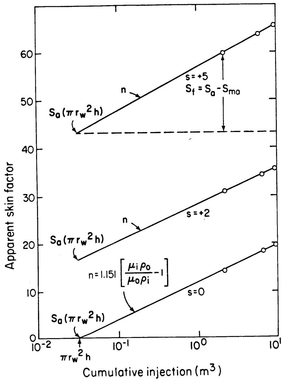
Figure 25. Apparent skin factors vs. cumulative injection for Example 4.
