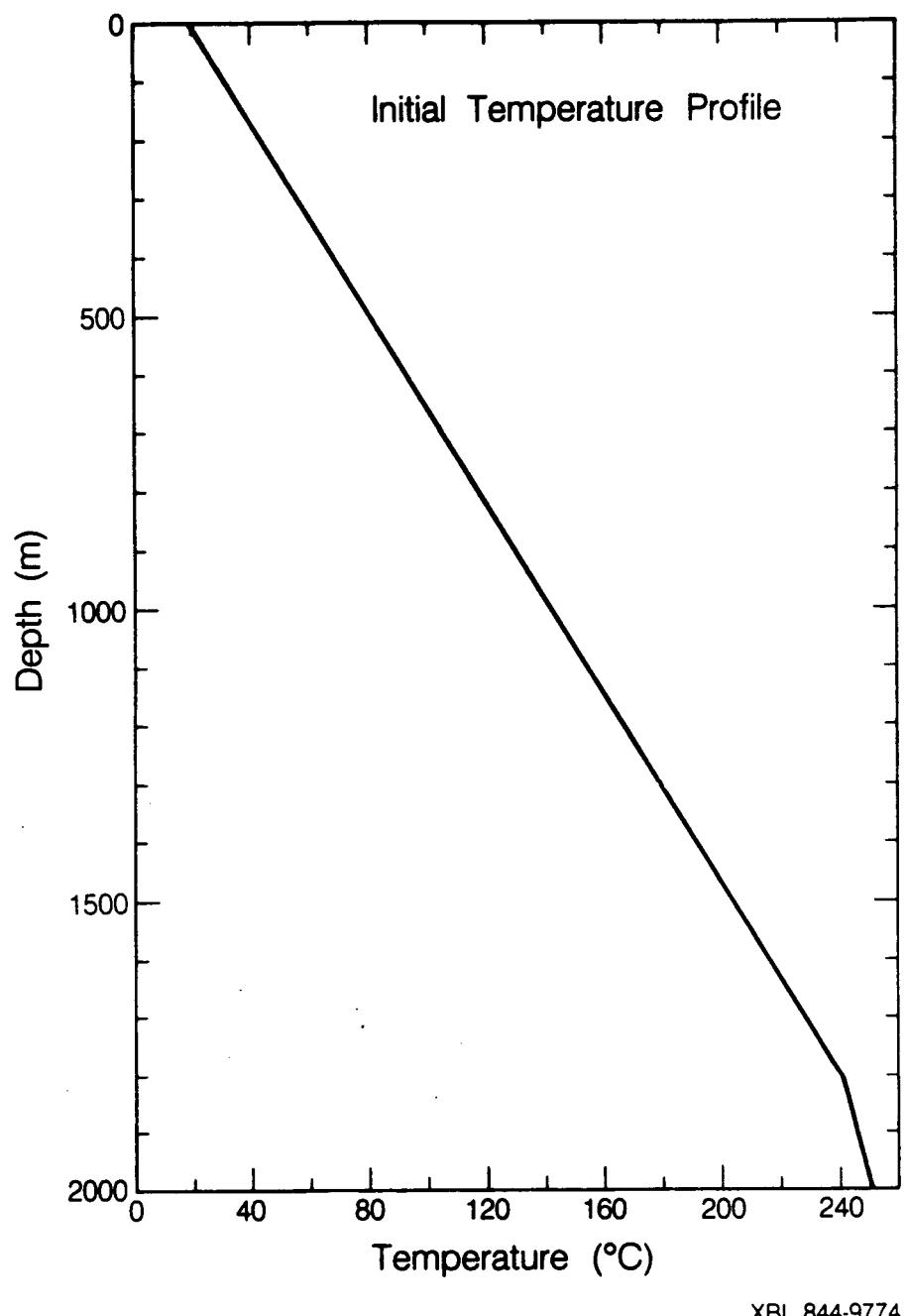
Figure 17. Initial temperature profile for the simulated wellbore-temperature transients.
