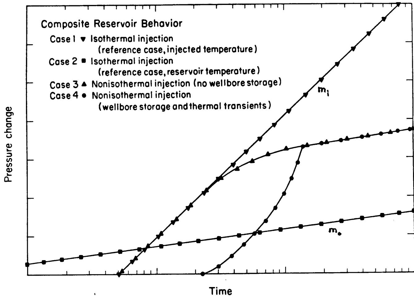
Figure 20. Schematic of the pressure transient response during moving-front dominated injection tests.
