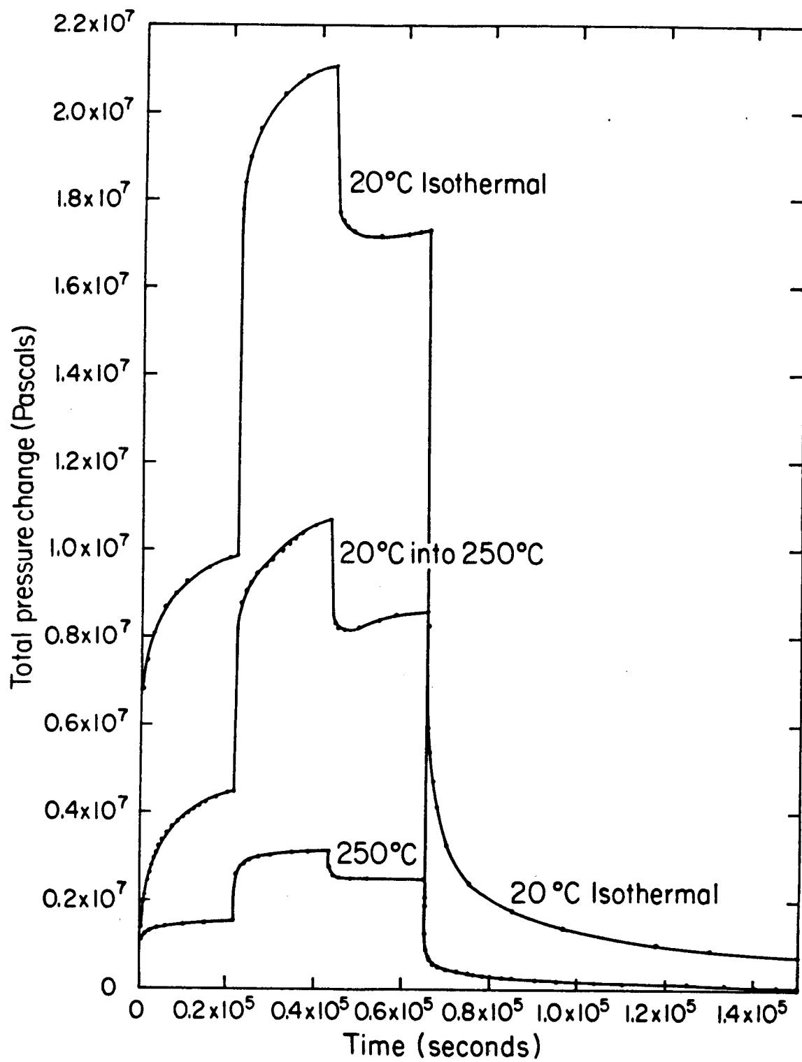
Figure 11. Simulated step-rate injection test.
