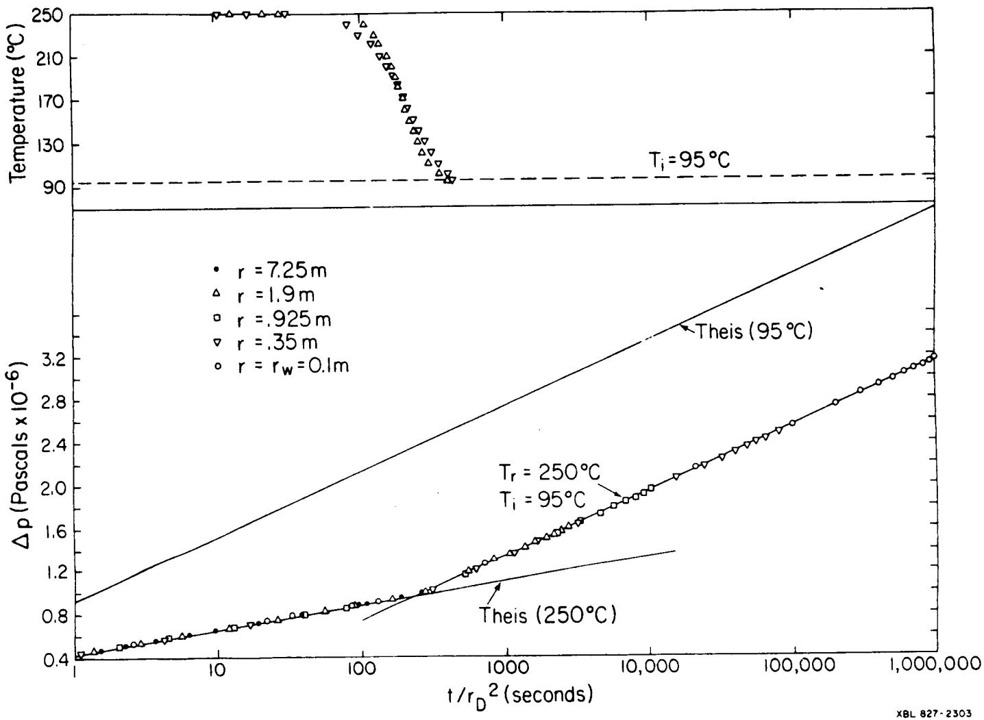
Figure 3. Pressure buildup during injection of  $95^{\circ}\text{C}$  water into a  $250^{\circ}\text{C}$  reservoir.
