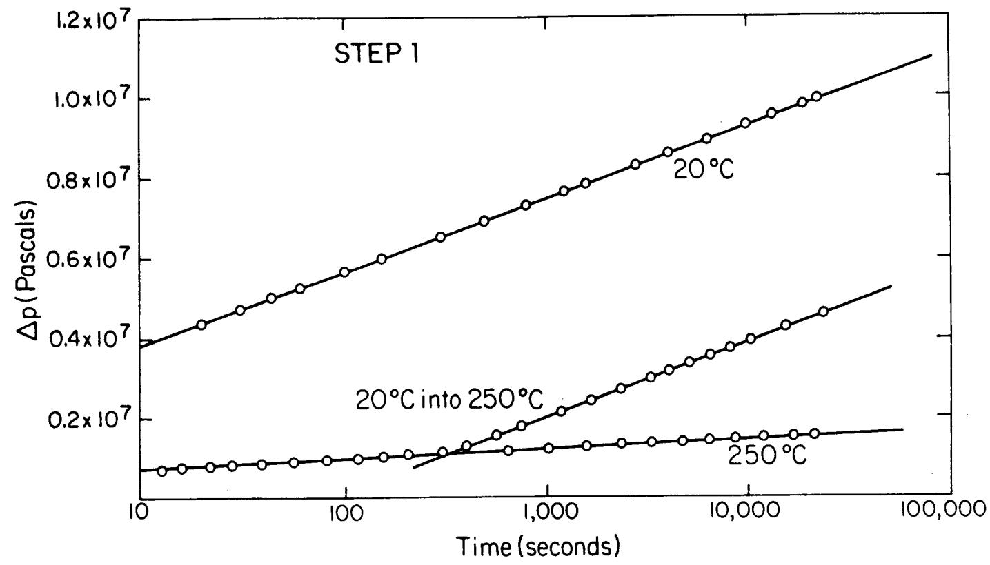
Figure 12. Pressure transient data for Step 1 of the simulated step-rate test.
