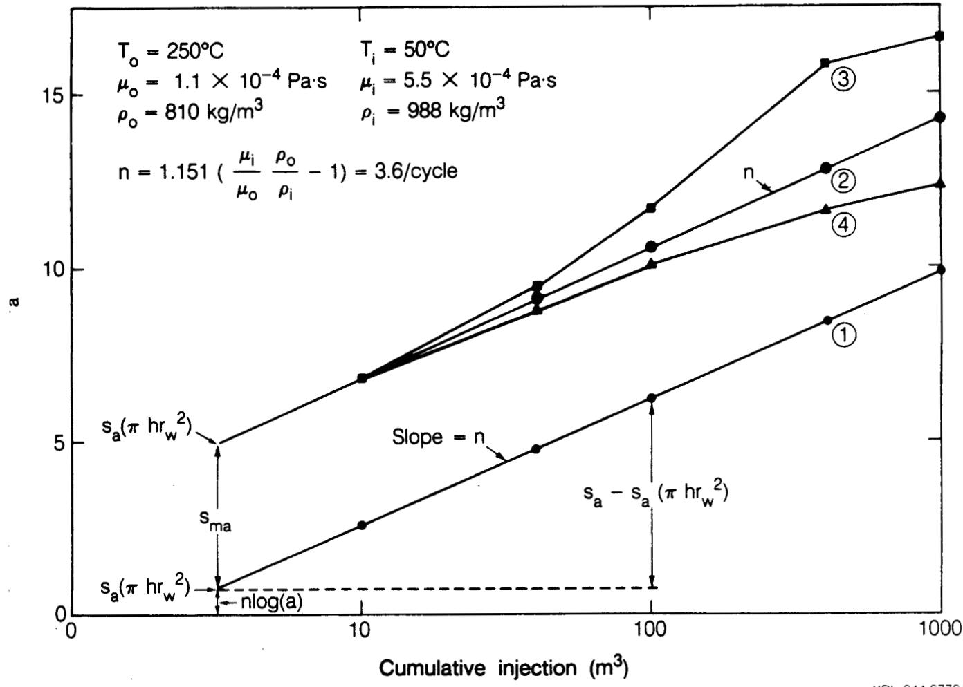
Figure 21. Schematic of the pressure transient response during composite-reservoir type injection tests.
