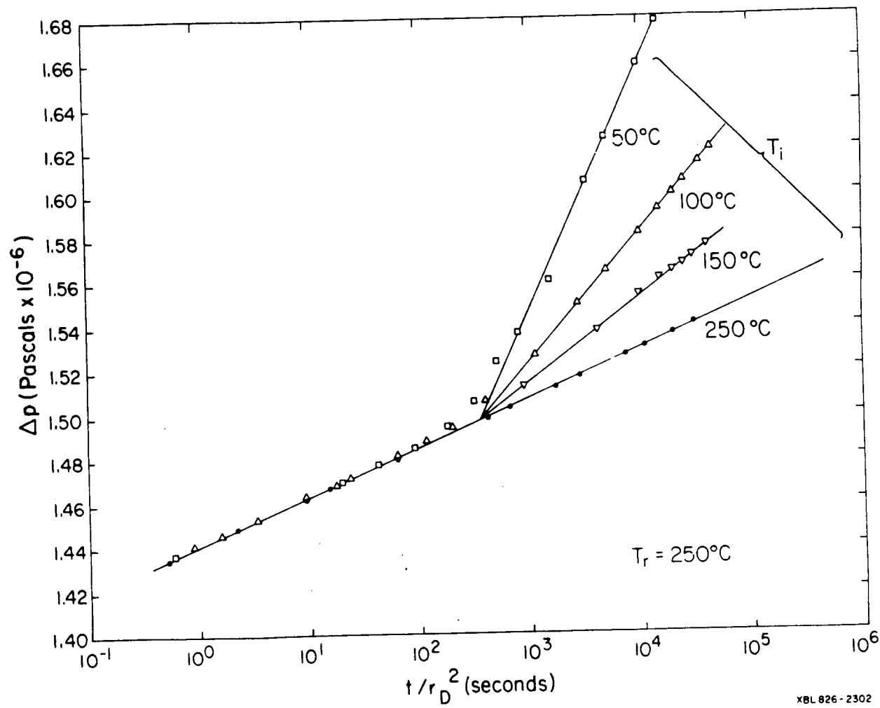
Figure 4. Pressure buildup at the well due to injection of 50°C, 100°C and 150°C into a 250°C reservoir.
