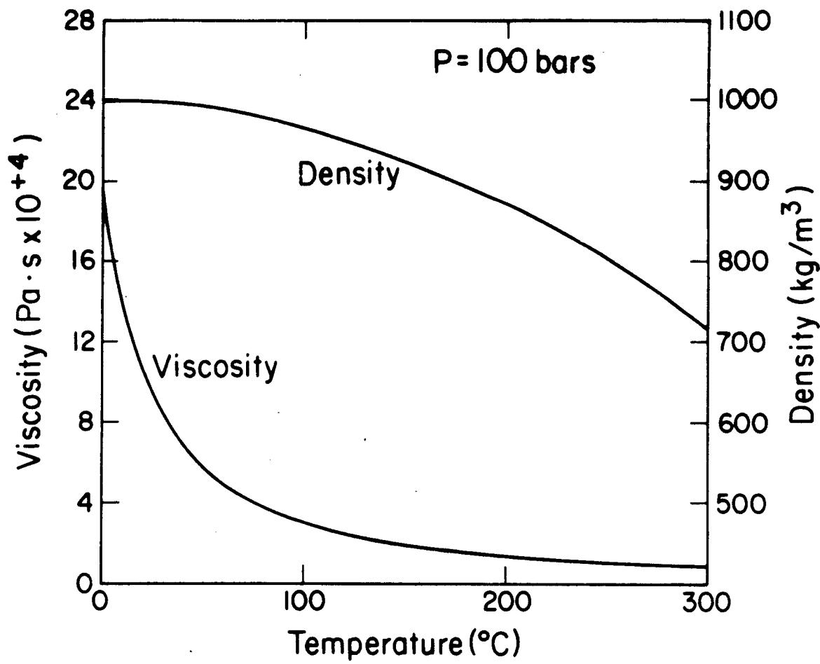
Figure 1. Viscosity and density of water as a function of temperature.
