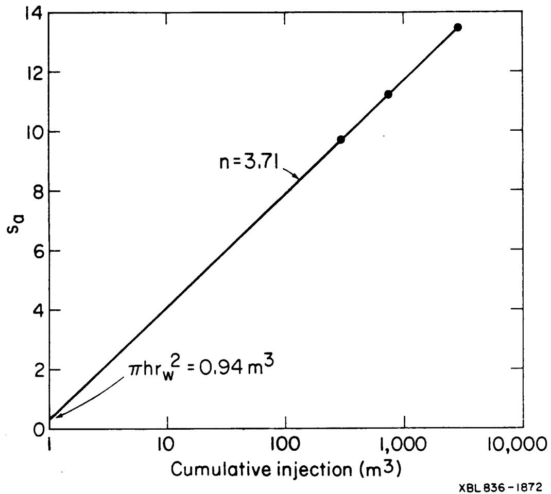
Figure 28. Apparent skin factors vs. cumulative injection for Example 6.
