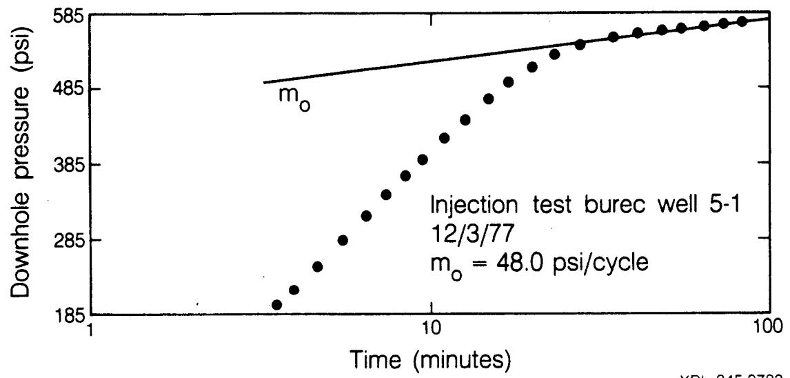
Figure 30. Pressure buildup data from East Mesa well 5-1.
