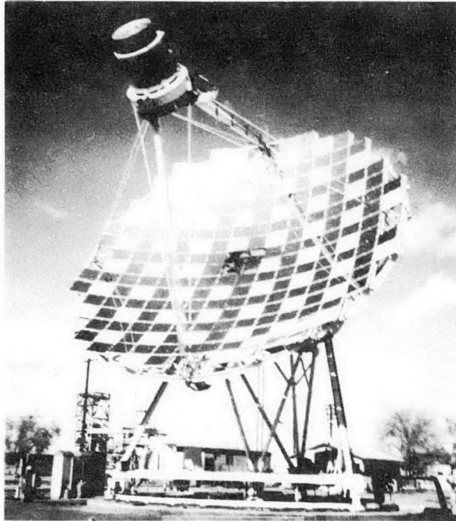
Figure 4-4. Test Bed Concentrator with 25% Checkerboard Masking Pattern
