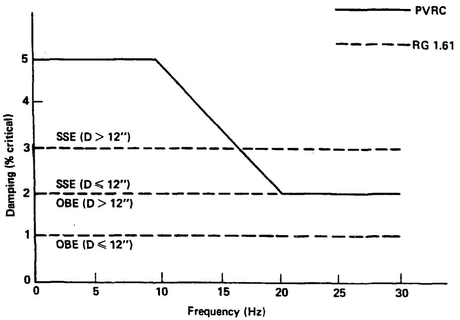
Figure 2. PVRC Proposed Damping vs. RG 1.61 Damping
