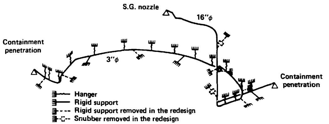
Figure 5. AFW Line inside Containment of a PWR Plant
