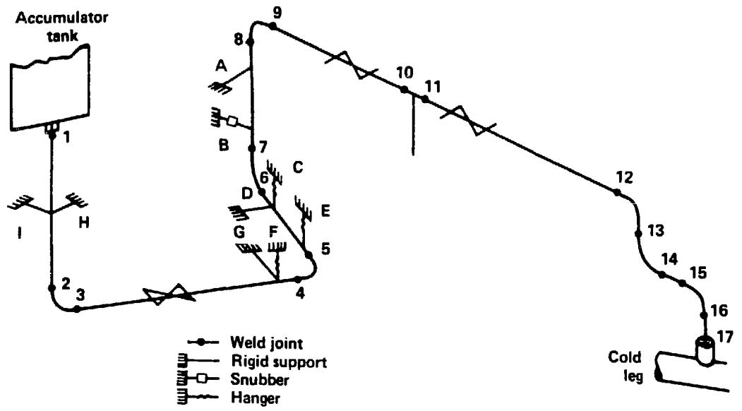
Figure 1. Safety Injection Line from a PWR Plant
