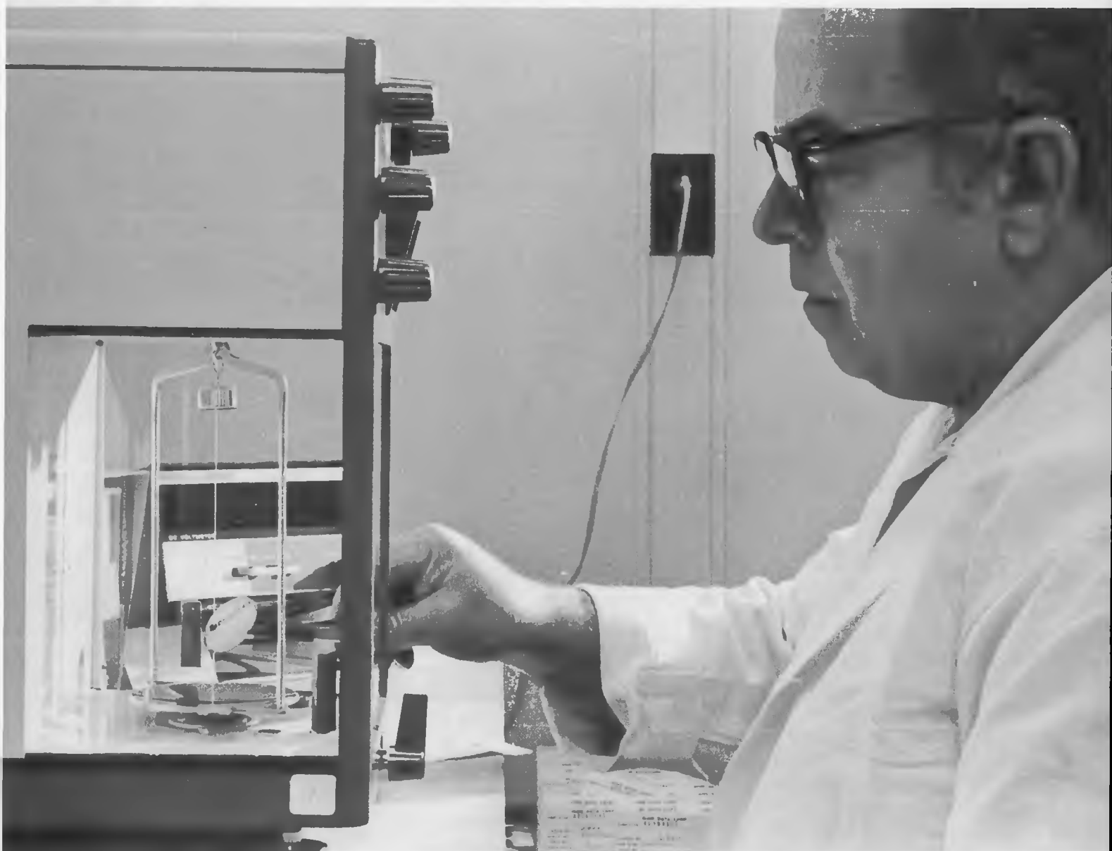
A sample of mine dust is weighed as one step in determining compliance with respirable dust standards.
