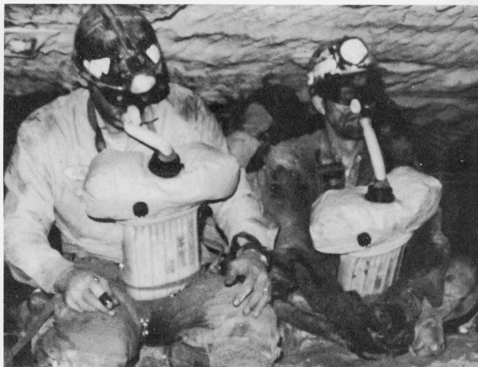
Miners in a low-coal mine don self-contained self-rescuers during an evaluation of the devices in the mine environment.
