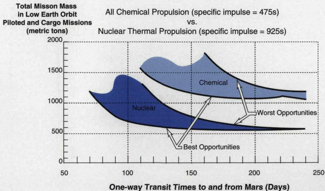
extended from 30 to 100 days at an increase of 100 to 200 metric tons in the initial mass to low Earth orbit during favorable years.
