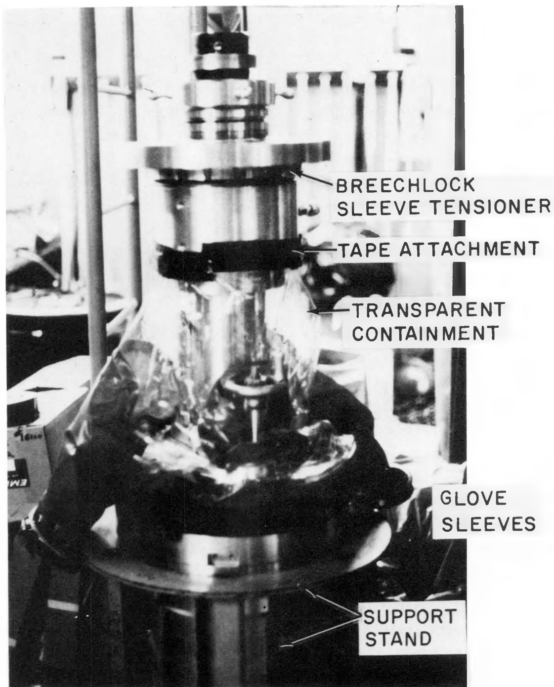
Figure A2-16. Breechlock Sleeve Tensioner in Top Part of Three-Part Containment
