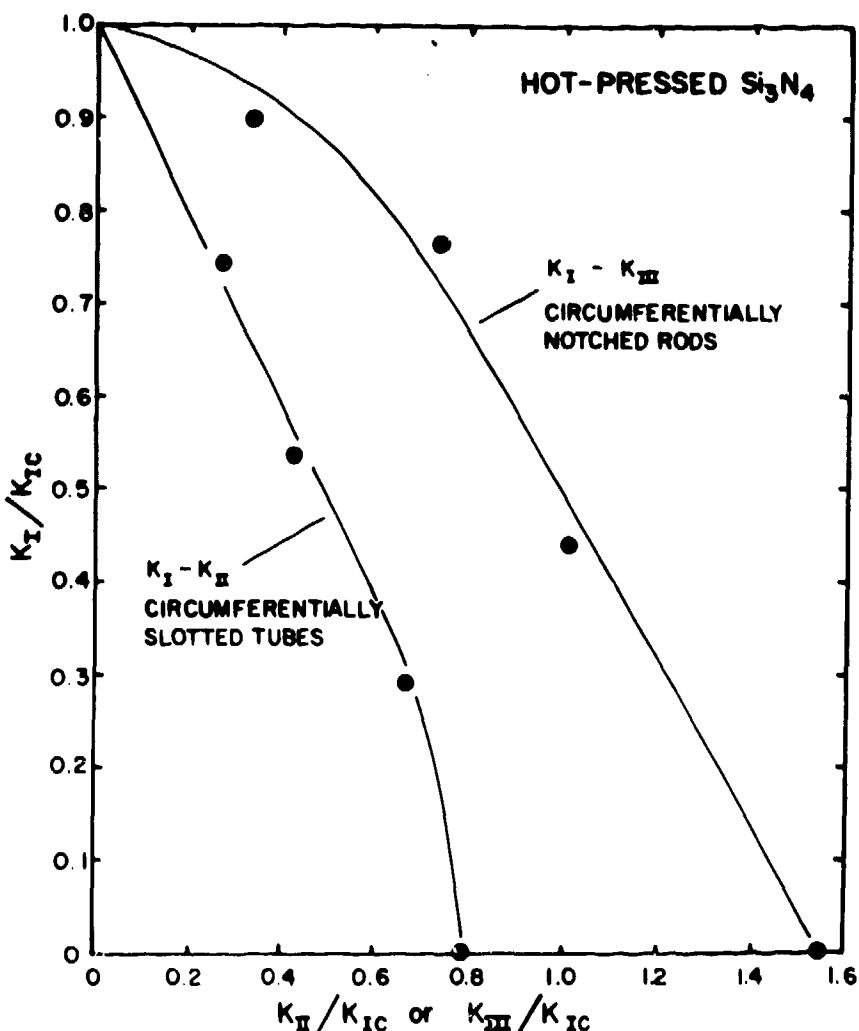
FIGURE 4: Mixed-Mode Fracture of Large Cracks in Hot-Pressed  $\text{Si}_3\text{N}_4$ .
