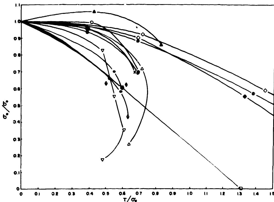
FIGURE 3: Mixed-Mode Fracture Results for Indentation Surface Flaws.
