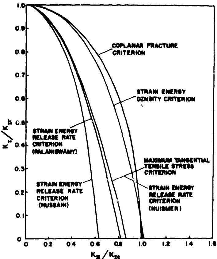
FIGURE 2: Predictions of Theoretical Mixed-Mode Fracture Criteria.
