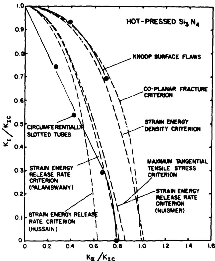
FIGURE 5: Comparison of the Mixed-Mode Fracture of Circumferentially Slotted Tubes and Annealed Surface Flaws in Hot-Pressed  $Si_3N_4$ .
