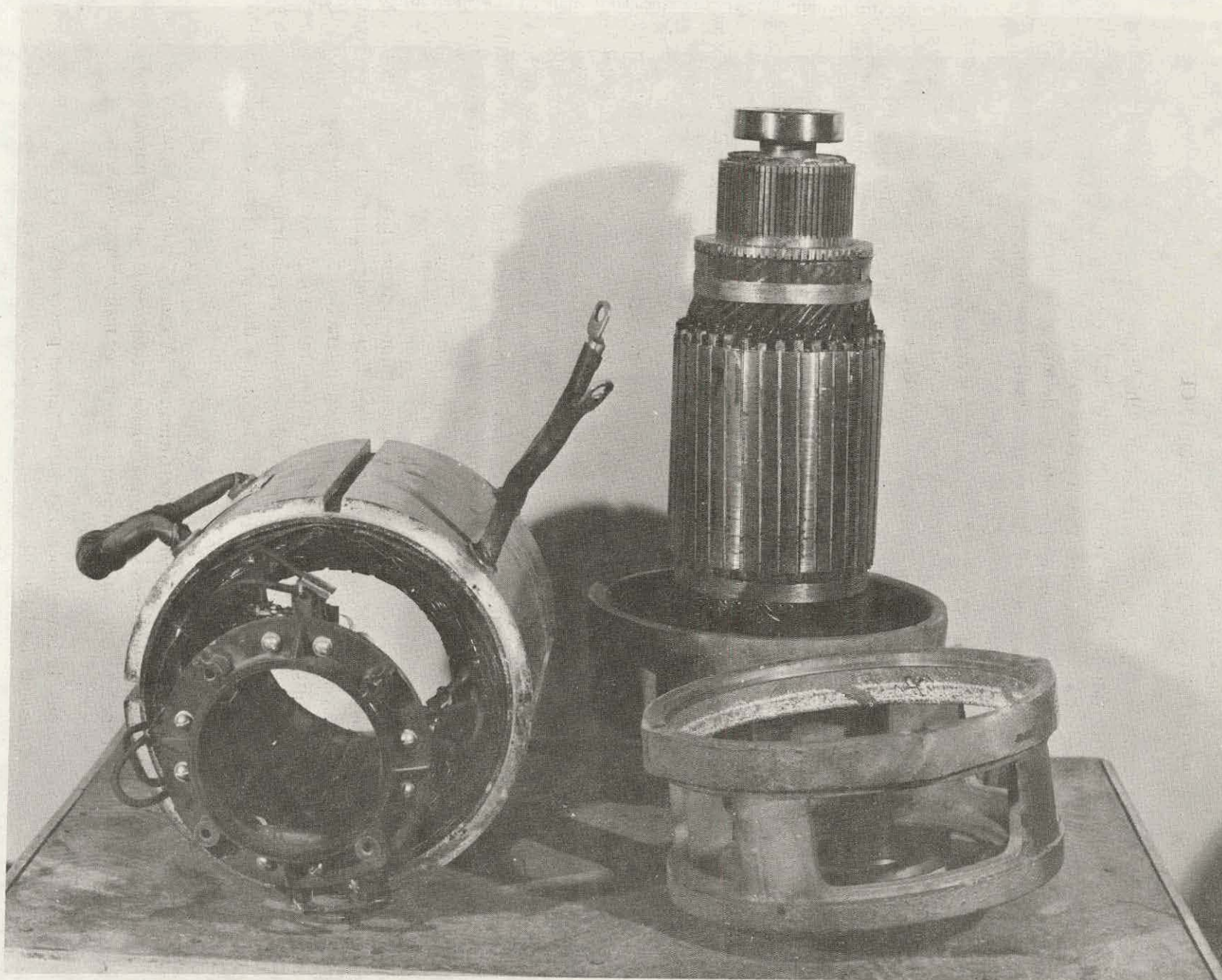
Figure 6.6. Overall view of motor damage caused by disintegration of soft solder joints.
