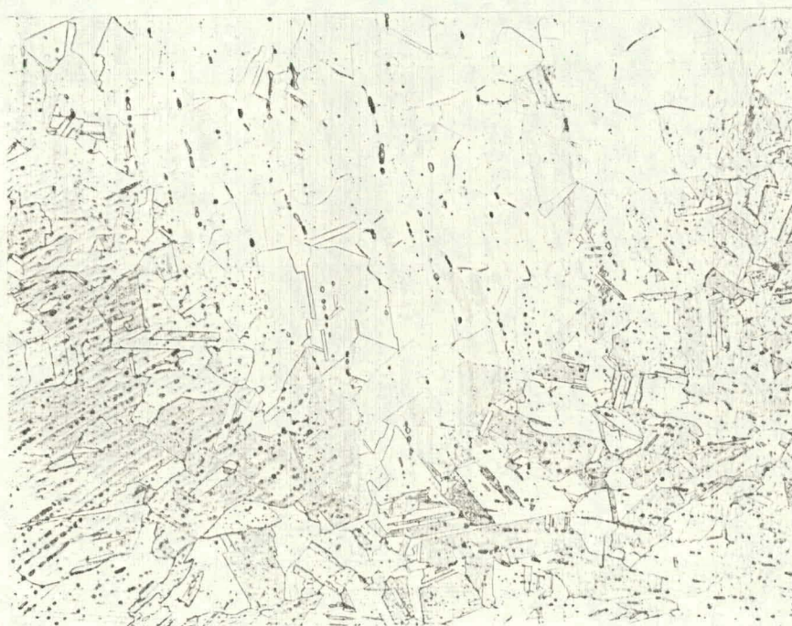
(B) The transformed equiaxed austenitic grain structure shows short dark streaks of the transformed ferrite and stringers of inclusions, carbides, etc. in the fusion zone. The HAZ shows \gamma grains, annealing twins and stringers.
