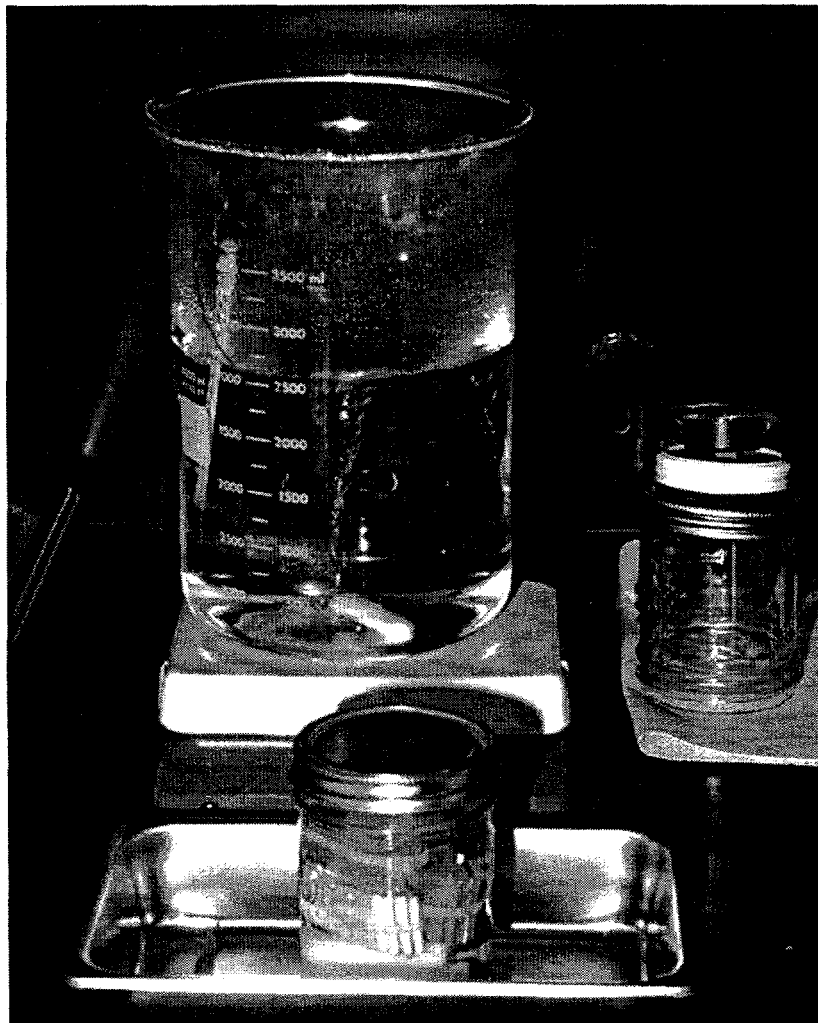
Fig. 2. Exposure cell containing five liner materials in lower portion of photograph.
