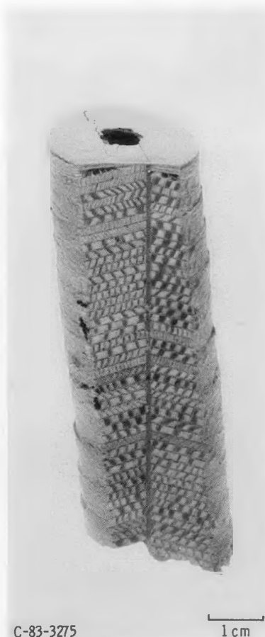
(d) Blade 1012 plug with crack at bond line and 1/4 in. away.
