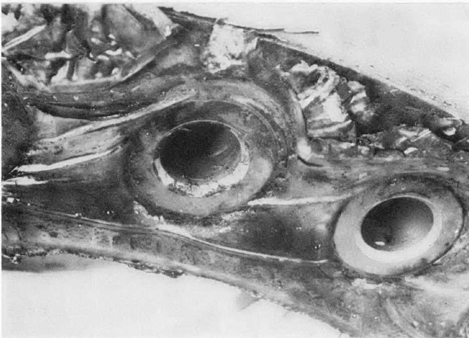
(b) Corrosion of face of spool piece.
