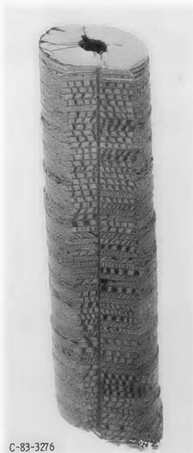
(c) Blade 1012 plug with crack at bond line.
