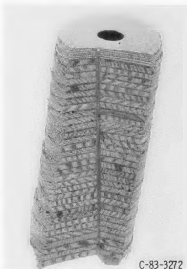
(a) Blade 1013 plug without cracked leading edge.
