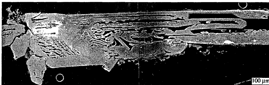
Fig. 4: Cross-section of a large crystal from a Deposit 8 sample showing complex internal structure (40X).
