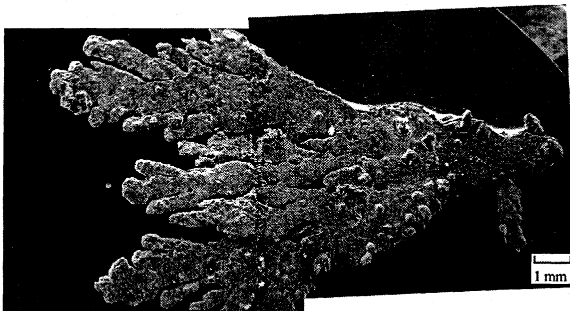
Fig. 8: Overview of a leaf-shaped dendrite from Deposit 30 (10X).
