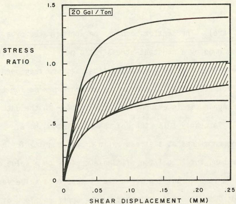
Figure 5. Direct shear results for 20 gal/ton oil shale. Stress ratio is the ratio of shear stress to normal stress. The shaded band is the envelope of all "slow" tests, while the solid curves are results of "fast" tests.
