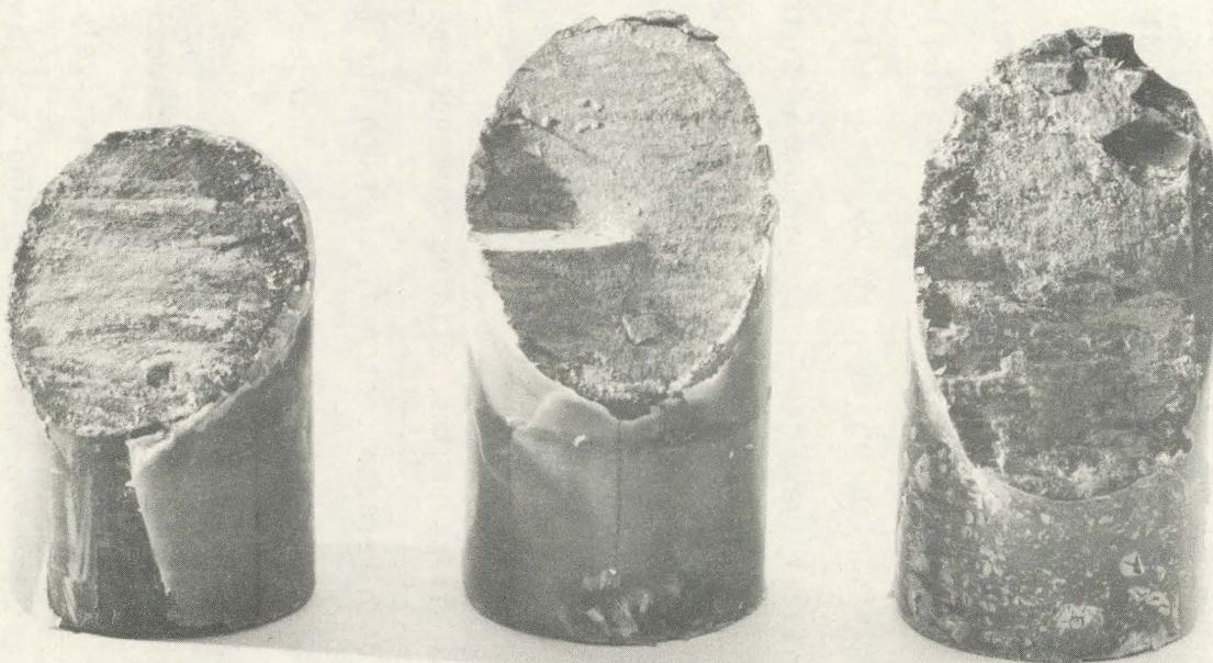
Figure 13. Representative joint surfaces after triaxial shear testing. Comparison with Figure 5 illustrates the greater degree of surface asperity crushing which occurs at the higher stress levels used in the triaxial shear tests.
