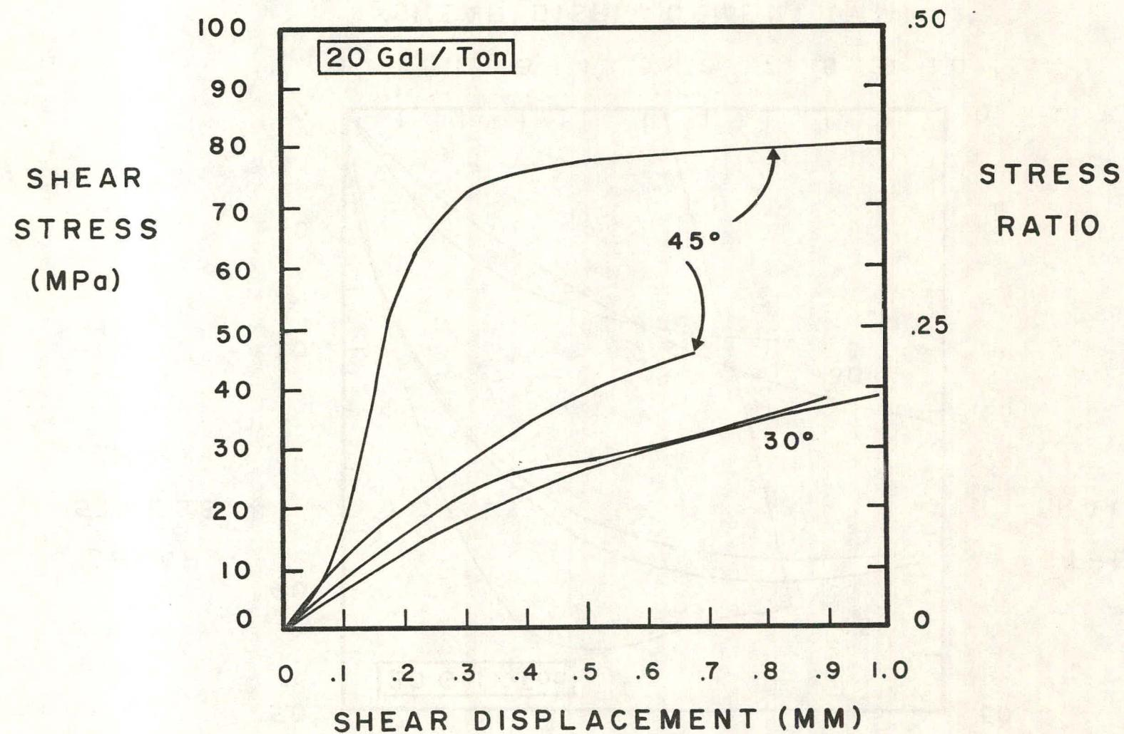
Figure D-3. Shear stress vs. shear displacement results for 20 gal/ton oil shale triaxial shear tests, with 200 MPa normal stress.
