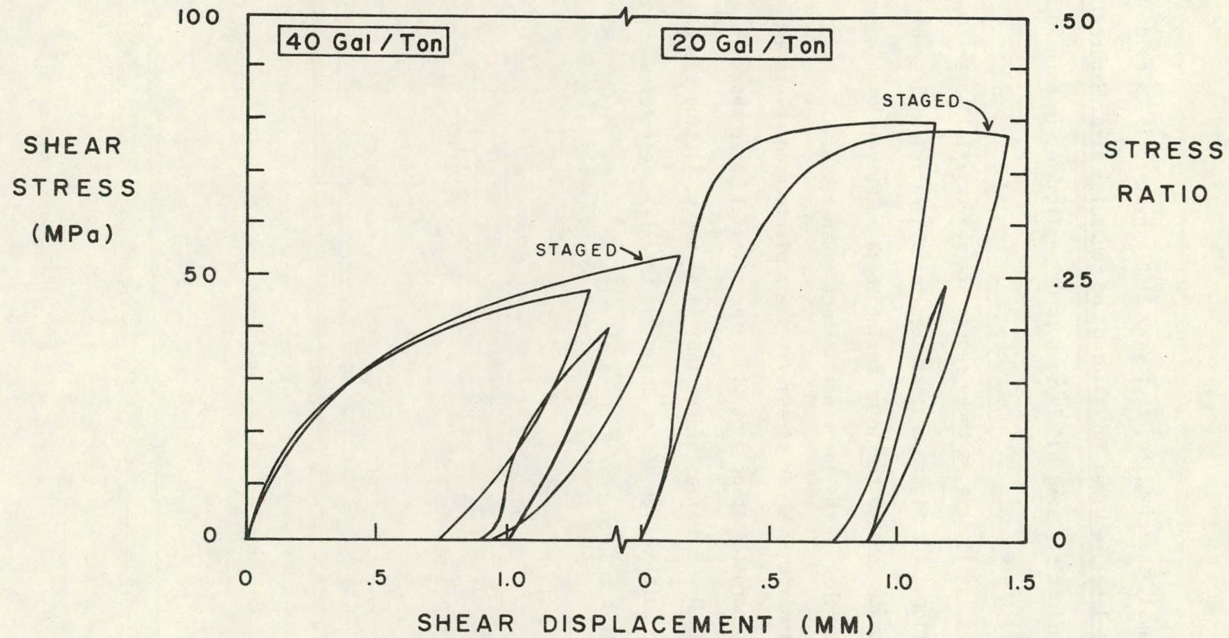
Figure 12. Shear stress vs. shear displacement curves for four  $45^\circ$  joints at 200 MPa normal stress, illustrating the difference in stiffness and strength between 20 gal/ton and 40 gal/ton oil shale and the negligible effect of staging on the joint properties. Note that unloading and reloading below the sliding strength shows relatively little nonlinearity and hysteresis.
