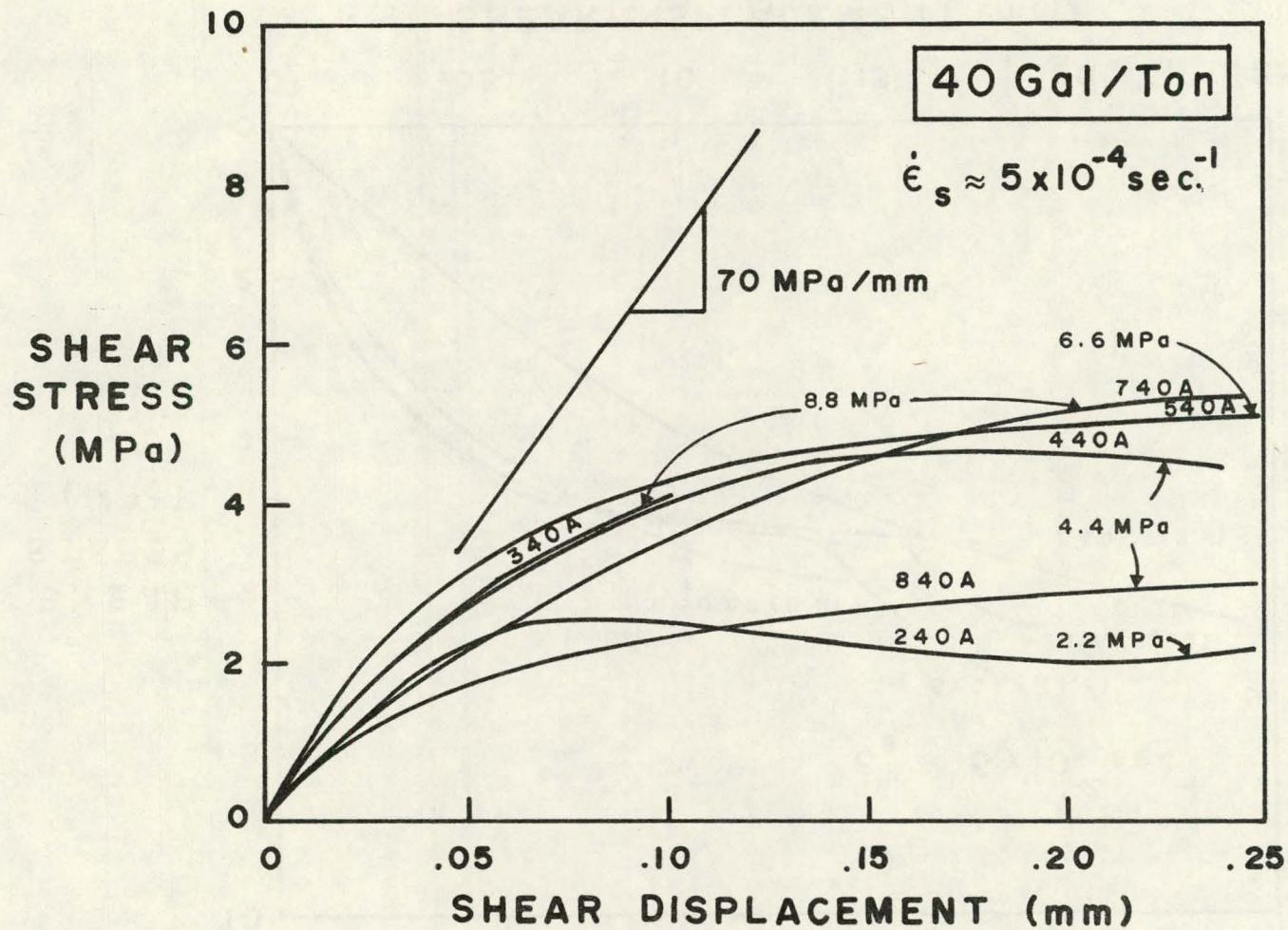
Figure C-4. Shear stress vs. shear displacement results for 40 gal/ton oil shale direct shear tests at an average strain rate of  $5 \times 10^{-4} \text{ sec.}^{-1}$ .
