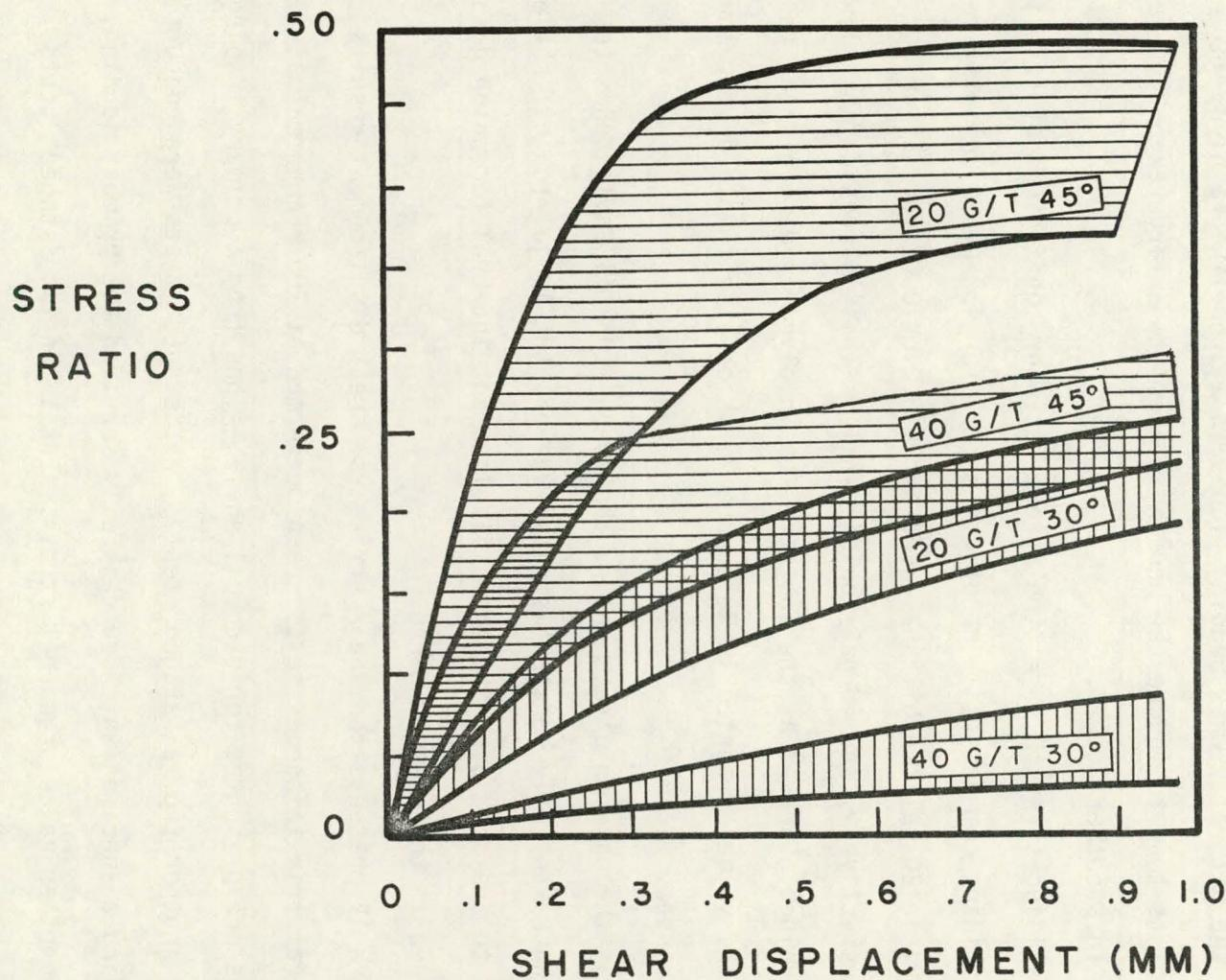
Figure 11. Shear stress/normal stress ratio vs. shear displacement results for all triaxial shear tests. 30° joints are less stiff and weaker than 45° joints in the same grade of oil shale, and 40 gal/ton oil shale is considerably weaker and more compliant than 20 gal/ton oil shale, in this high normal stress regime.
