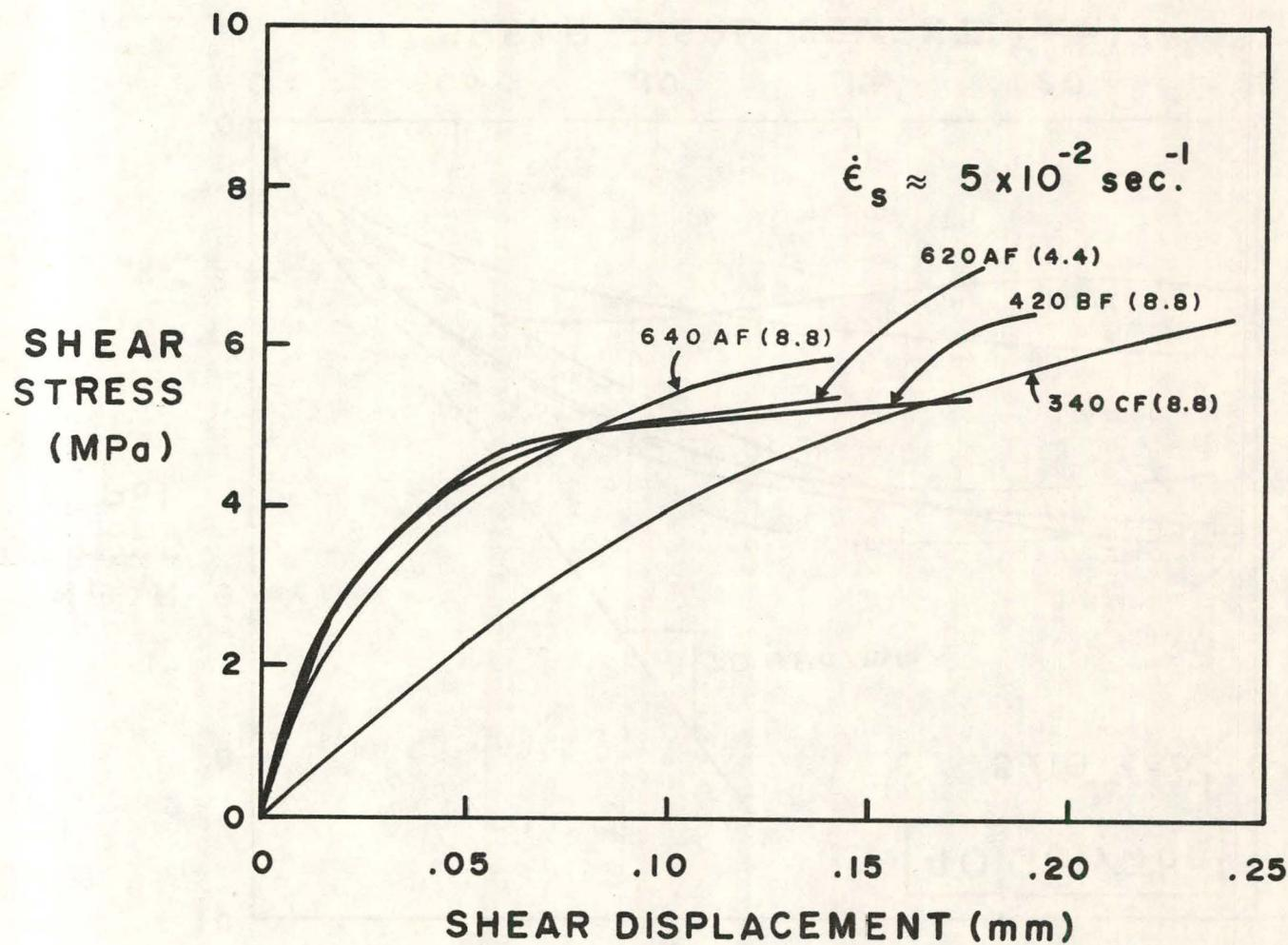
Figure C-5. Shear stress vs. shear displacement results for 20 and 40 gal/ton oil shale direct shear tests at an average strain rate of  $5 \times 10^{-2} \text{ sec}^{-1}$ .
