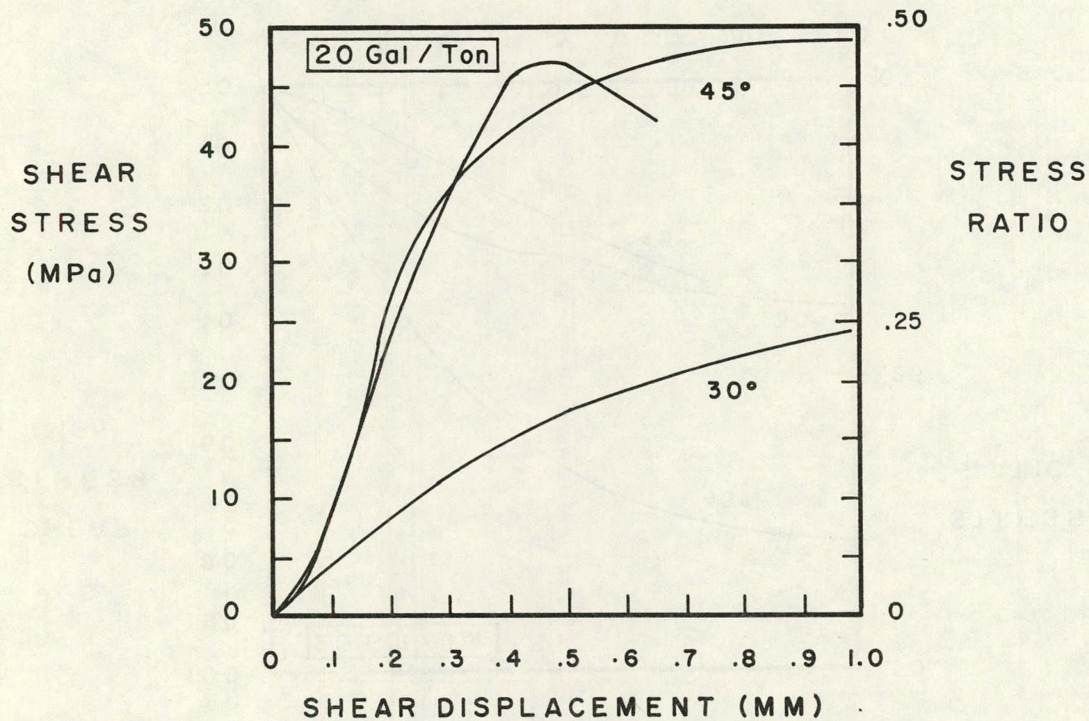
Figure D-4. Shear stress vs. shear displacement results for 20 gal/ton oil shale triaxial shear tests, with 100 MPa normal stress. These are "staged" tests, on specimens previously tested at 200 MPa normal stress.
