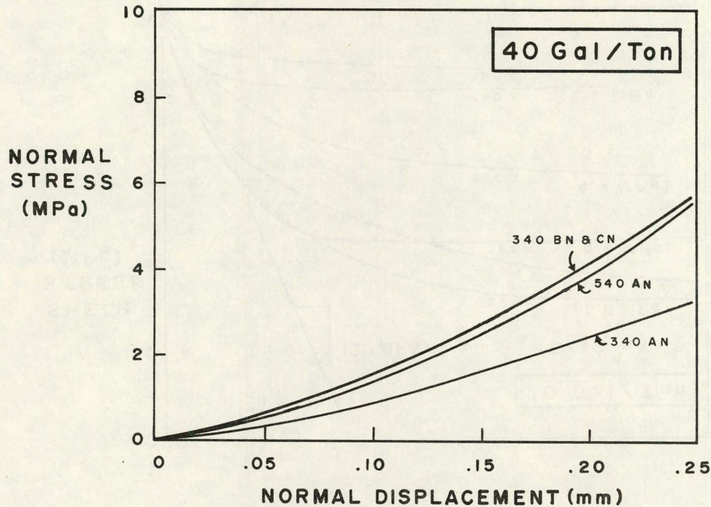
Figure C-2. Normal stiffness results for 40 gal/ton oil shale direct shear specimens.
