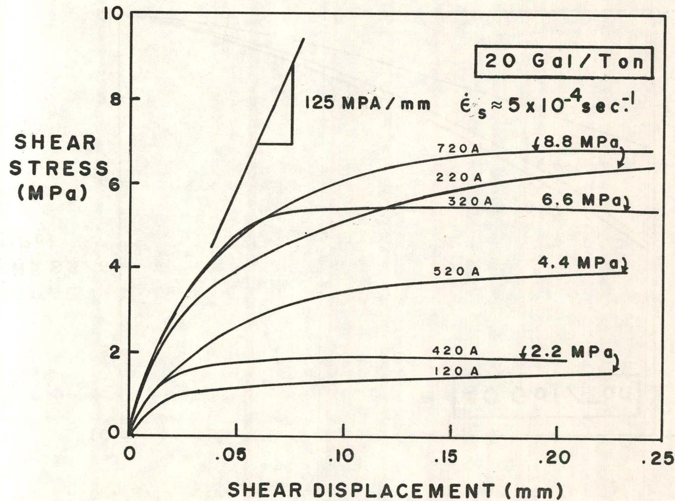
Figure C-3. Shear stress vs. shear displacement results for 20 gal/ton oil shale direct shear tests at an average strain rate of  $5 \times 10^{-4} \text{ sec}^{-1}$ .
