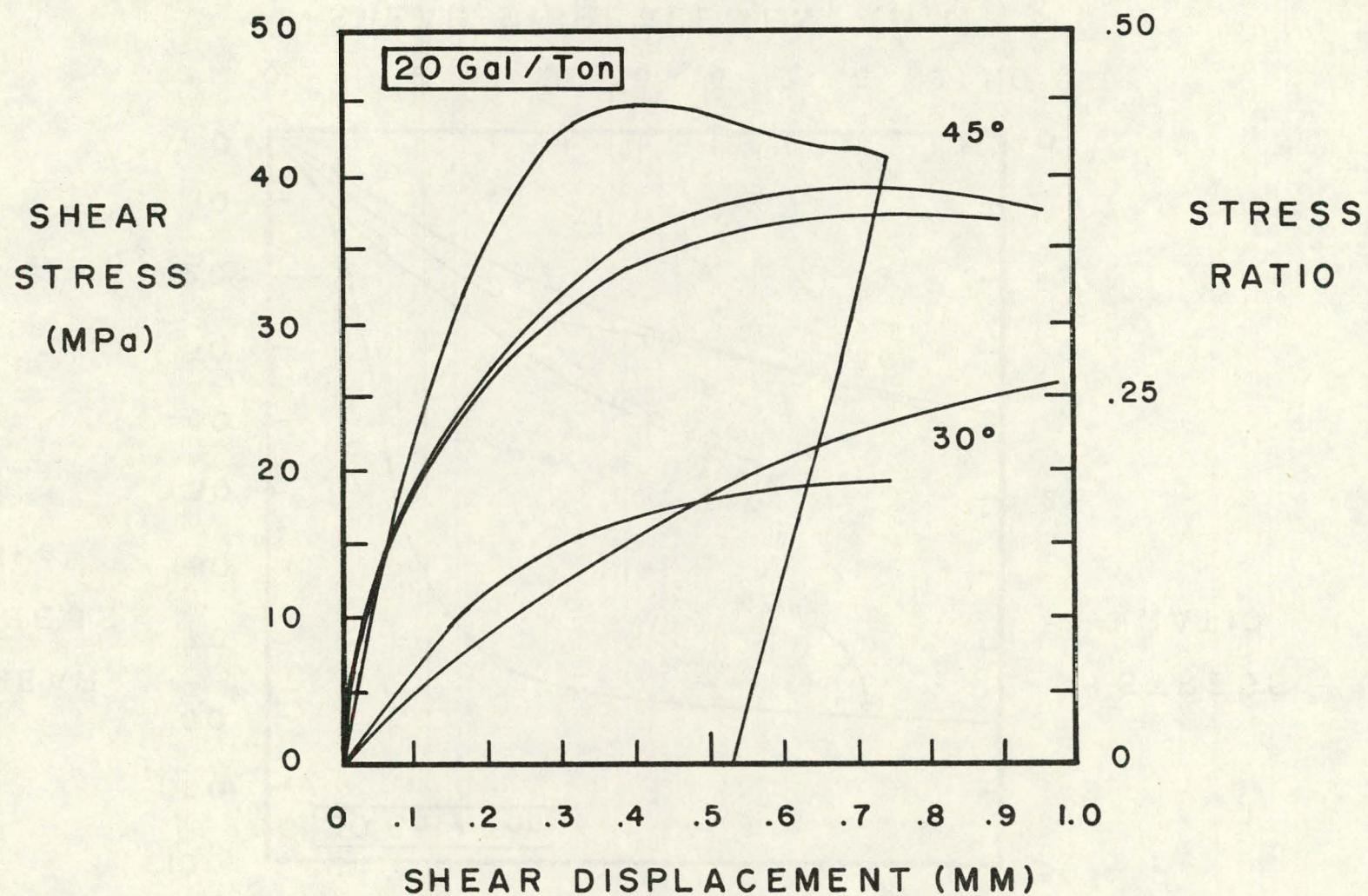
Figure D-2. Shear stress vs. shear displacement results for 20 gal/ton oil shale triaxial shear tests, with 100 MPa normal stress.
