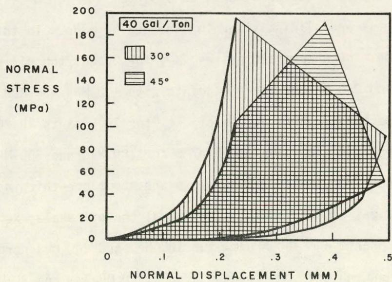
Figure 10. Normal stiffness results for 40 gal/ton oil shale triaxial shear specimens. Note that the scale is different from Figure 9.
