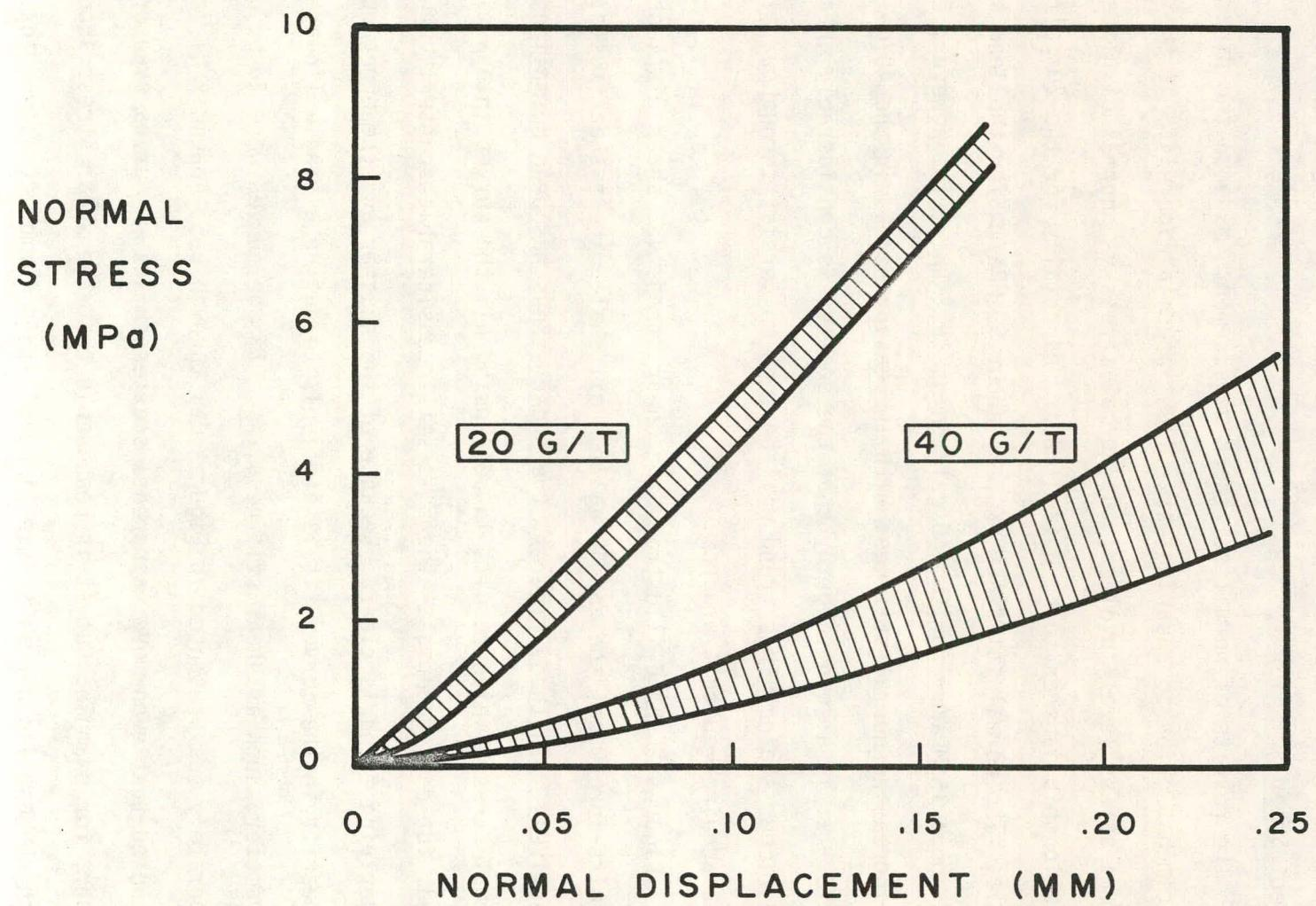
Figure 4. Normal stiffness results for direct shear specimens.
