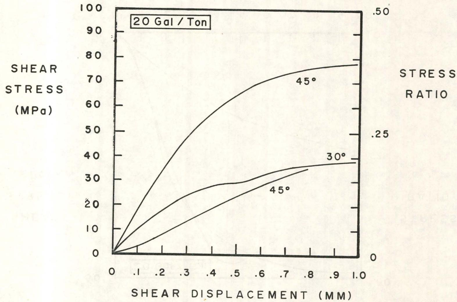
Figure D-5. Shear stress vs. shear displacement results for 20 gal/ton oil shale triaxial shear tests, with 200 MPa normal stress. These are "staged" tests, on specimens previously tested at 100 MPa normal stress.
