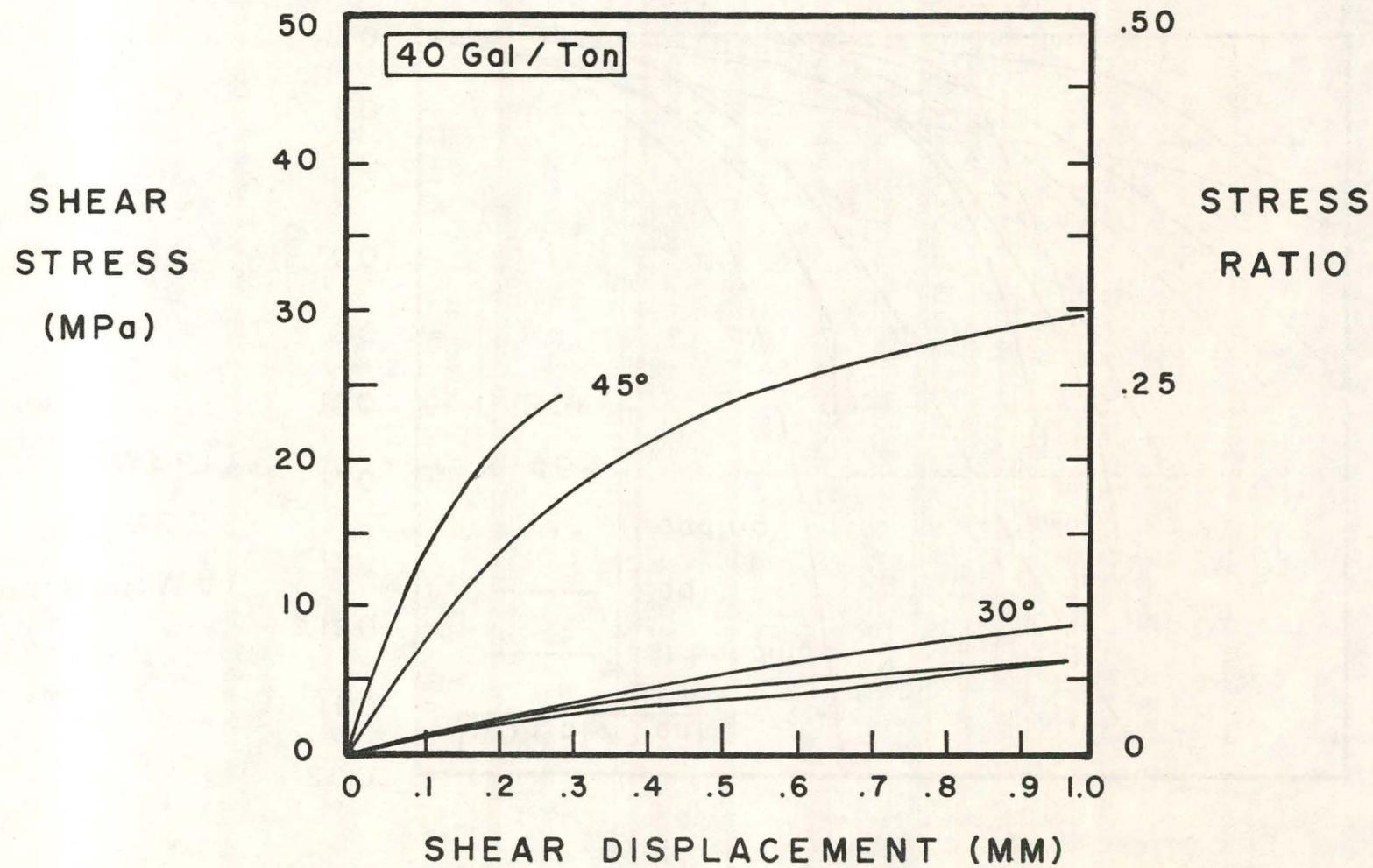
Figure D-7. Shear stress vs. shear displacement results for 40 gal/ton oil shale triaxial shear tests, with 100 MPa normal stress.
