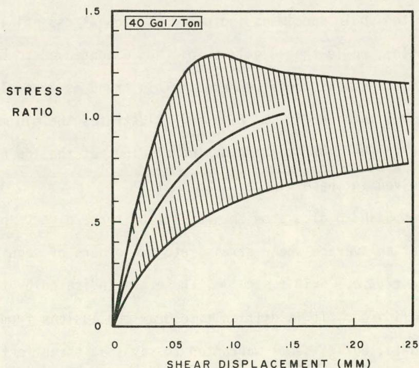
Figure 6. Direct shear results for 40 gal/ton oil shale. Stress ratio is the ratio of shear stress to normal stress. The shaded band is the envelope of all "slow" tests, while the solid curve is the result of the "fast" test.
