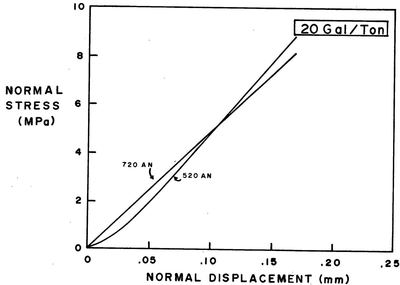
Figure C-1. Normal stiffness results for 20 gal/ton oil shale direct shear specimens.
