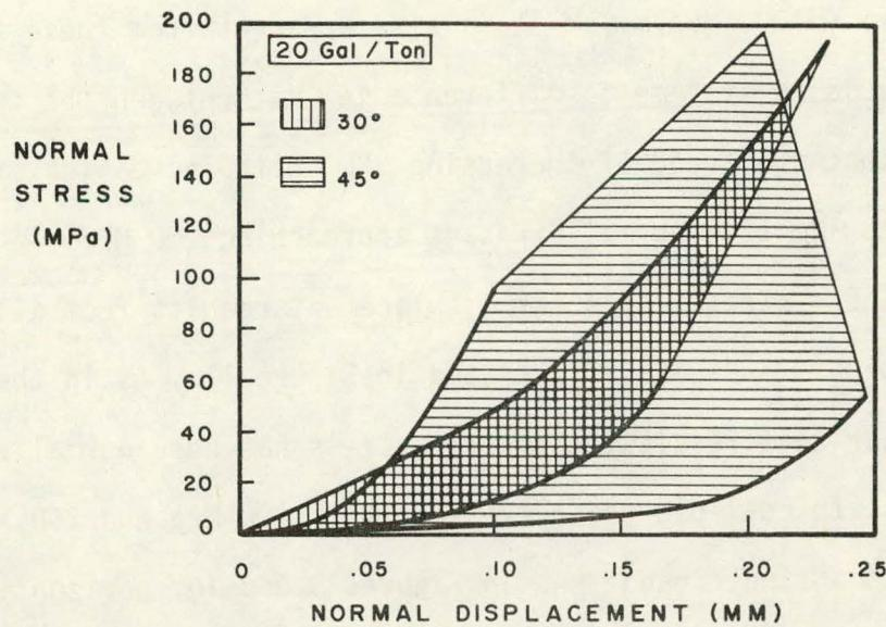
Figure 9. Normal stiffness results for 20 gal/ton oil shale triaxial shear specimens. The wider scatter band for 45° joints is simply a consequence of a larger number of tests than for the 30° joints.
