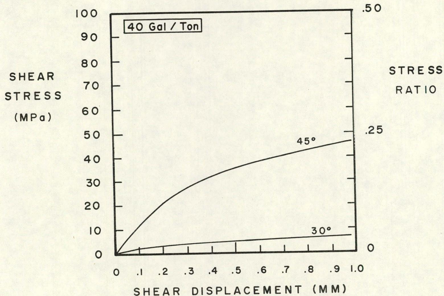
Figure D-10. Shear stress vs. shear displacement results for 40 gal/ton oil shale triaxial shear tests, with 200 MPa normal stress. These are "staged" tests, on specimens previously tested at 100 MPa normal stress.
