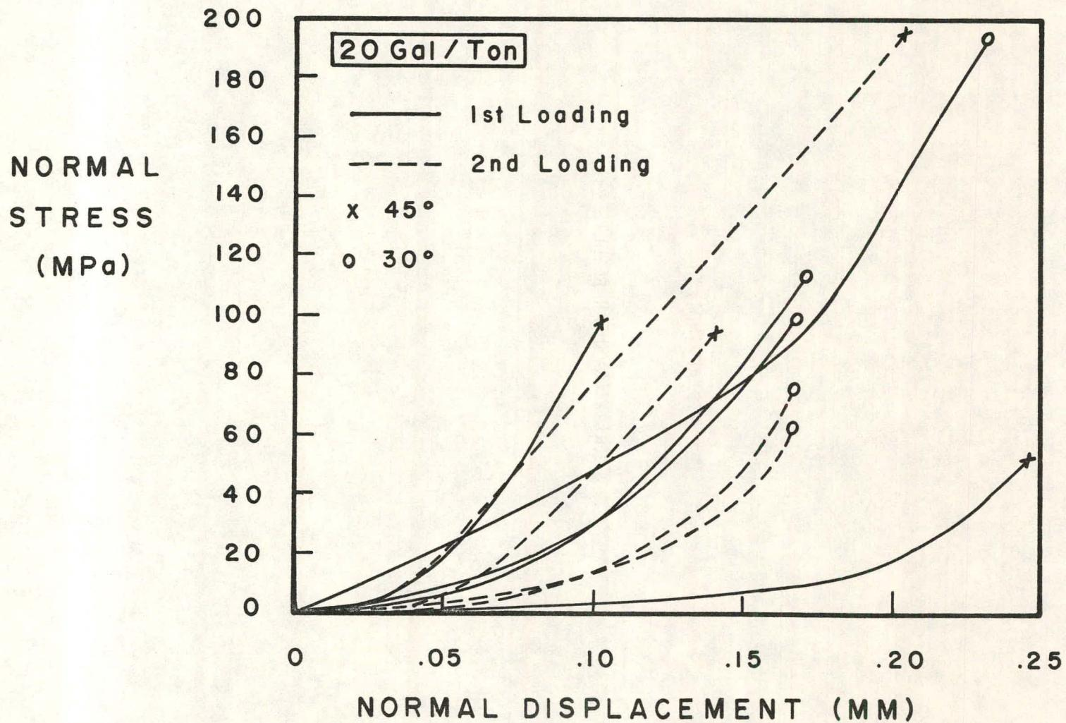
Figure D-1. Normal stiffness results for 20 gal/ton oil shale triaxial shear specimens.
