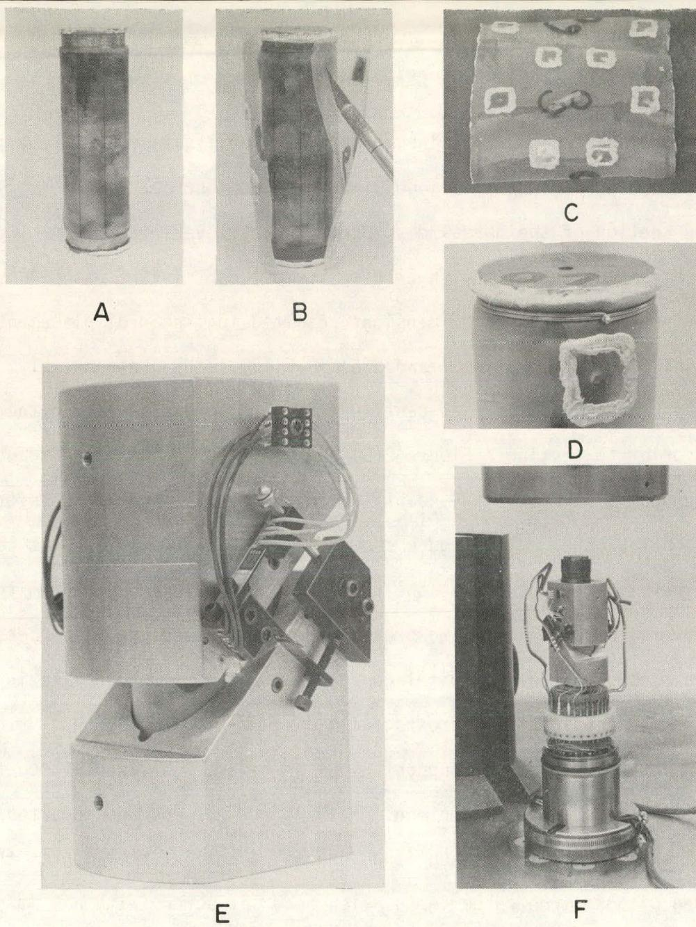
Figure 3. Sequence of preparation of triaxial shear specimens.
