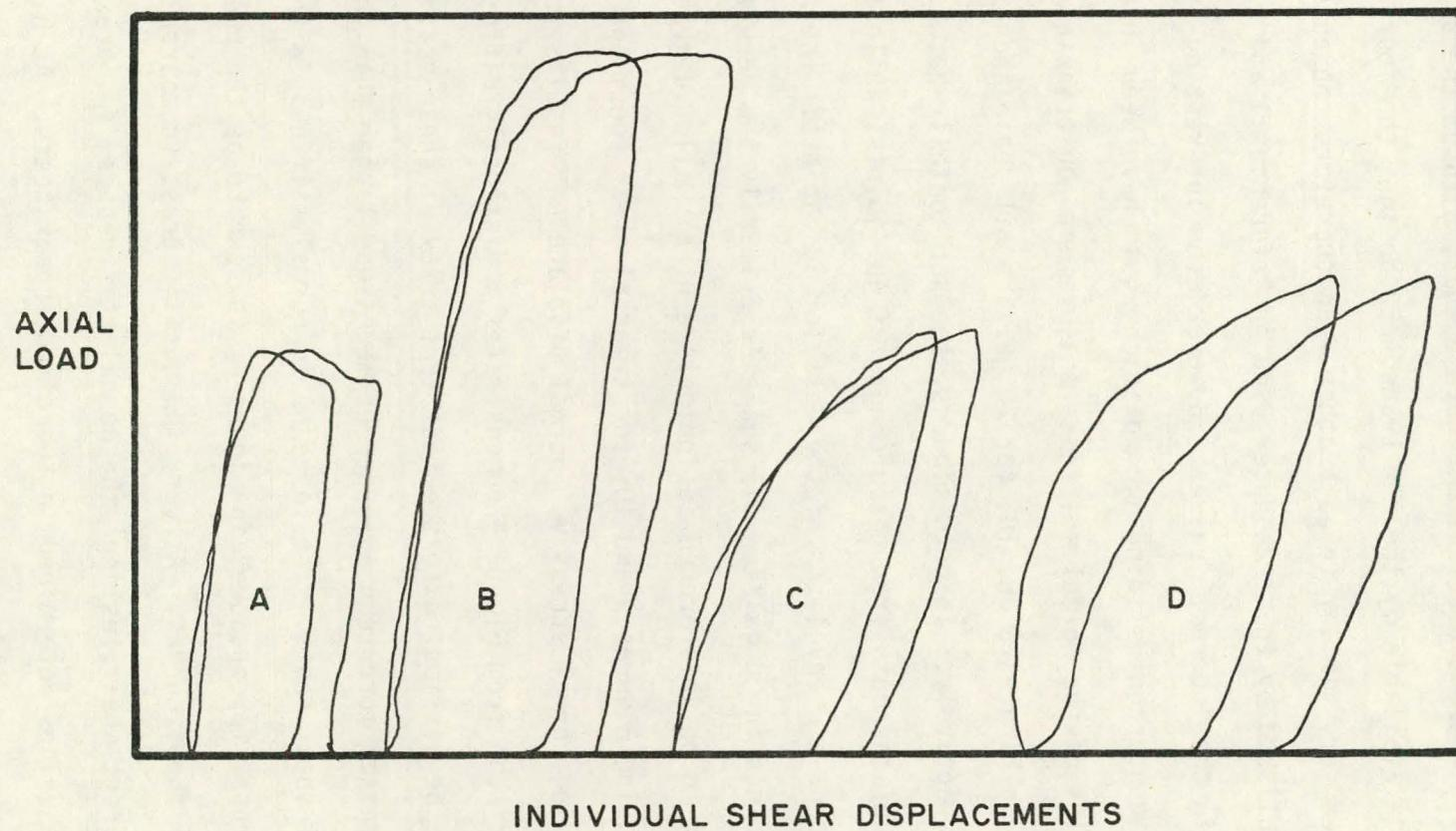
Figure 8. Representative raw data illustrating the axial load vs. shear displacement results. The two curves are those obtained from opposite sides of the specimen. A, B and C are typical of most of the results, while D is an example of some of the worst disagreement between the two individual shears.
