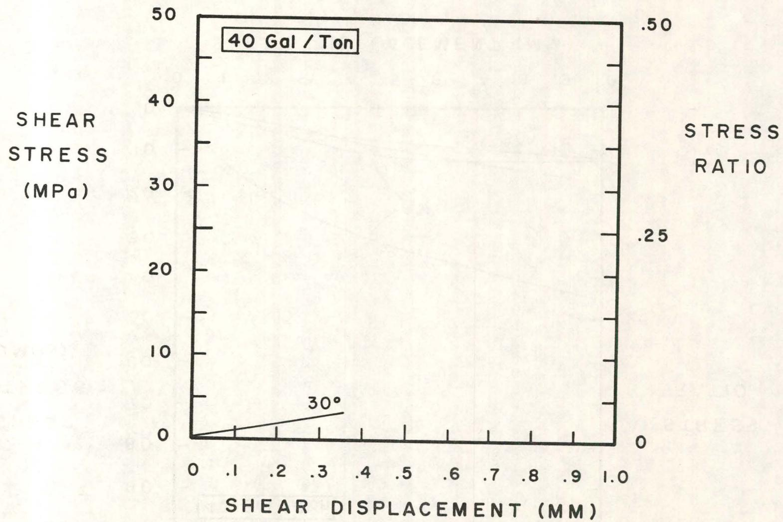
Figure D-9. Shear stress vs. shear displacement results for 40 gal/ton oil shale triaxial shear tests, with 100 MPa normal stress. These are "staged" tests, on specimens previously tested at 200 MPa normal stress.
