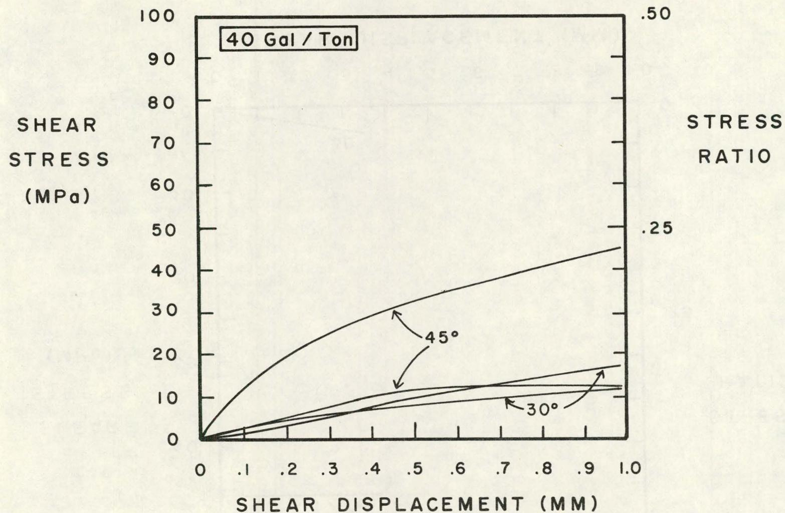
Figure D-8. Shear stress vs. shear displacement results for 40 gal/ton oil shale triaxial shear tests, with 200 MPa normal stress.
