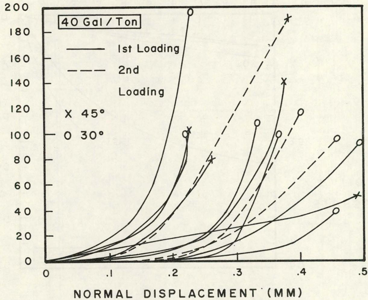
Figure D-6. Normal stiffness results for 40 gal/ton oil shale triaxial shear specimens.
