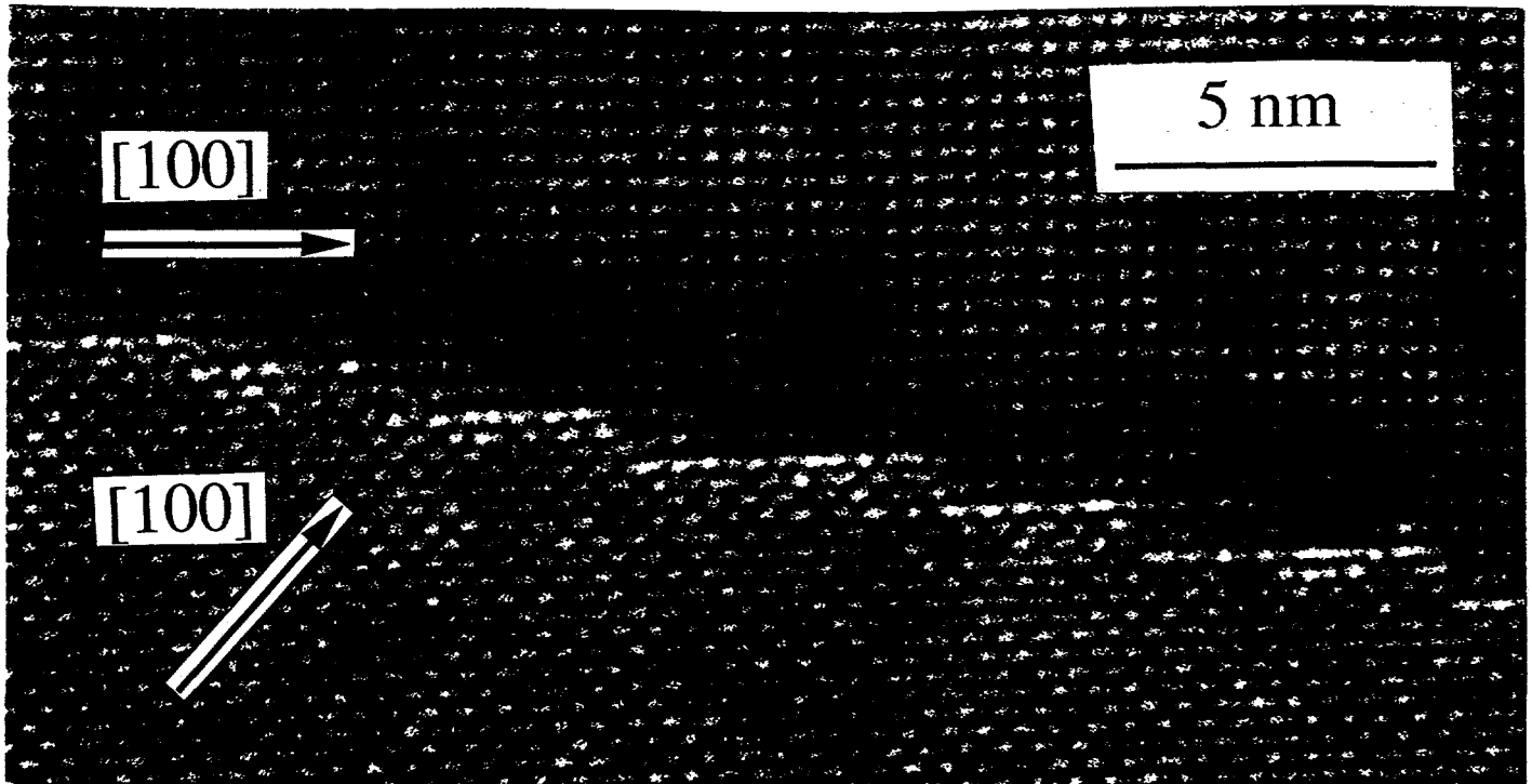
Figure 5. High resolution electron micrograph of a \text{YBa}_2\text{Cu}_3\text{O}_{7-x} 45^\circ [001] tilt grain boundary junction showing a series of asymmetric microfacets.
