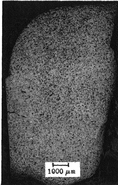
FIGURE 6. Longitudinal Section of GPHS Pellet 7. Heat treated, polished.
