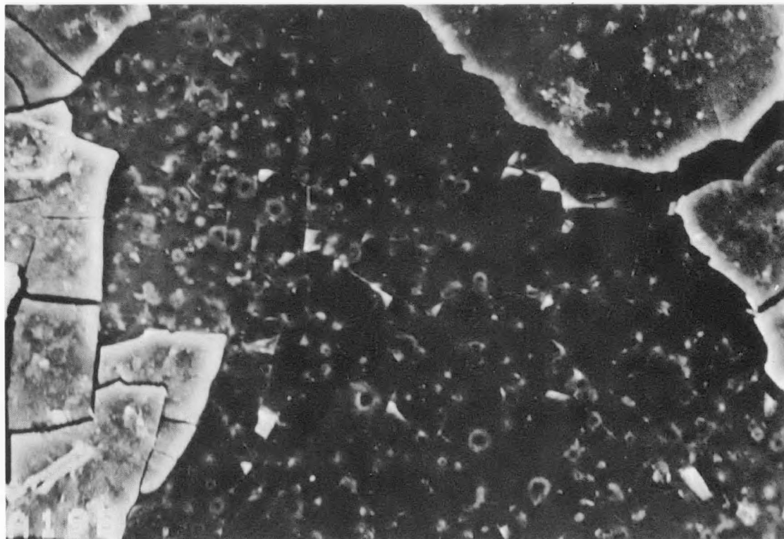
FIGURE 30 SEM VISUALIZATION OF FILM SLOUGHING ON ALUMINUM SURFACE (MAG. 270X)
