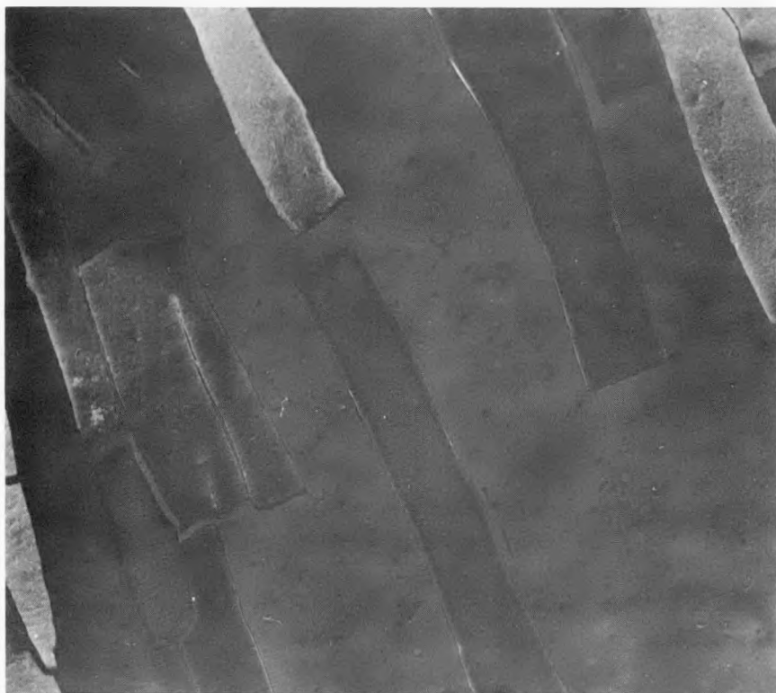
FIGURE 37 SEM VISUALIZATION OF THE CLEANED ALUMINUM SURFACES (MAG. 430X)
