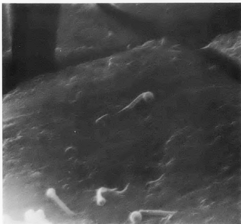
FIGURE 39 SEM VISUALIZATION OF THE CLEANED ALUMINUM SURFACE (MAG. 5000X)
