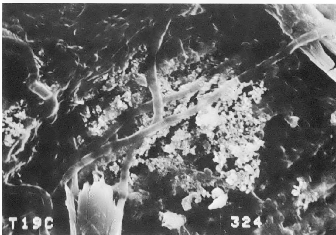
FIGURE 29 SEM VISUALIZATION OF FILM BULK GROWTH ON TITANIUM SURFACE (MAG. 1800X)
