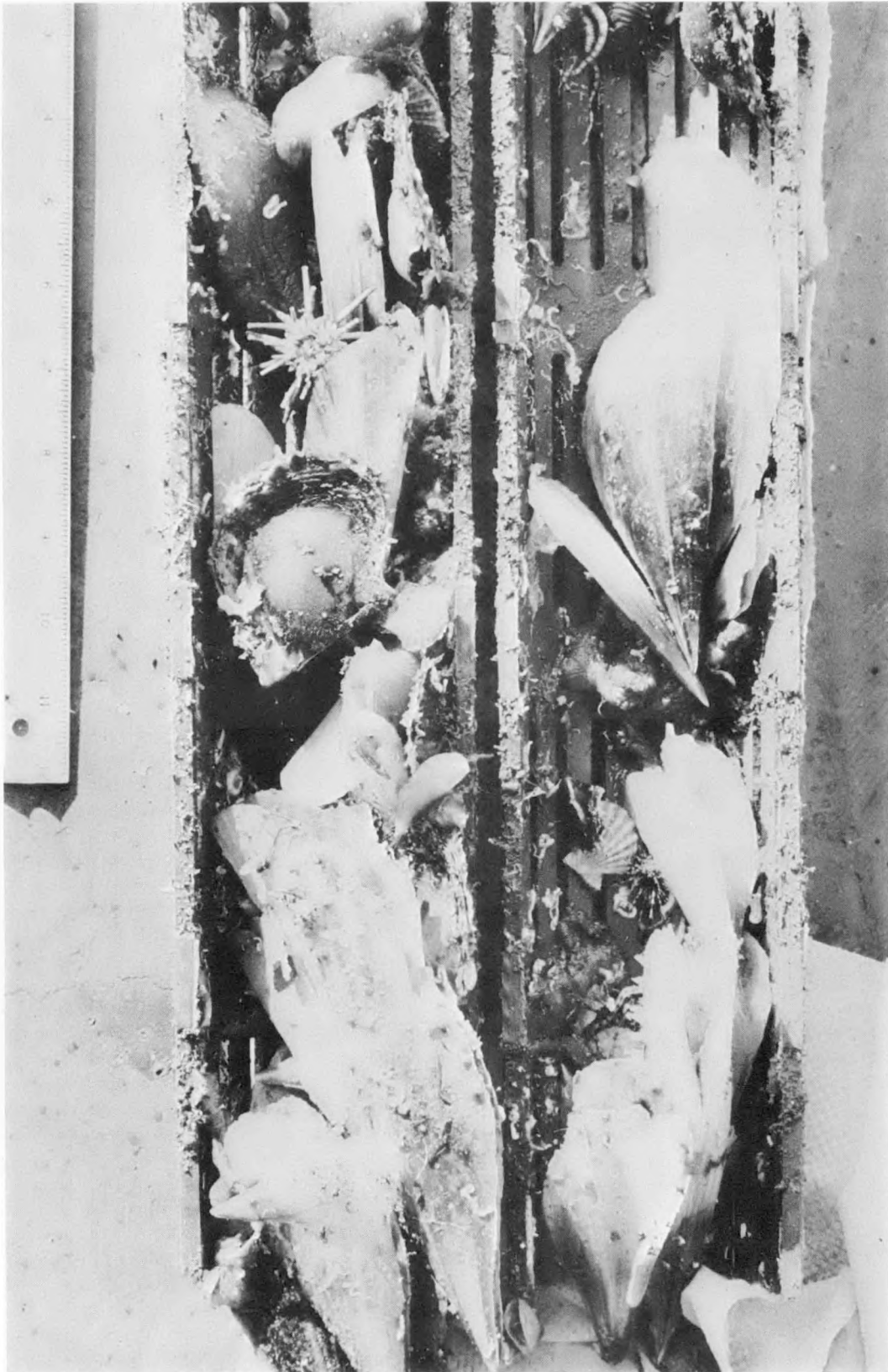
FIGURE 44 PHOTOGRAPH OF AN INTAKE STRAINER SPLIT LENGTHWISE TO EXPOSE THE ORGANISMS LIVING INSIDE
