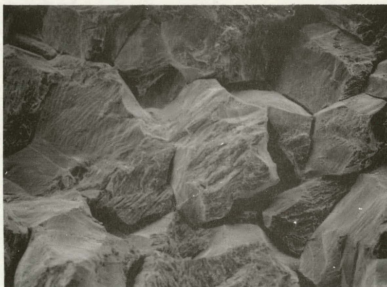
FIGURE 8. Fracture of Notch Tensile Specimen of Sensitized Type 304L Stainless Steel in High-Pressure Hydrogen
