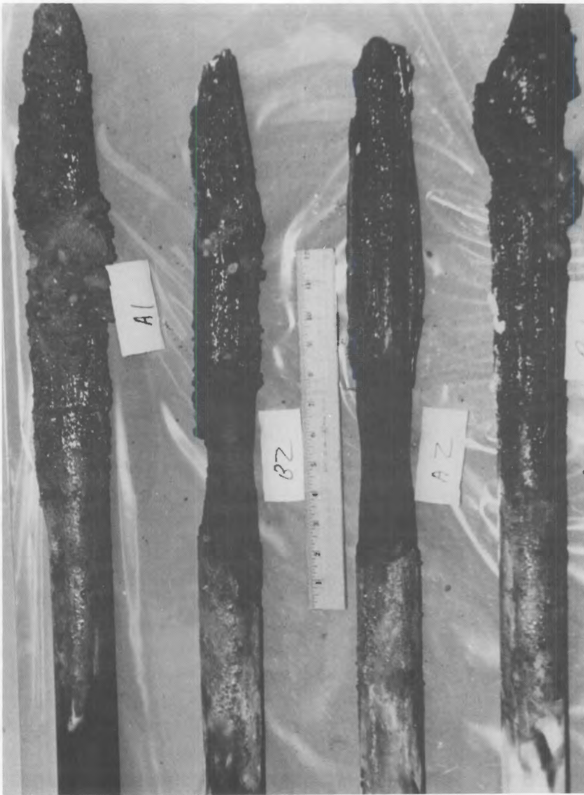
FIGURE 5.6. Posttest Observation of Electrode Corrosion from ES-INEL-4
