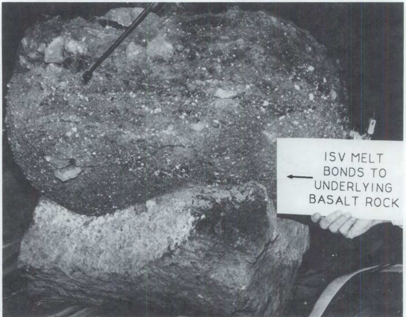
FIGURE 5.3. Vitrified Block Resulting from ES-INEL-4
