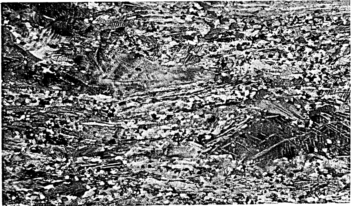
Figure 22. ALLOY N, URANIUM- (IMPURE) 600 PPM SILICON-300 PPM IRON, ANNEALED FOR SEVEN HOURS AT 550°C. (Partial recrystallization.) (Polarized light; 100X)
