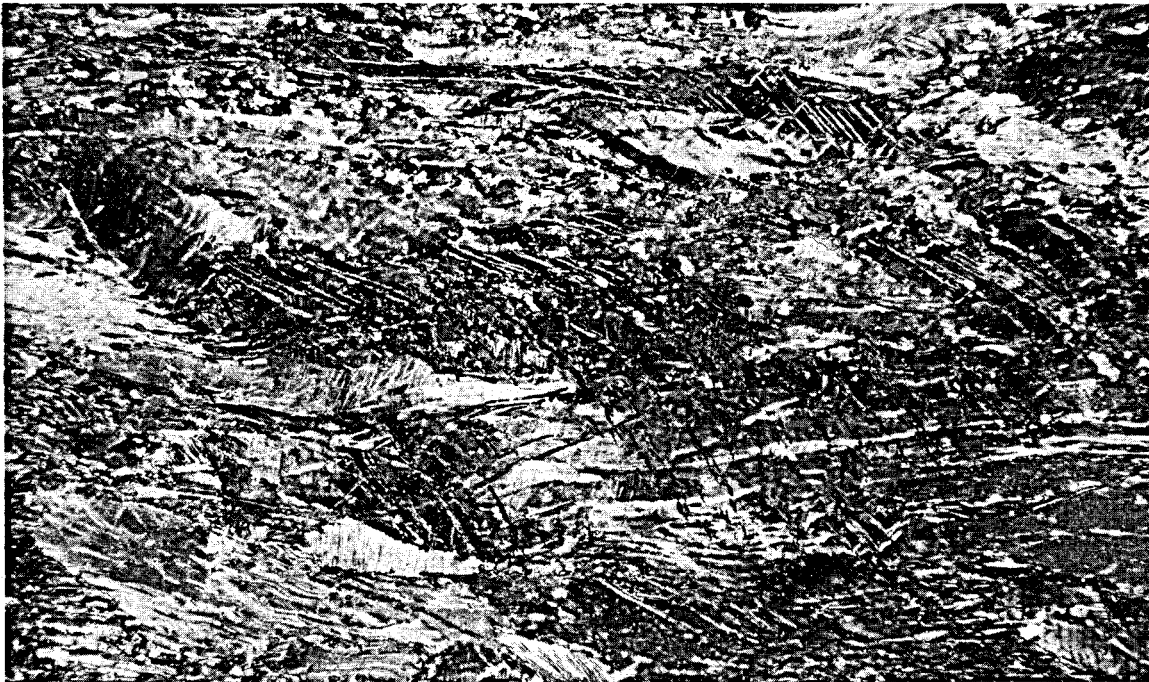
Figure 20. ALLOY 2K, URANIUM- (IMPURE) 800 PPM SILICON-400 PPM IRON, ANNEALED FOR SEVEN HOURS AT 550°C. (Incipient recrystallization.) (Polarized light; 100X)
