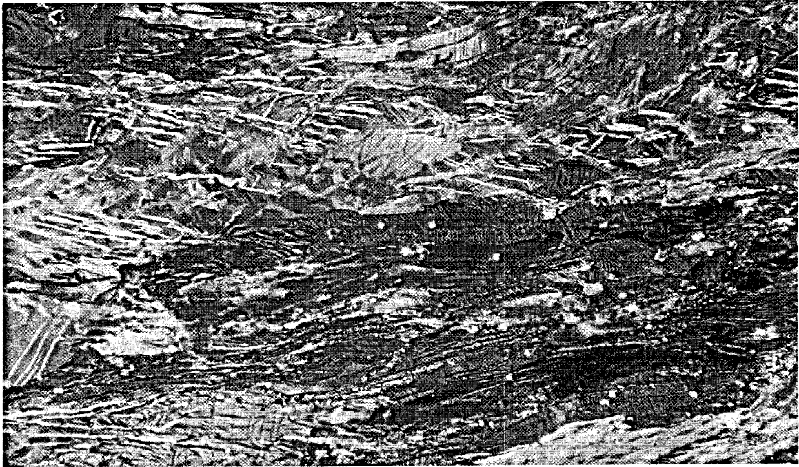
Figure 21. ALLOY N, URANIUM- (IMPURE) 600 PPM SILICON-300 PPM IRON, ANNEALED FOR FOUR HOURS AT 550°C. (Incipient recrystallization.) (Polarized light; 100X)
