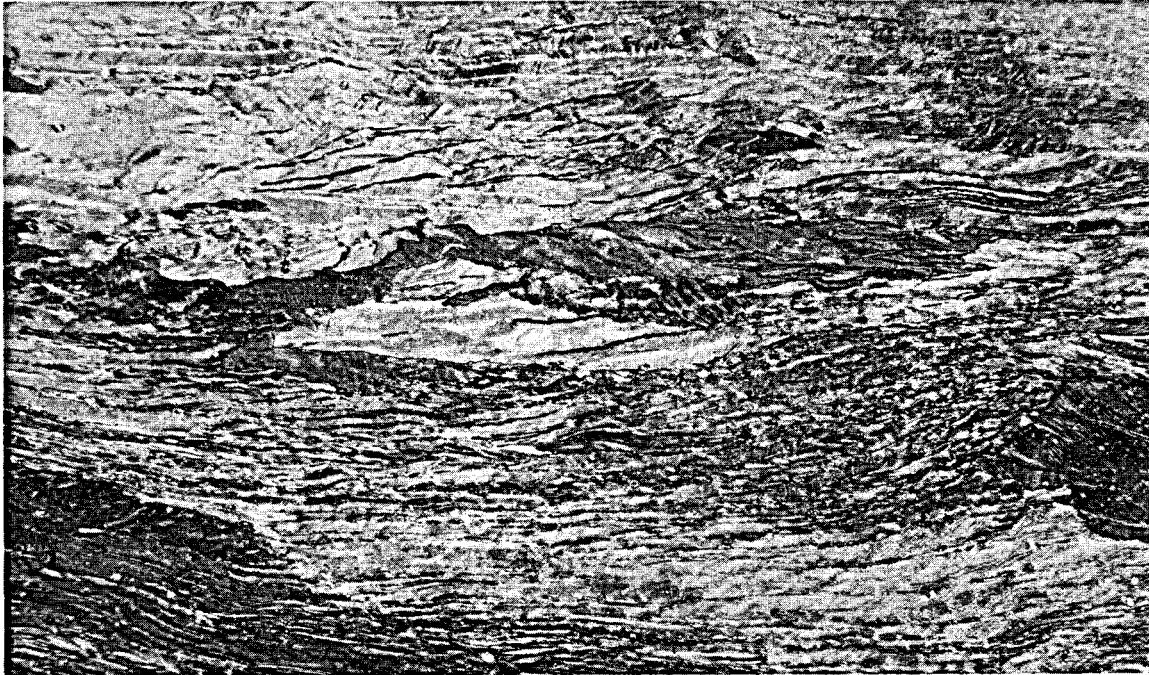
Figure 19. ALLOY 2K, URANIUM- (IMPURE) 800 PPM SILICON-400 PPM IRON, ANNEALED FOR FOUR HOURS AT 550°C. (Incipient recrystallization.) (Polarized light; 100X)
