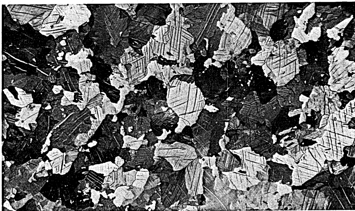
Figure 8. ALLOY L, URANIUM-600 PPM IRON, VACUUM SOLUTION HEAT-TREATED FOR FOUR HOURS AT 800° C AND WATER-QUENCHED. (Polarized light; 100X)
