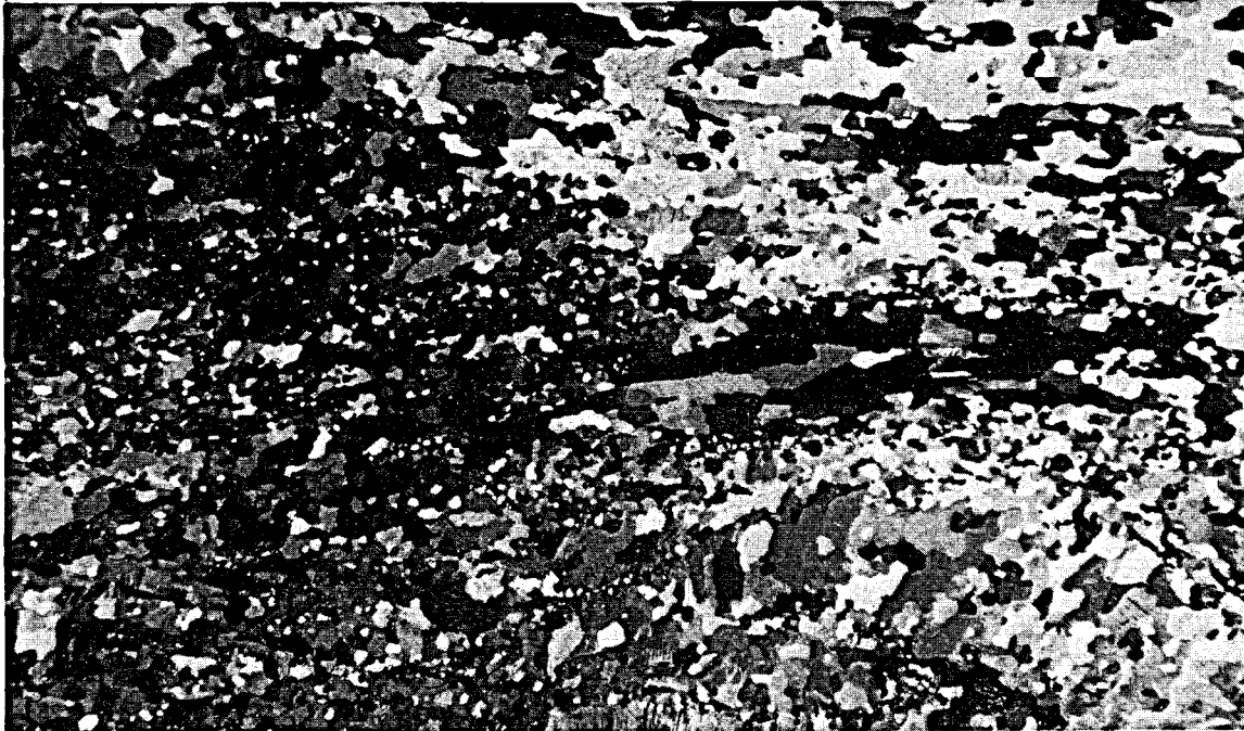
Figure 23. ALLOY L, URANIUM-600 PPM IRON, ANNEALED FOR FOUR HOURS AT 550°C. (Completely recrystallized.) (Polarized light; 100X)
