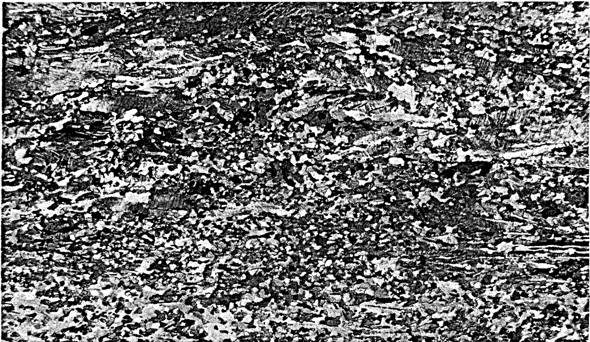
MS-80-0724-11 Figure 18. ALLOY I, URANIUM-400 PPM SILICON-200 PPM ALUMINUM, ANNEALED FOR ONE HOUR AT 550°C. (Incompletely recrystallized.) (Polarized light; 100X)
