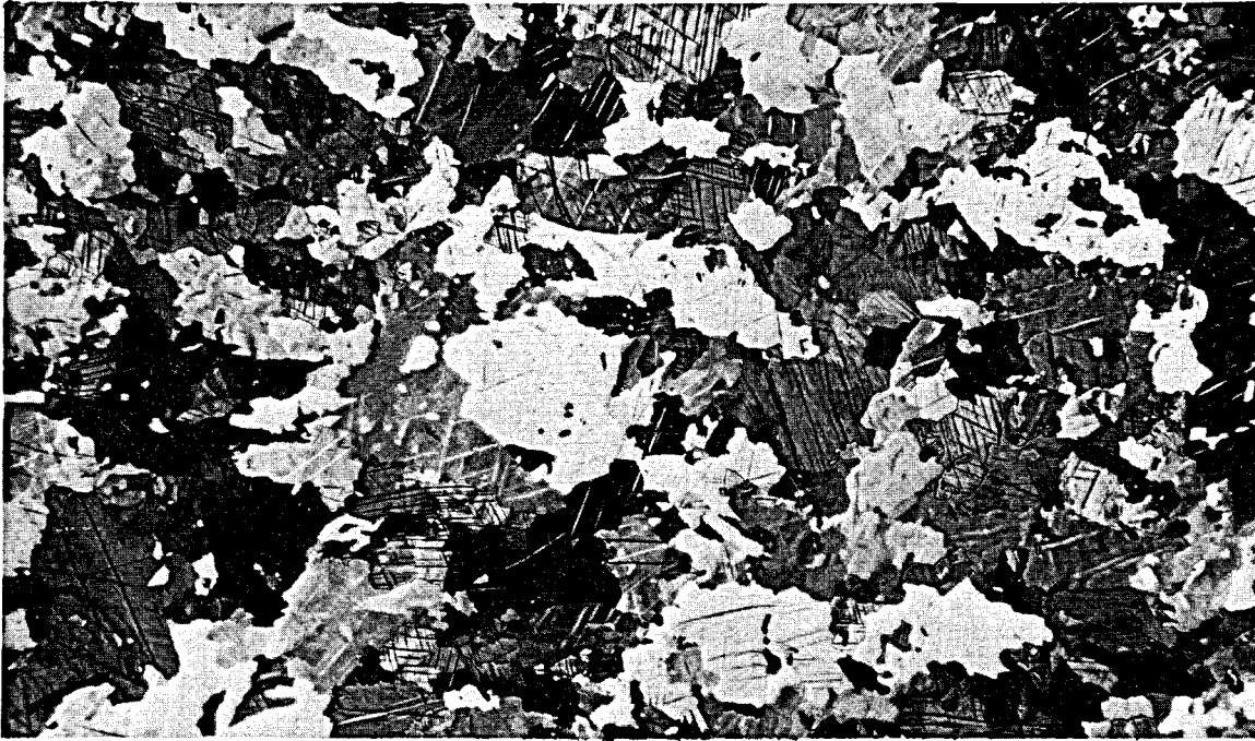
Figure 5. ALLOY F, URANIUM-300 PPM IRON, VACUUM SOLUTION HEAT-TREATED FOR FOUR HOURS AT 800°C AND WATER-QUENCHED. (Polarized light; 100X)
