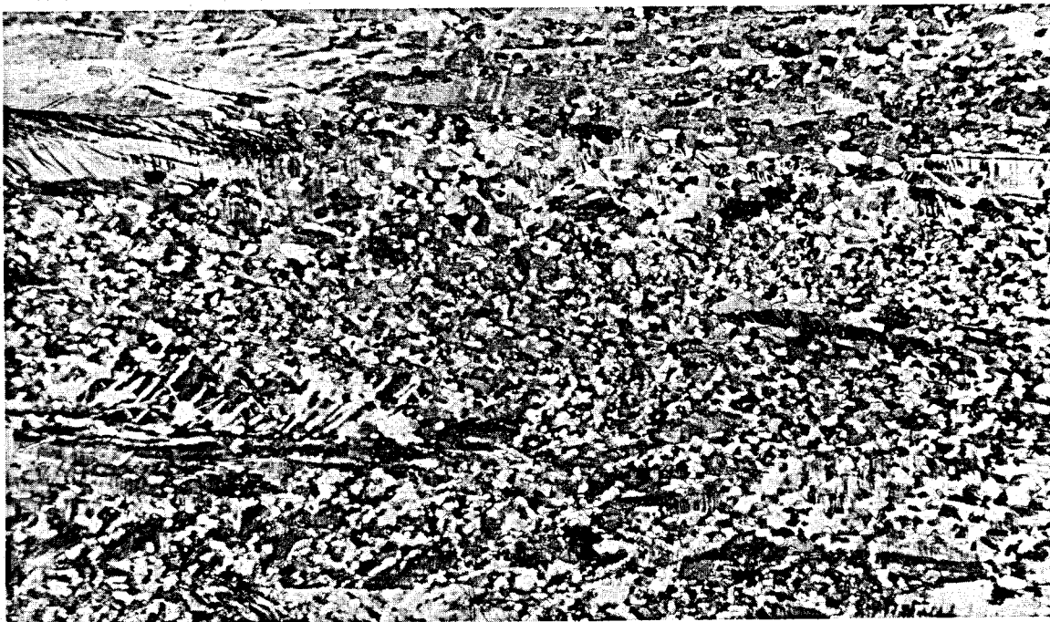
Figure 13. ALLOY D, URANIUM-400 PPM SILICON-200 IRON, ANNEALED FOR ONE HOUR AT 550°C. (Incompletely recrystallized.) (Polarized light; 100X)
