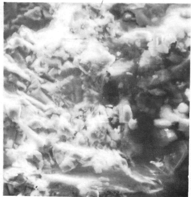
Figure 58. SEM Secondary Electron Images of Fuel Fragments on Cladding I.D. Surface of Standard Blanket Rod 1606710
