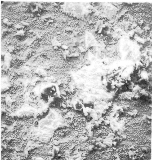
Figure 58. SEM Secondary Electron Images of Fuel Fragments on Cladding I.D. Surface of Standard Blanket Rod 1606710
