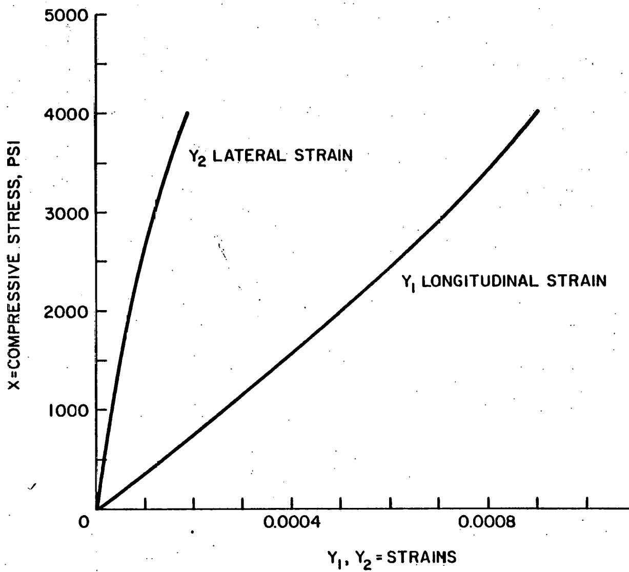
FIG. 2 - STRESS-STRAIN CURVES USING X-Y-Y PLOTTER FOR STATIC TEST
