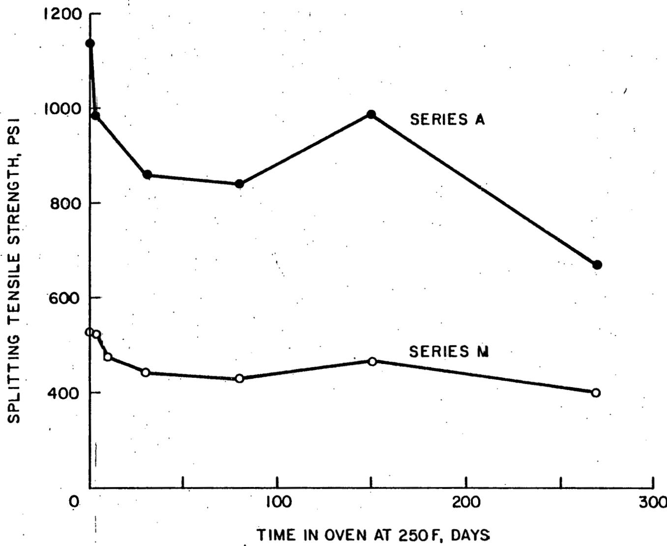
FIG. 13—SPLITTING TENSILE STRENGTH OF TANK FARM AND SERIES M CONCRETE EXPOSED TO ELEVATED TEMPERATURE
