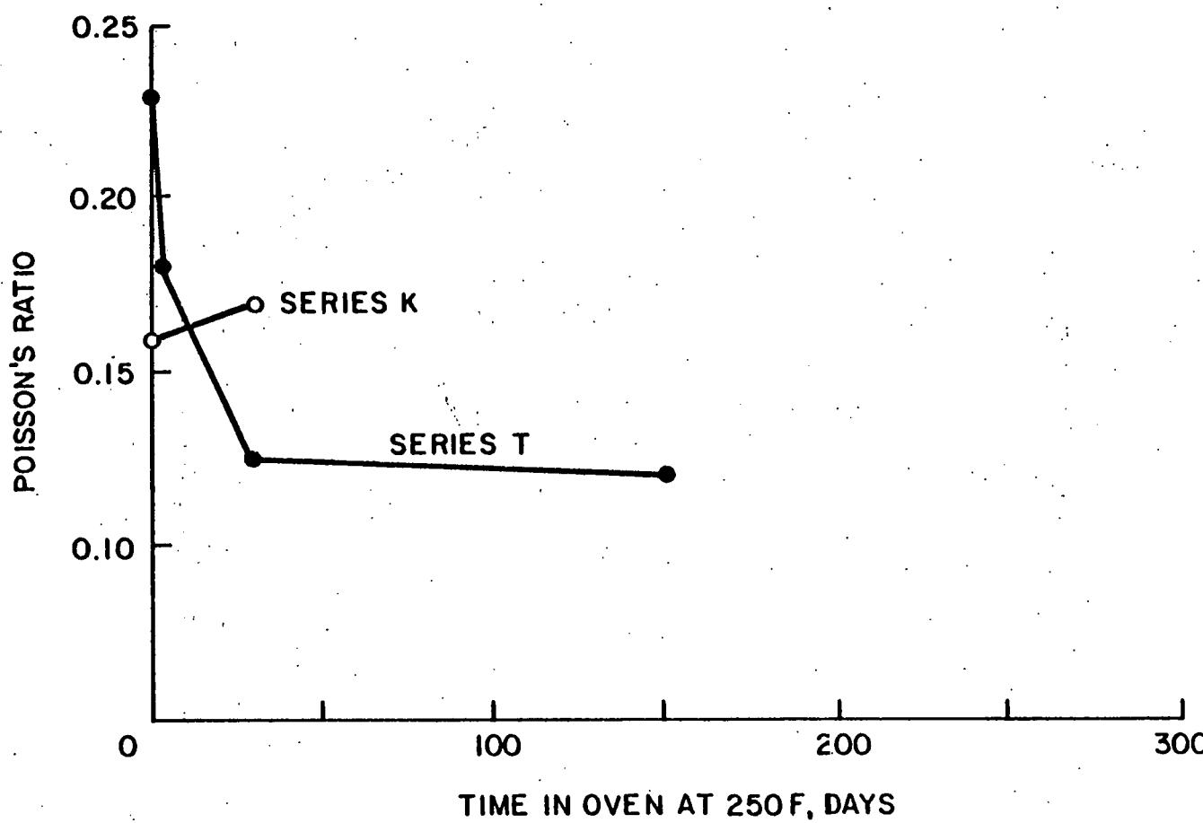
FIG. 6-POISSON'S RATIO OF 3-IN. CUBES EXPOSED TO ELEVATED TEMPERATURE
