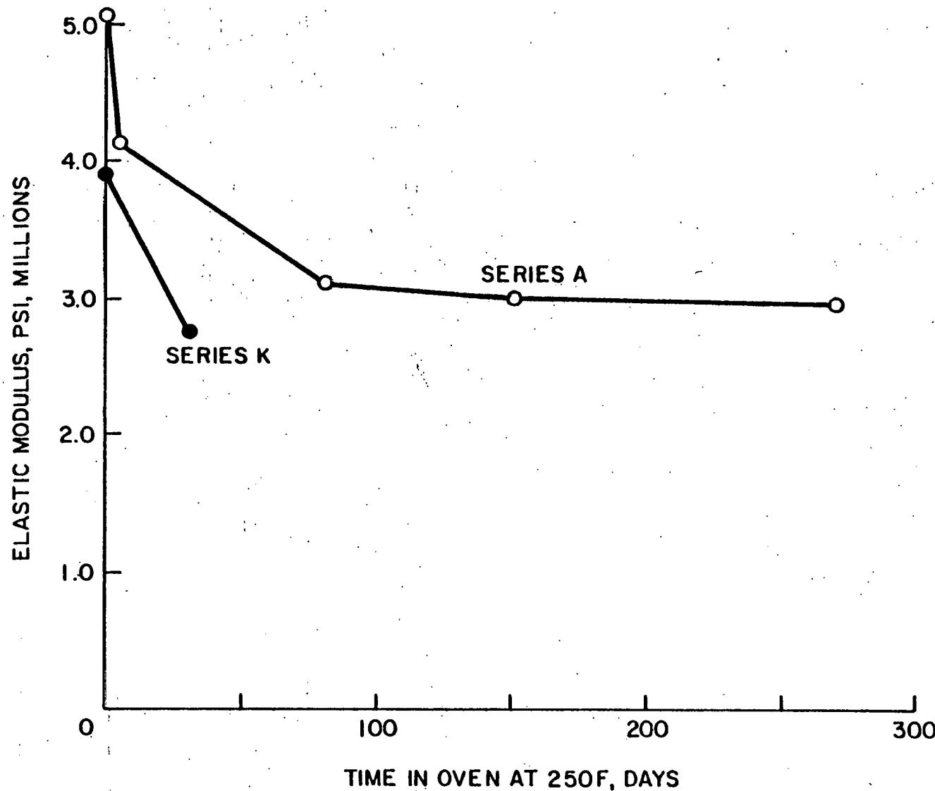
FIG. 3-ELASTIC MODULUS OF 3x6-IN. CYLINDERS EXPOSED TO ELEVATED TEMPERATURE
