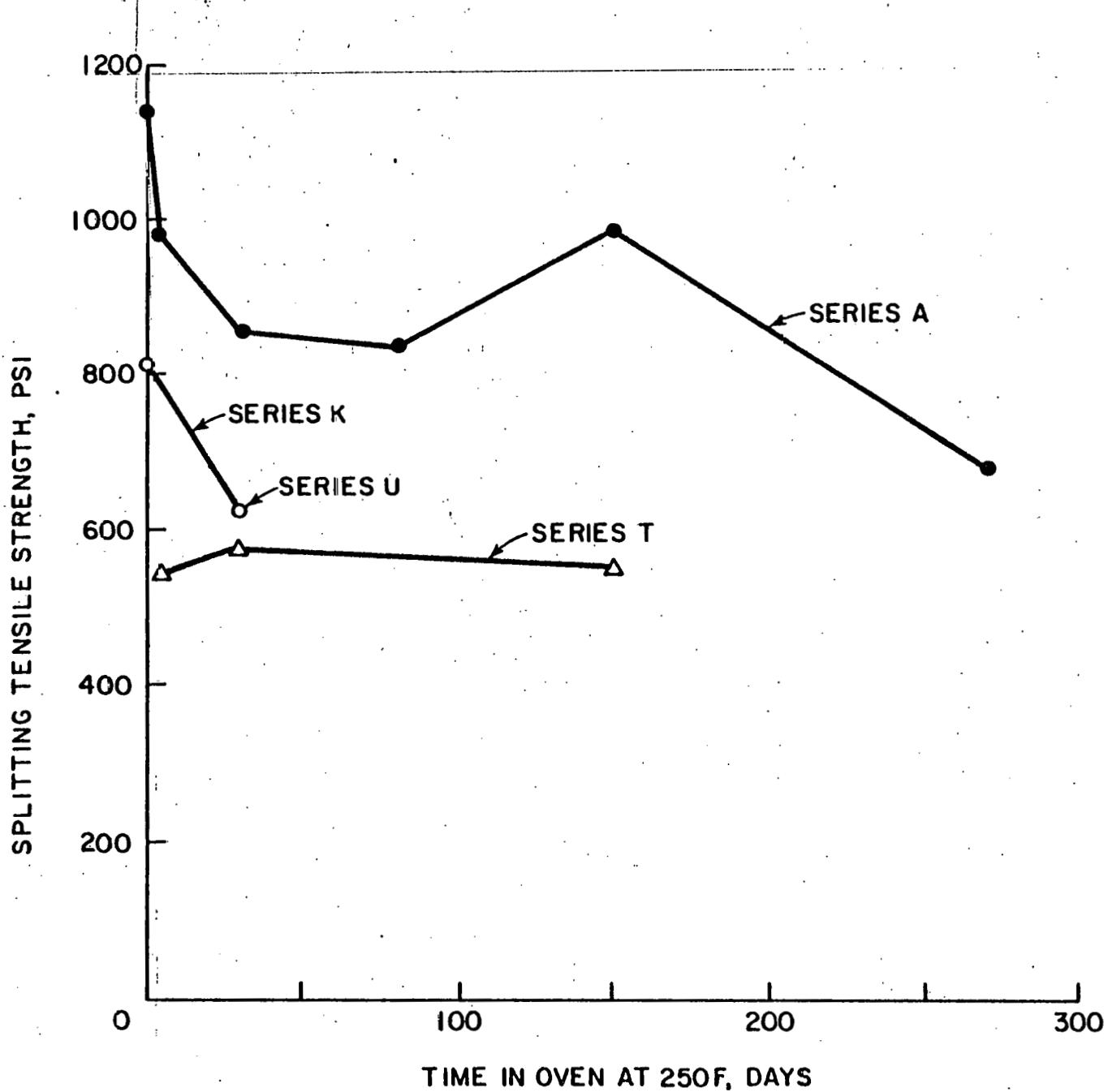
FIG. 9 - SPLITTING TENSILE STRENGTH OF 3x6 IN. CYLINDERS EXPOSED TO ELEVATED TEMPERATURE
