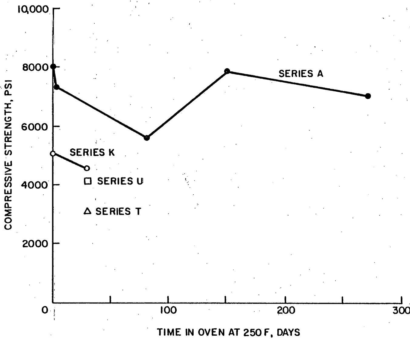
FIG. 7 - COMPRESSIVE STRENGTH OF 3x6 IN. CYLINDERS EXPOSED TO ELEVATED TEMPERATURE
