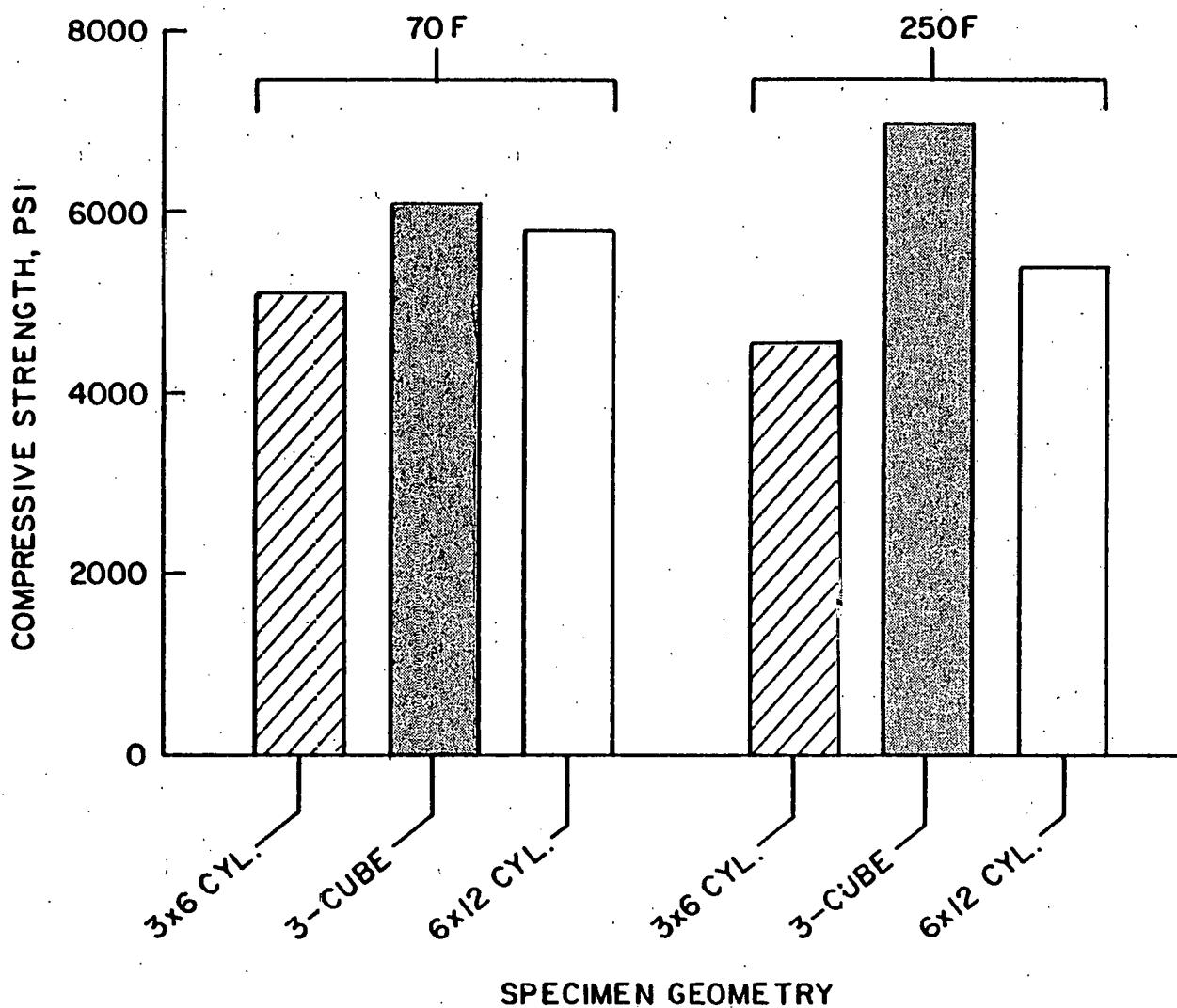
FIG. 14 - COMPARISON OF COMPRESSIVE STRENGTH VERSUS SPECIMEN GEOMETRY, SERIES K CONCRETE AT ROOM TEMPERATURE AND AFTER 30 DAYS AT 250F
