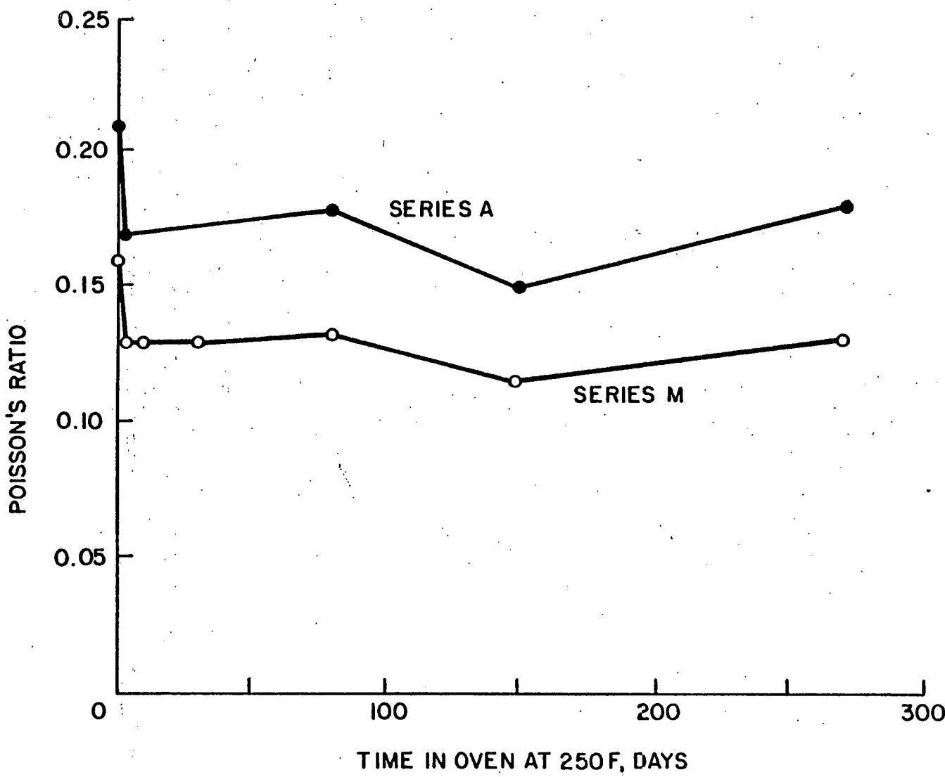
FIG. II - POISSON'S RATIO OF TANK FARM AND SERIES M CONCRETE
