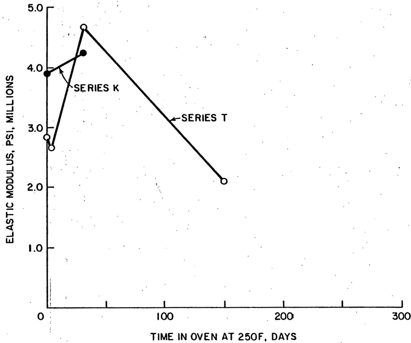
FIG. 4 - ELASTIC MODULUS OF 3-IN. CUBES EXPOSED TO ELEVATED TEMPERATURE
