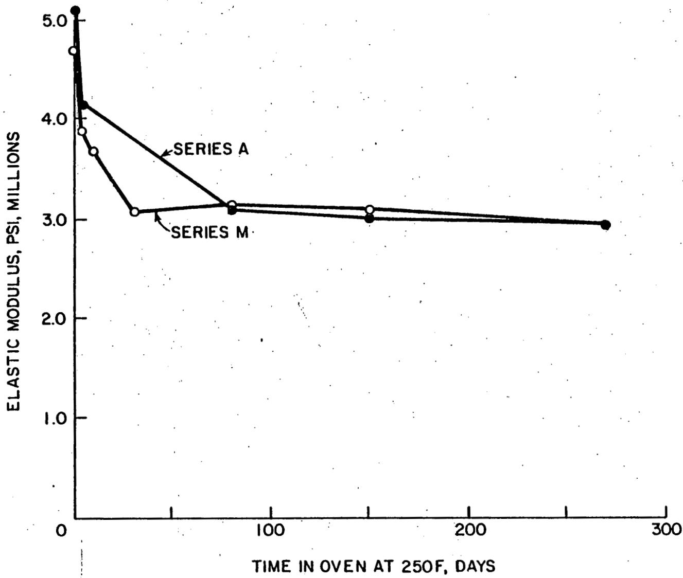
FIG. 10- ELASTIC MODULUS OF TANK FARM AND SERIES M CONCRETE EXPOSED TO ELEVATED TEMPERATURE
