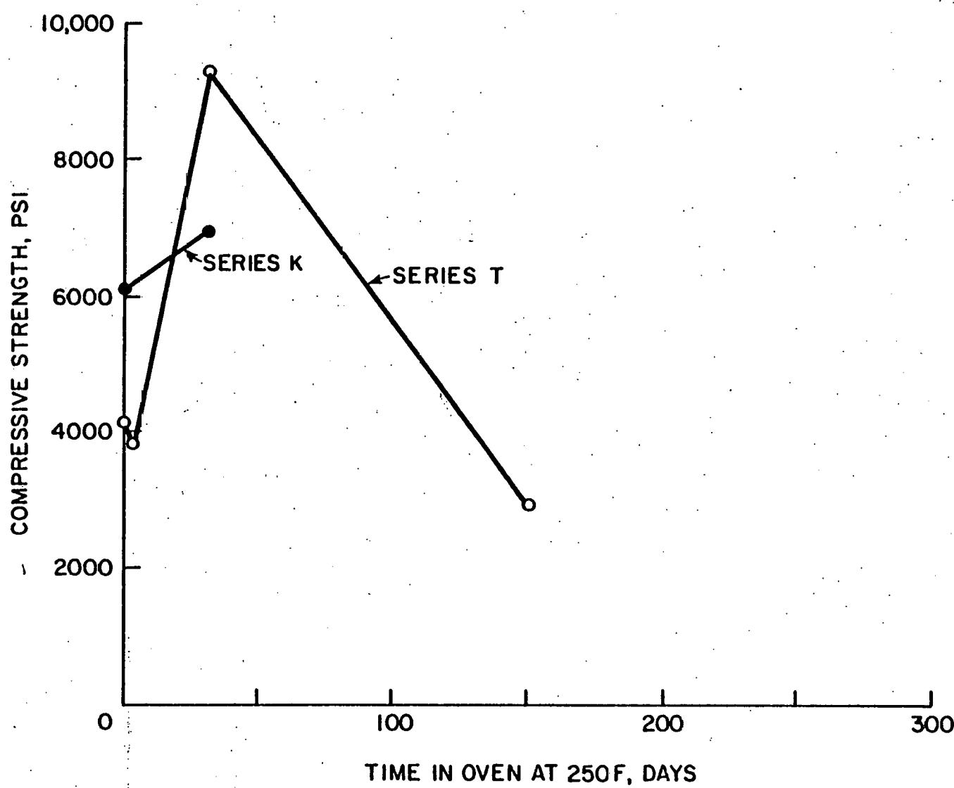
FIG. 8 - COMPRESSIVE STRENGTH OF 3-IN. CUBES EXPOSED TO ELEVATED TEMPERATURE
