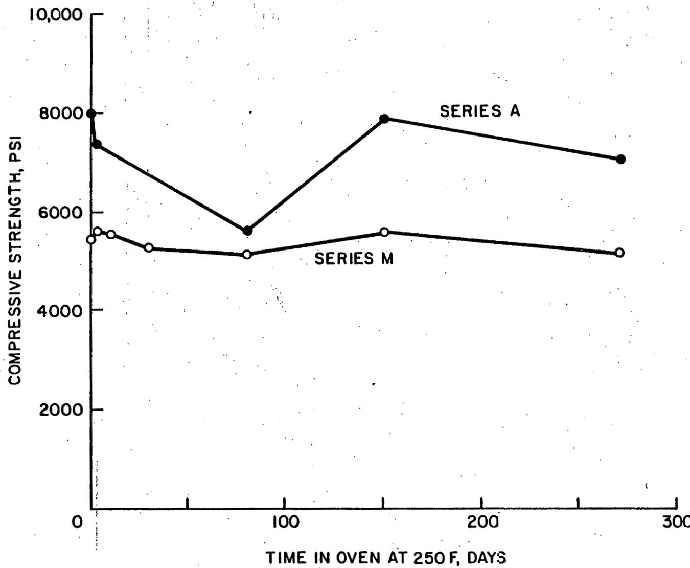
FIG. 12 - COMPRESSIVE STRENGTH OF TANK FARM AND SERIES M CONCRETE EXPOSED TO ELEVATED TEMPERATURE
