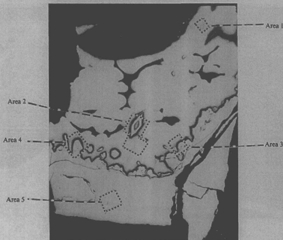
Fig. 45. Optical metallography revealed several phases on a cross section of the intermetallic blob; 40X.
