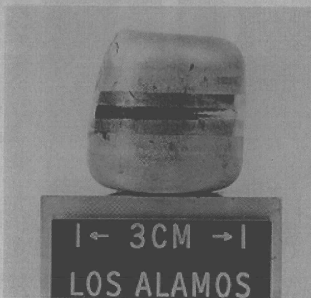
Fig. 48. Targeted GPHS fuel clad after bullet impact at 55 m/s. Note semicircular crack in upper left corner.
