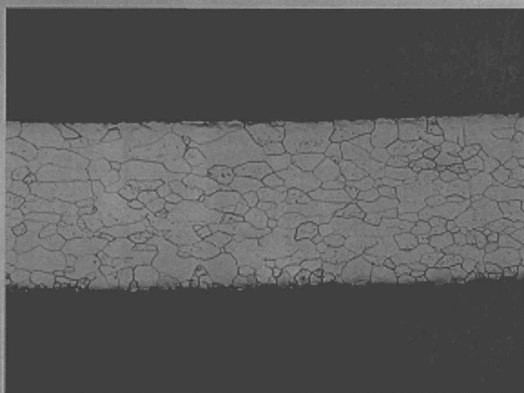
Fig. 5. The FC-589 weld shield cup had an acceptable microstructure; transverse section, 50X.
