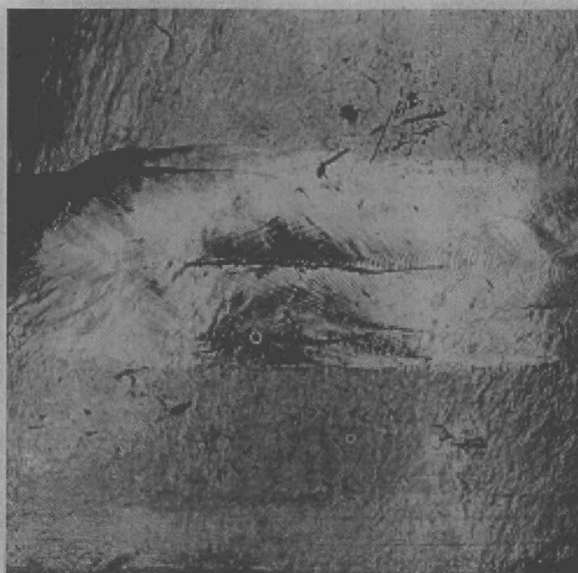
Fig. 47. Crack in the weld seam of the simulant-fueled GPHS clad after bullet impact at 555 m/s; 11X.
