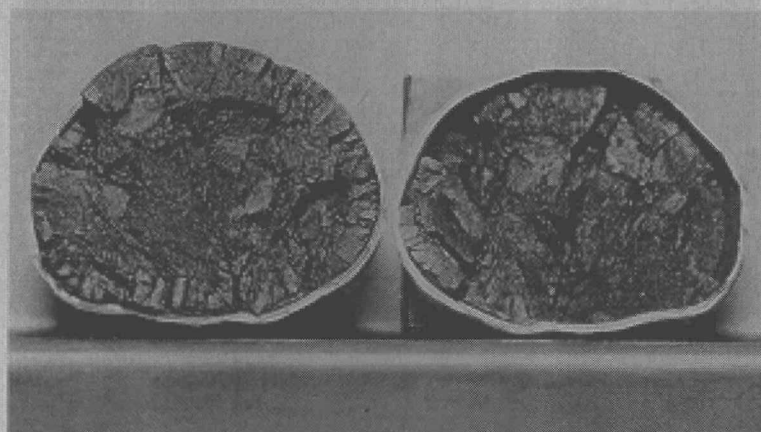
Fig. 43. The plutonia fracture pattern of FC-351 exhibited a tendency to form small, radially oriented fragments on the periphery, although the principal fracture mode was large, irregularly shaped fragments; ~1.5X.
