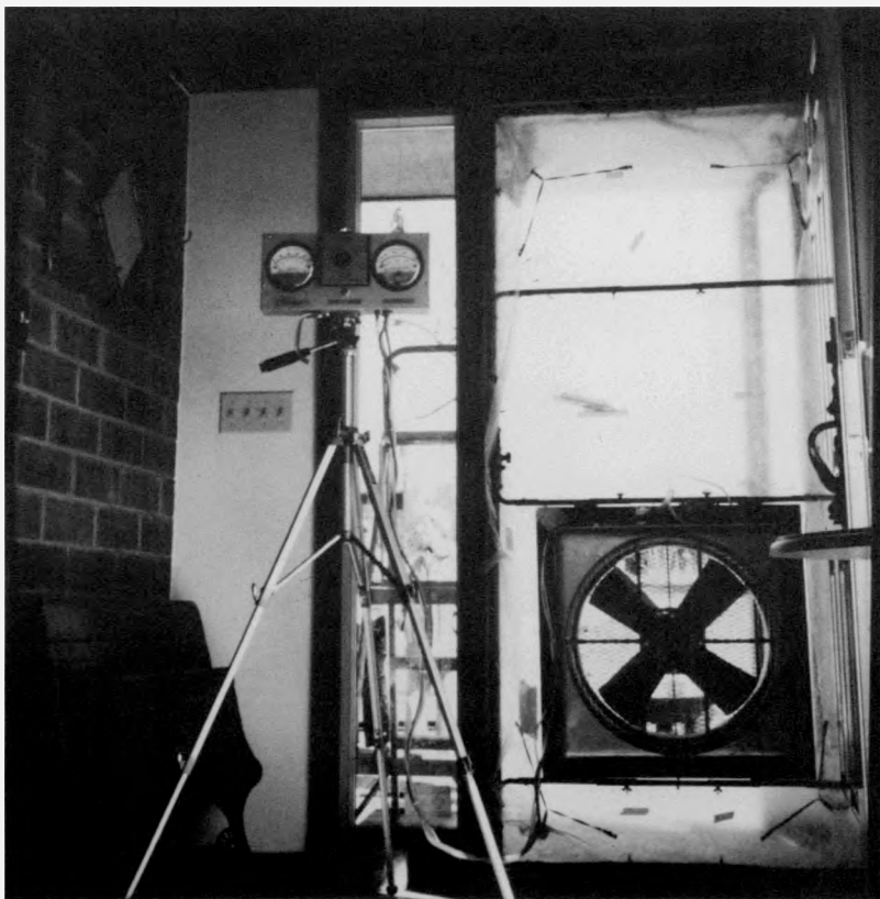
Figure 2-42. Blower door installed for testing a house. (Photograph by Steve Andrews)
