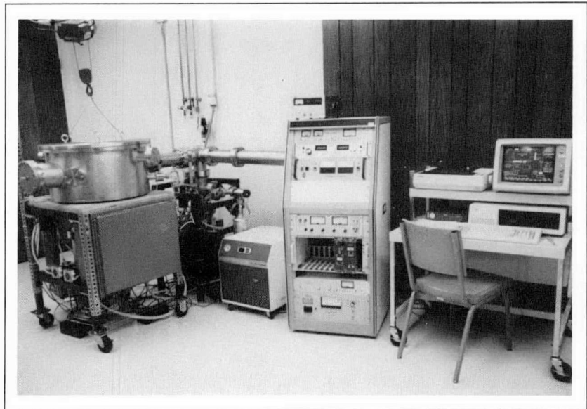
Fig. 1-37. XCALIBR II is a fully automated x-ray calibration facility that covers the energy range from 0.184 to 9.75 keV. All XCALIBR II operations are monitored and controlled by an IBM® PC-XT. The facility includes a vacuum chamber for test instruments, a point x-ray source, and a variety of pumps.
