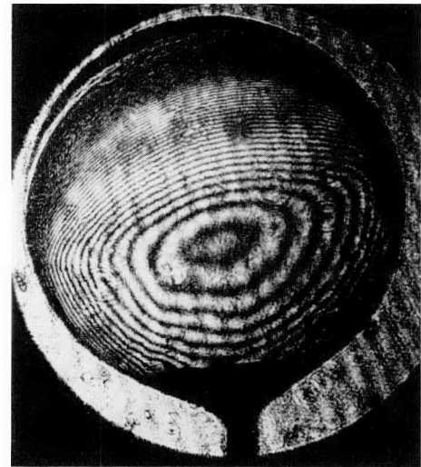
Fig. 2-25. The holographic interferometry system was used to produce this image of an inverted liquid layer within a 680 \mu\text{m} polymer-coated glass shell. The liquid is a 1:1 mixture of hydrogen and deuterium. The fringes are attributable only to the fuel layer. The only effect of the thick wall of the fuel container is the refraction of light out of the entrance pupil of the viewing optics, which produces the shadows at the edges of the shell image.
