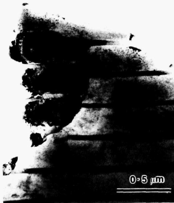
Fig. 1.1.18. Transmission electron micrograph of stoichiometric, rapidly solidified Ni 3 Al powder.
