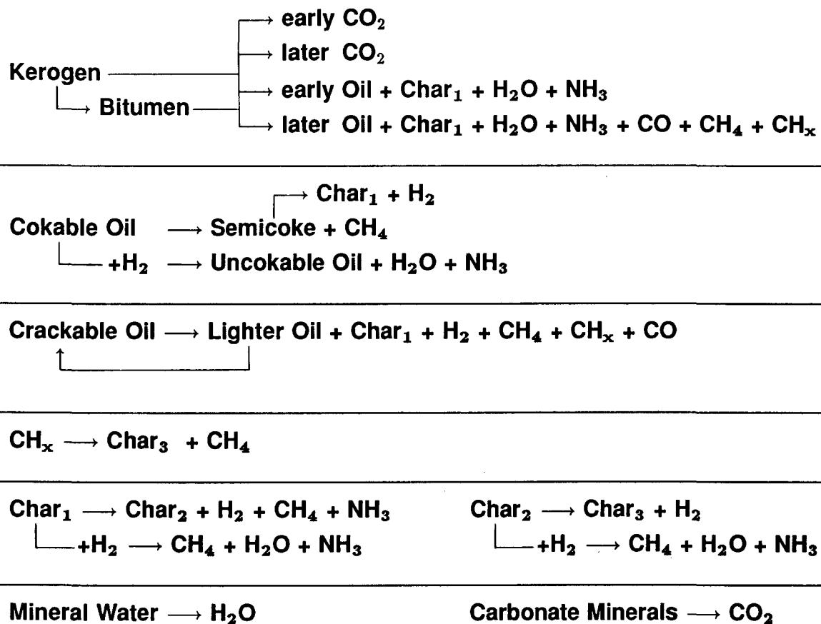
Figure 2. A schematic representation of the chemical reaction framework of PYROL. The complete model consists of time derivatives of 32 vapor species, 32 liquid species, 19 solid species, and 67 other variables, including pore pressure, pore volume, and diagnostics.
