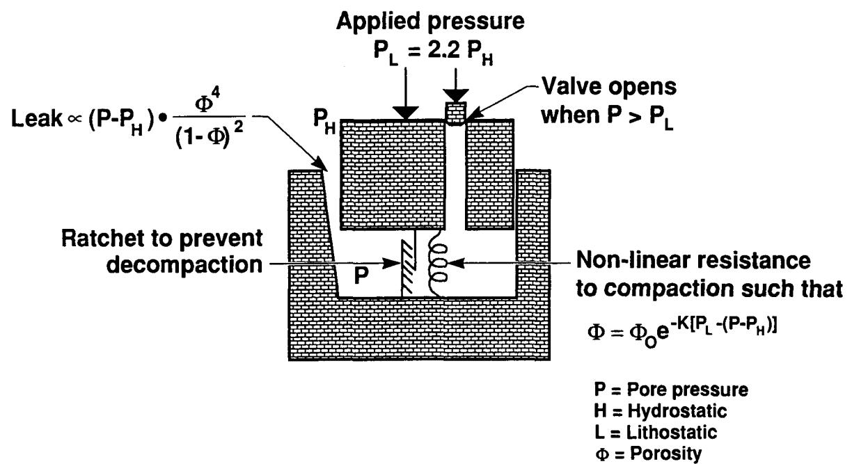
Figure 6. Schematic representation of the compaction model used in PYROL.
