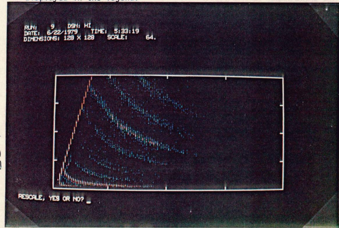
(b) Contour plot of counter telescope data obtained with 128 - MeV  $^{160}\text{O}$  on  $^{40}\text{Ca}$  at  $\theta_{\text{lab}} = .25^\circ$ . Brighter colors indicate regions of higher counting rate. The moderately intense group at left center is  $^{160}\text{O}$ ; that toward the lower left corner is  $^4\text{He}$ .
