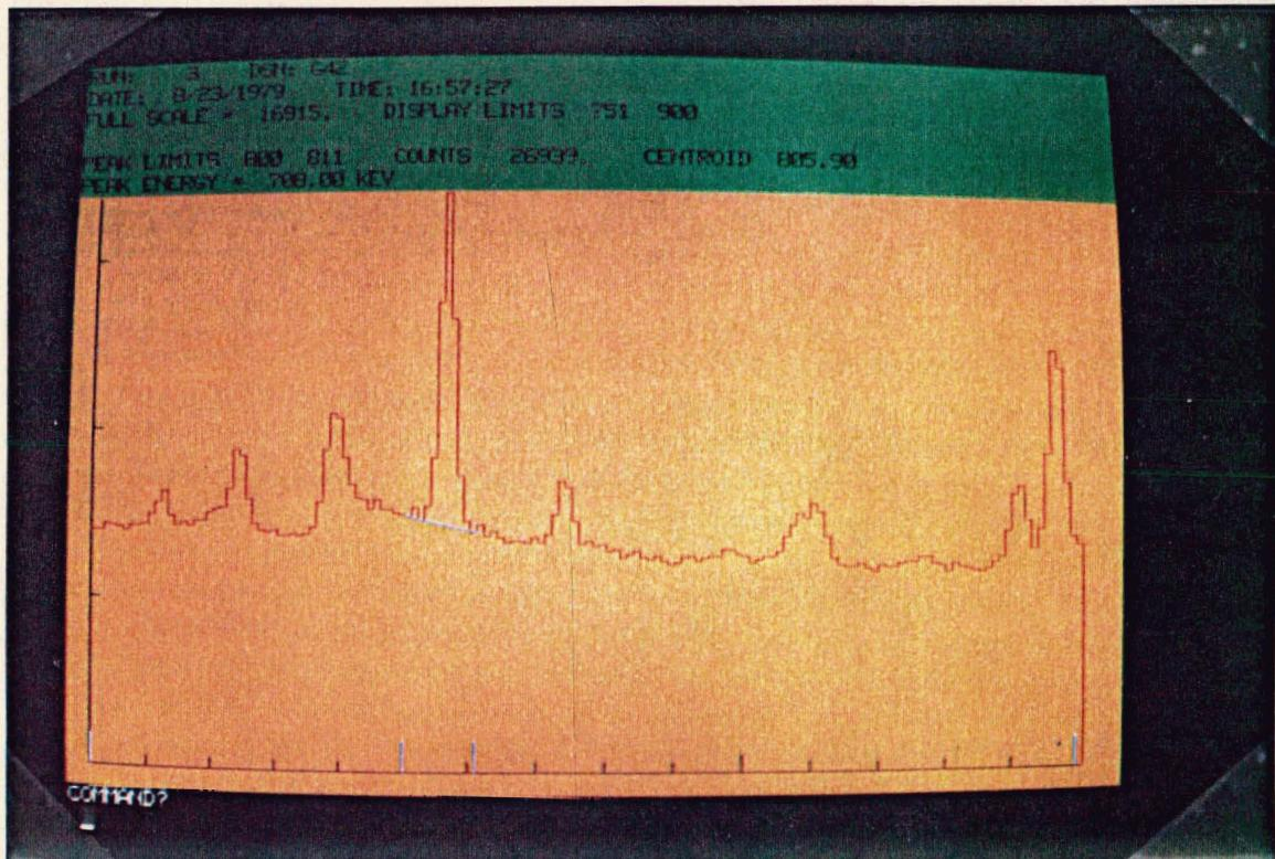
(a) Portion of a Ge(Li) spectrum from 40 - MeV  $^{160}\text{O}$  on  $^{26}\text{Mg}$ . A typical use of the background subtraction procedure, done with cross-hair cursors, is shown. The net peak counts, centroid and energy are displayed in the legend.
