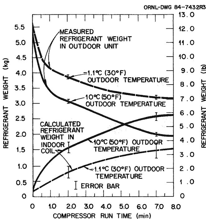
Fig. 5.12. On period refrigerant charge distribution as affected by outdoor temperature for cycling tests have 8-min-on and 30-min-off cycling rate.
