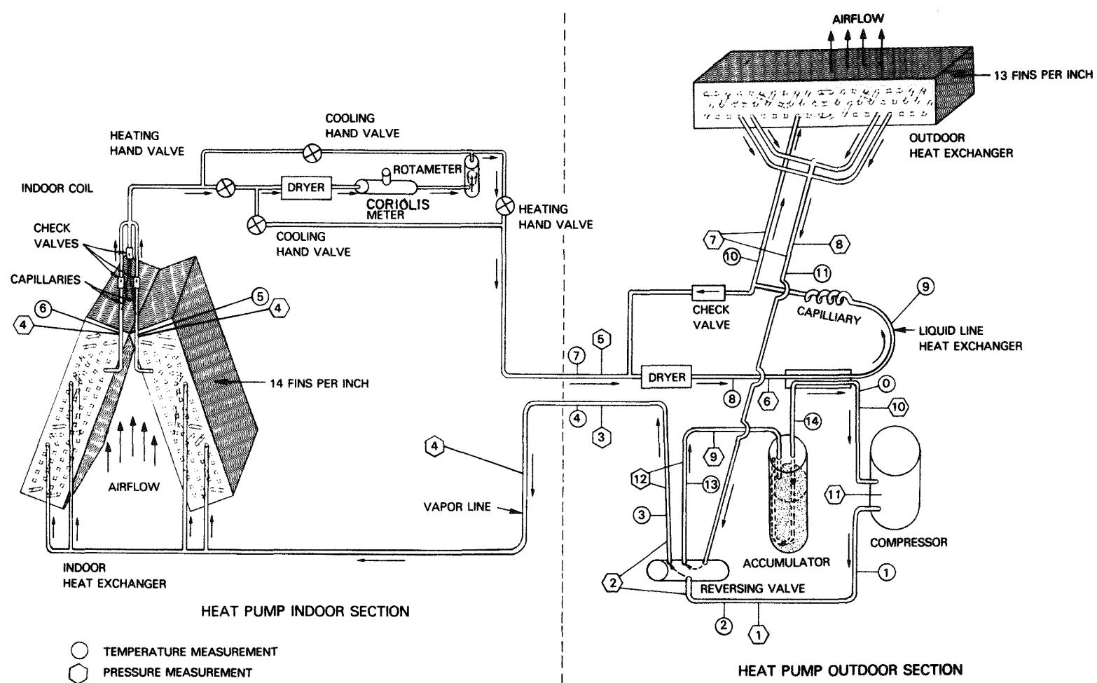
Fig. 3.1. Heat pump refrigerant sensor locations.
