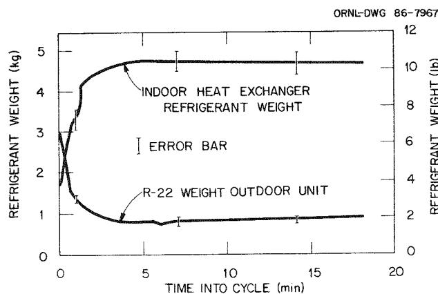
Fig. 7.6. Refrigerant weight distribution observed during the off cycle of a 10-min-on and 20-min-off cooling mode cycling test conducted at 28°C (82°F) outdoor air temperature.
