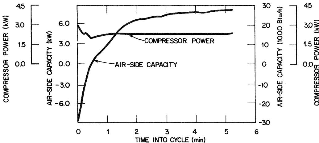
Fig. 6.27. Recovery following defrosting conducted at  $1.7^{\circ}\text{C}$  ( $35^{\circ}\text{F}$ ) outdoor temperature and 70% relative humidity.
