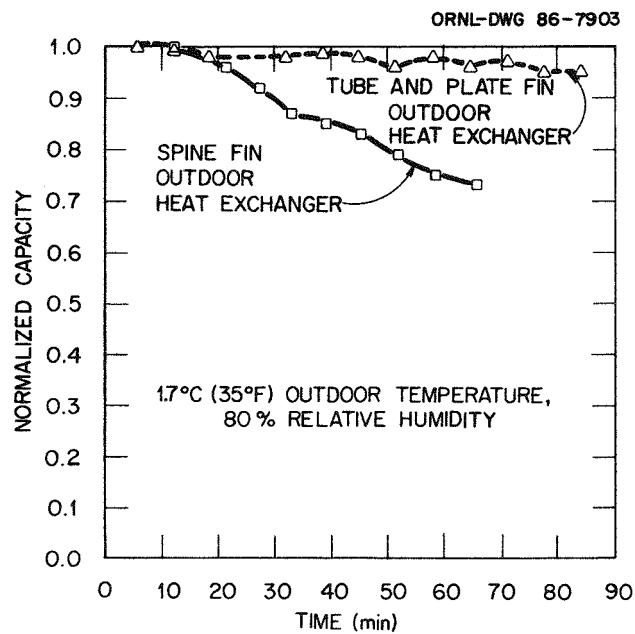
Fig. 6.8. Normalized capacity for two heat pumps, one having a spine fin outdoor coil and the other having tube and plate fin outdoor coil.
