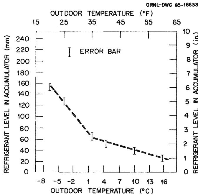
Fig. 5.4. Refrigerant level in accumulator.
