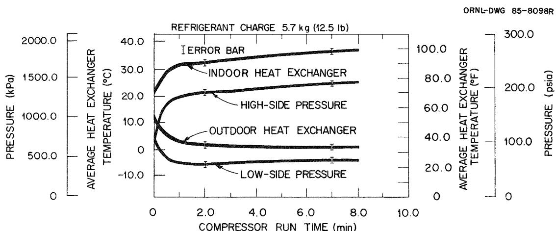
Fig. 5.9. Average heat exchanger temperature and refrigerant pressure measured during the on period of an 8-min-on and 30-min-off cycling test conducted at  $10^{\circ}\text{C}$  ( $50^{\circ}\text{F}$ ) outdoor temperature.
