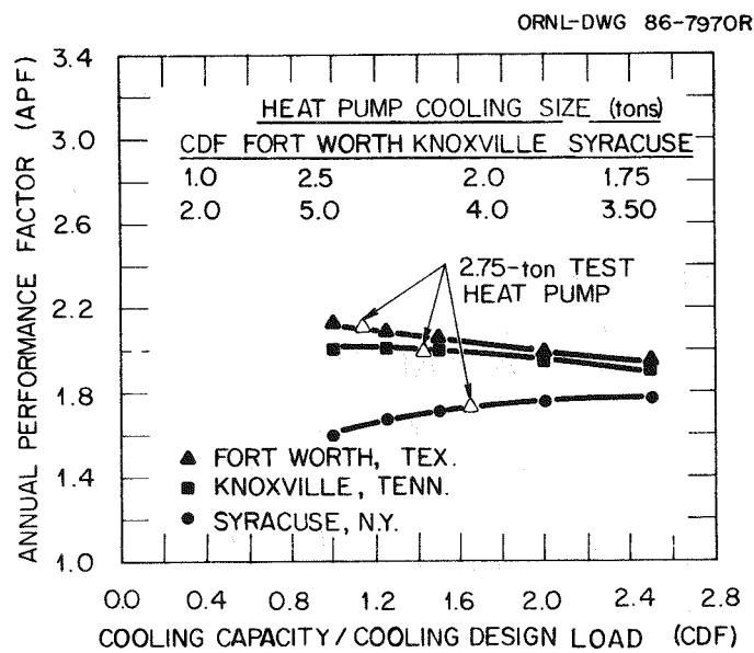
Fig. 8.9. Annual performance factor as a function of heat pump size.
