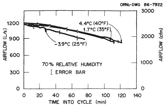
Fig. 6.15. Outdoor airflow measured under frosting conditions with relative humidity fixed at 70%.
