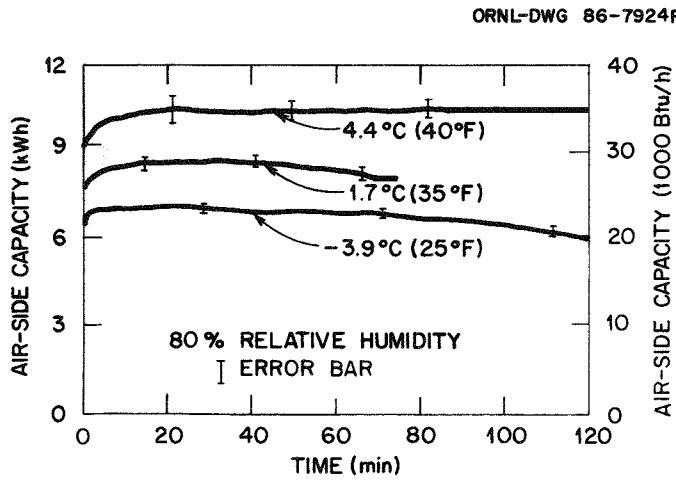
Fig. 6.18. Air-side capacity measured during frosting tests with 80% outdoor relative humidity.
