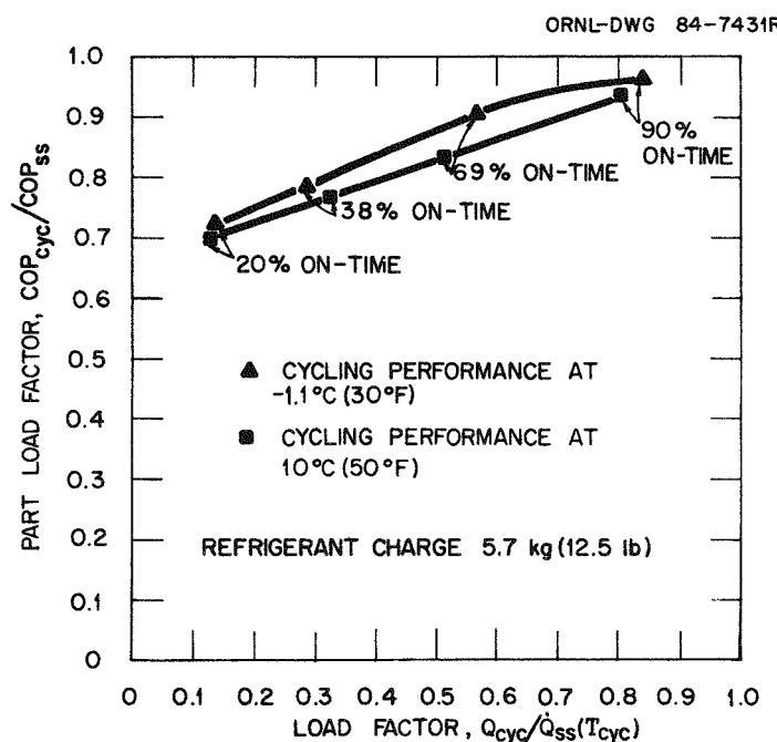
Fig. 5.10. Outdoor temperature affect on heat pump part-load factor.
