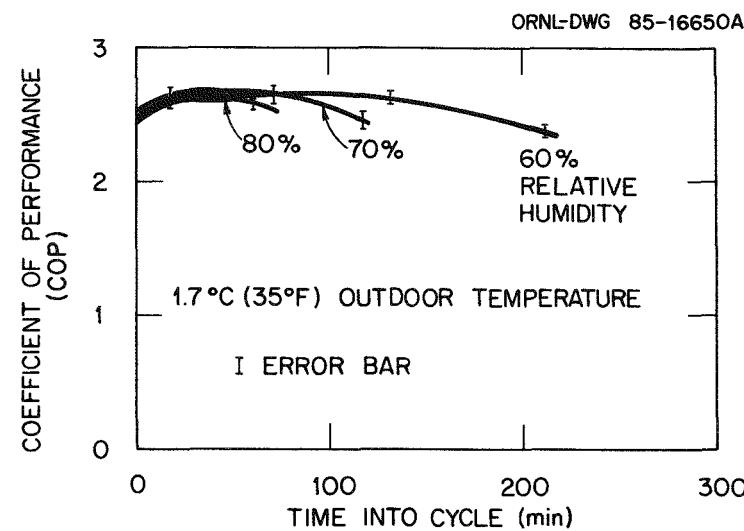
Fig. 6.1. The COP observed for frosting tests conducted at an outdoor air temperature of 1.7°C (35°F).
