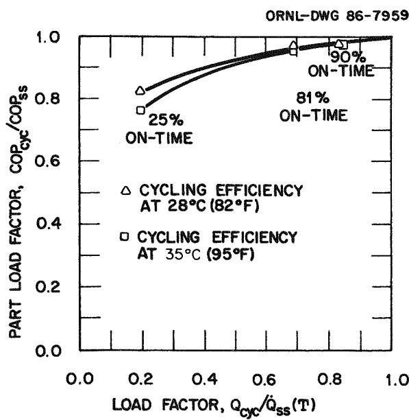
Fig. 7.10. Cooling mode cycling efficiency as affected by outdoor air temperature.
