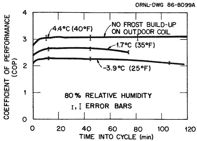
Fig. 6.17. COP observed for various outdoor temperature frosting tests with 80% outdoor relative humidity.
