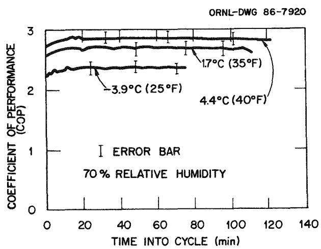
Fig. 6.13. The COP observed for various outdoor temperatures with relative humidity fixed at 70%.
