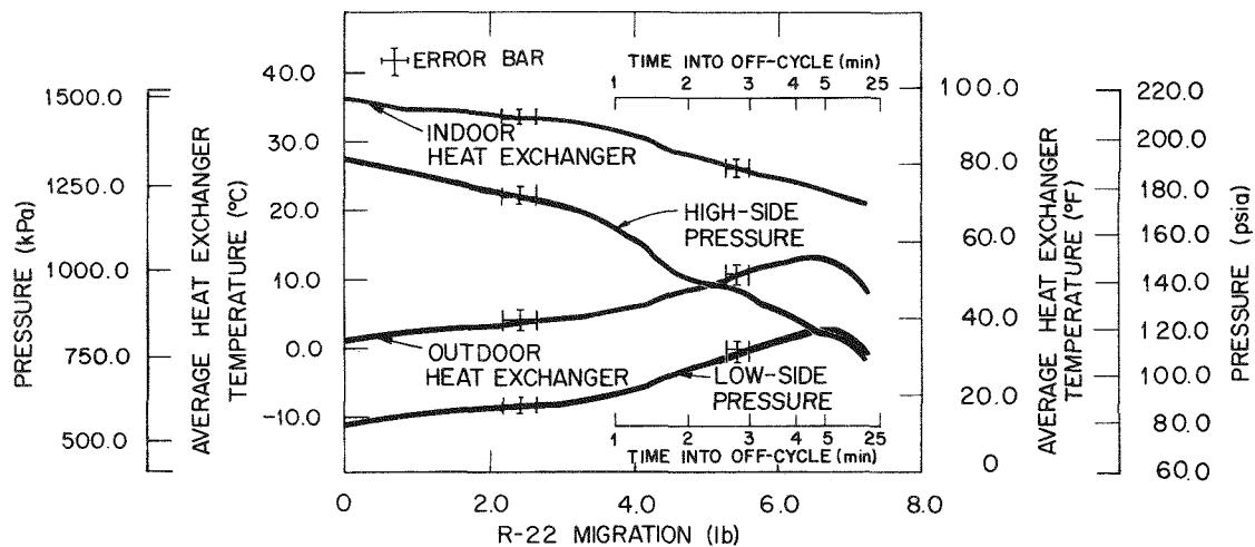
Fig. 5.6. Average heat exchanger temperature and refrigerant pressure plotted as a function of refrigerant migration to the outdoor unit during the off cycle of an 8-min-on and 30-min-off cycling test conducted at 10°C (50°F) outdoor temperature.
