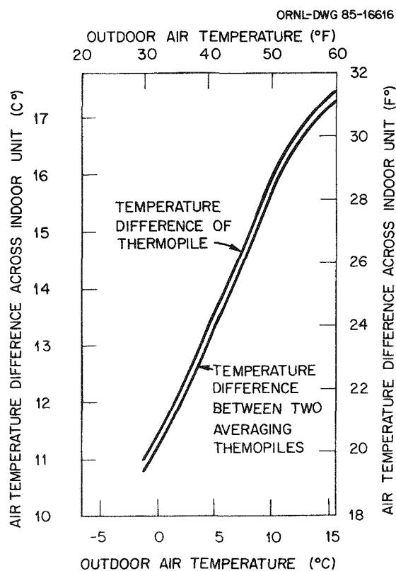
Fig. 3.4. Air temperature measurement comparison between two measuring techniques.
