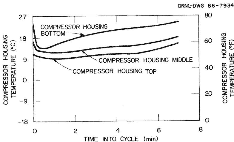
Fig. 6.25. Compressor housing temperature measured during defrost with  $1.7^{\circ}\text{C}$  ( $35^{\circ}\text{F}$ ) outdoor air temperature and 70% relative humidity.
