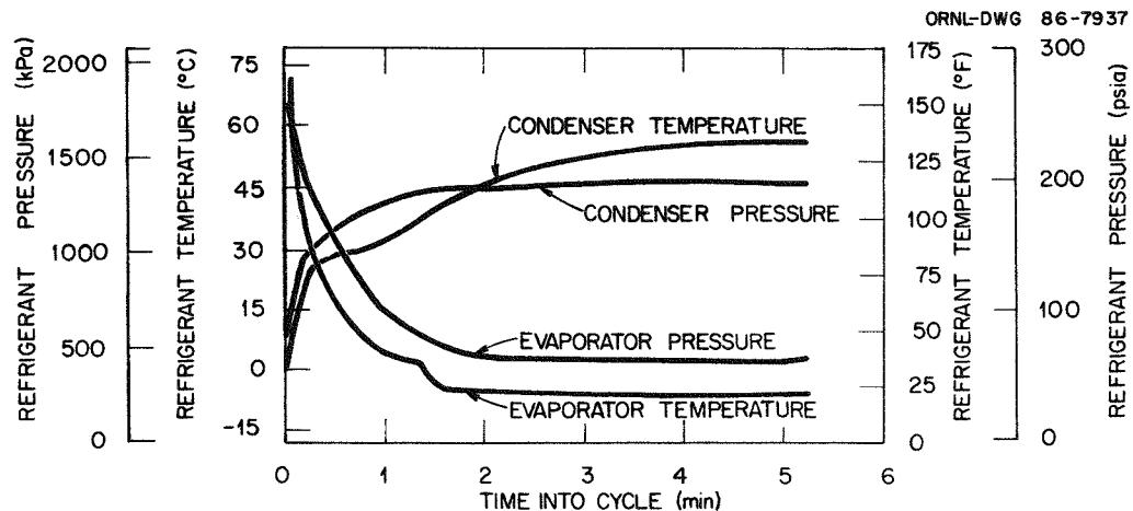
Fig. 6.28. High-side and low-side refrigerant pressures and temperatures measured during recovery with  $1.7^{\circ}\text{C}$  ( $35^{\circ}\text{F}$ ) outdoor air temperature and 70% relative humidity.
