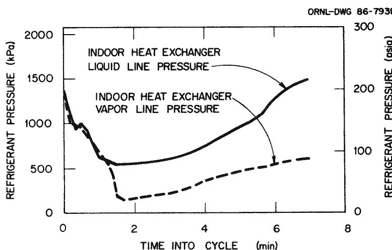
Fig. 6.22. Refrigerant pressures measured across the indoor capillary tubes during defrost with 1.7°C (35°F) outdoor air temperature and 70% relative humidity.
