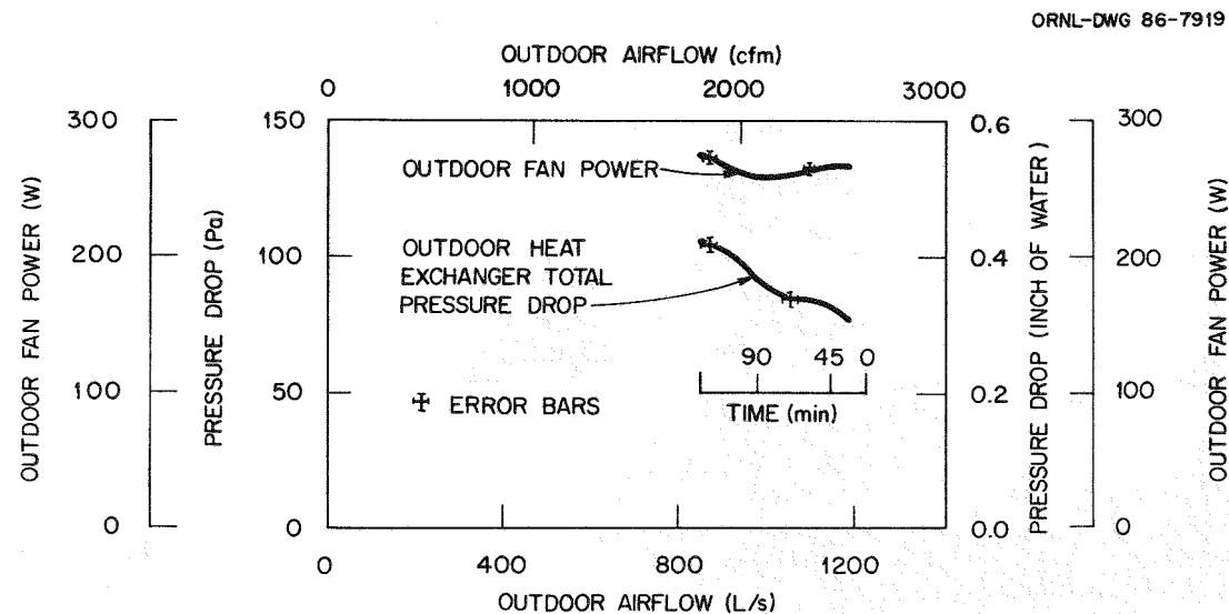
Fig. 6.12. Outdoor propeller fan characteristics observed during frosting test conducted at 1.7°C (35°F) outdoor temperature and 70% relative humidity.
