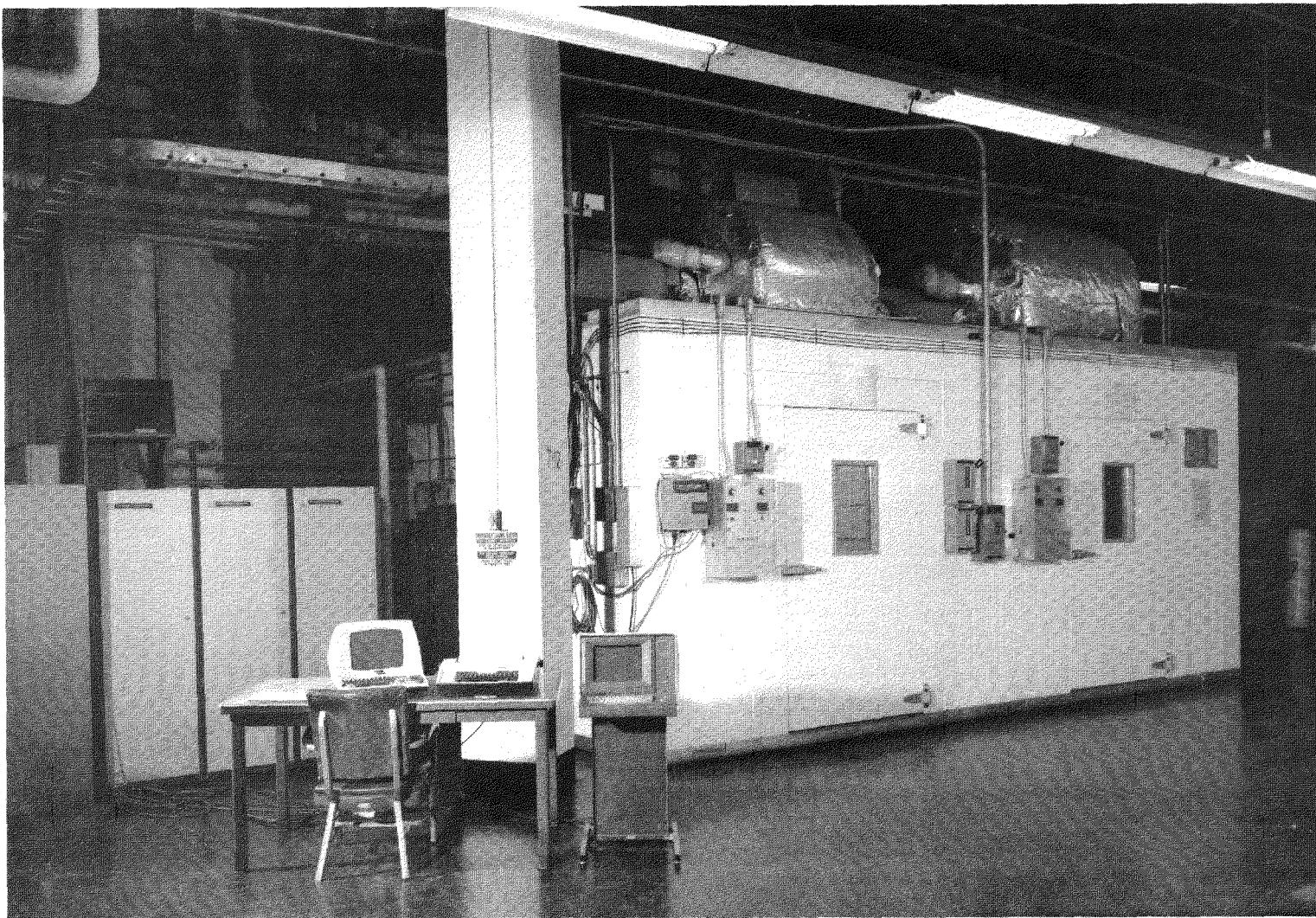
Fig. 3.2. Environmental chambers and data acquisition system.
