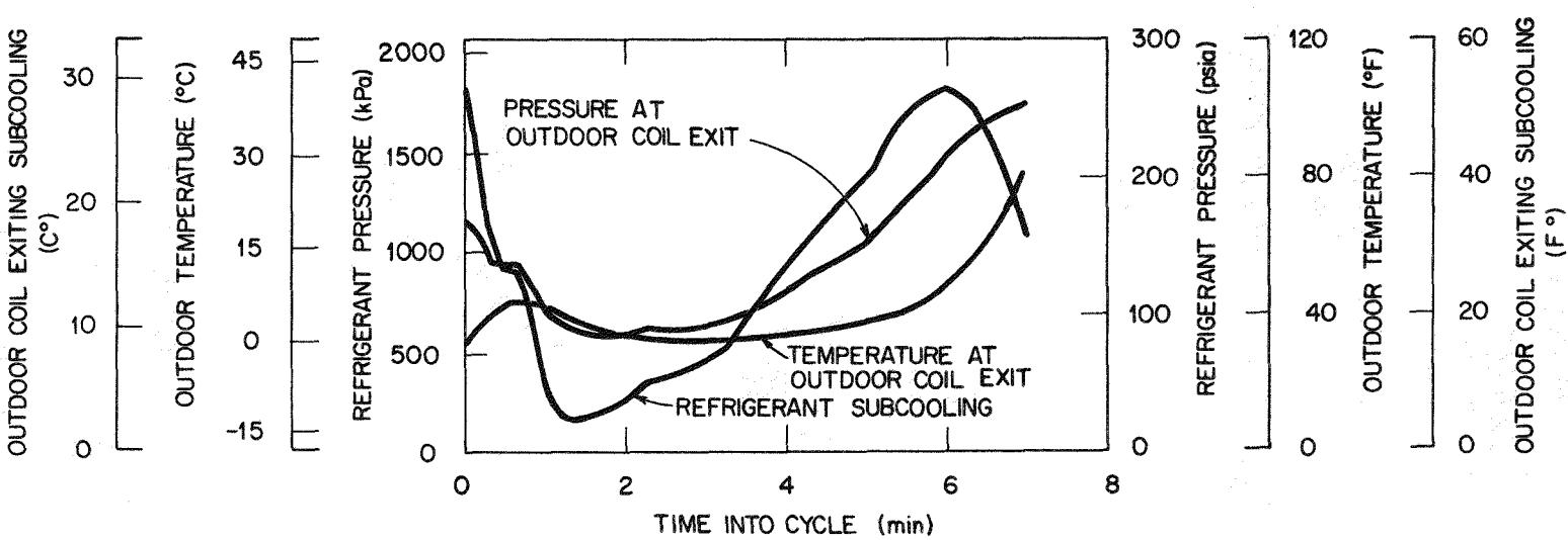
Fig. 6.26. The state point of refrigerant exiting the outdoor coil during defrost conducted at  $1.7^{\circ}\text{C}$  ( $35^{\circ}\text{F}$ ) outdoor air temperature and 70% relative humidity.
