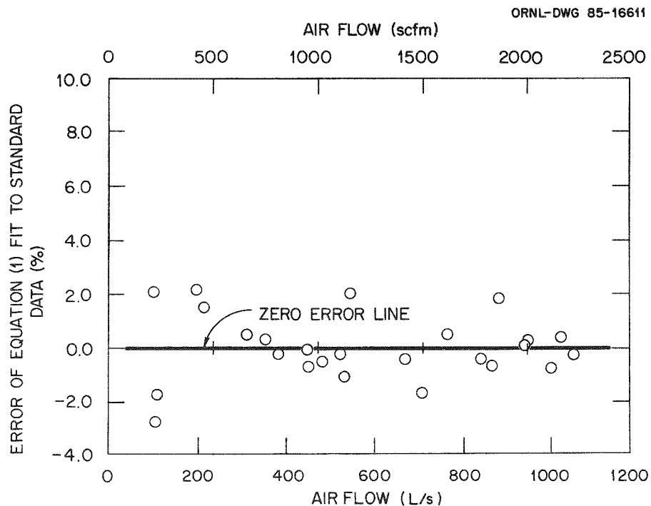
Fig. 3.3. Multipoint Pitot tube calibration data for indoor airflow.
