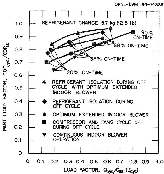
Fig. 5.13. Heat pump heating mode cycling COP observed at 10°C (50°F) outdoor temperature for various cycling control strategies.
