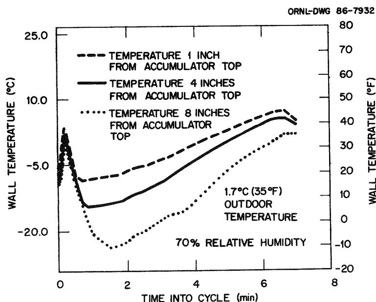
Fig. 6.23. Accumulator wall temperatures measured during defrost with 1.7°C (35°F) outdoor air temperature and 70% relative humidity.
