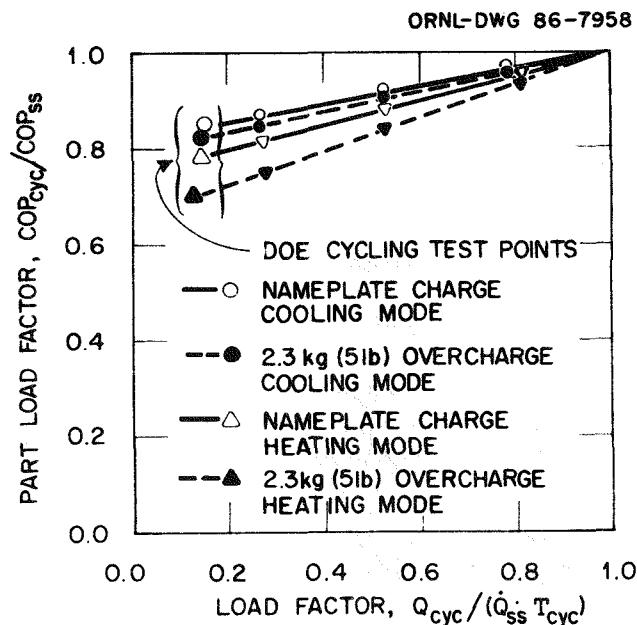
Fig. B.1. Part-load efficiency as affected by refrigerant overcharge.
