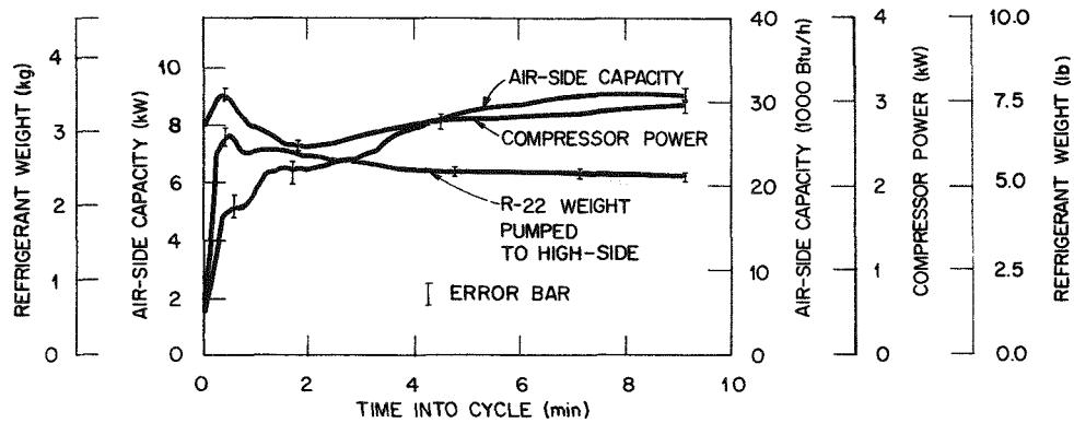
Fig. 7.7. Capacity, compressor power, and refrigerant pumped to high side during the on cycle of a 10-min-on and 20-min-off cooling mode cycling test conducted at 28°C (82°F) outdoor air temperature.
