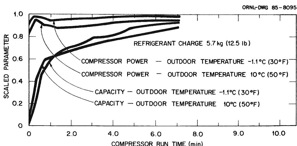
Fig. 5.11. Capacity and compressor power, normalized to steady state value, for the on period of 8-min-on and 30-min-off cycling tests.
