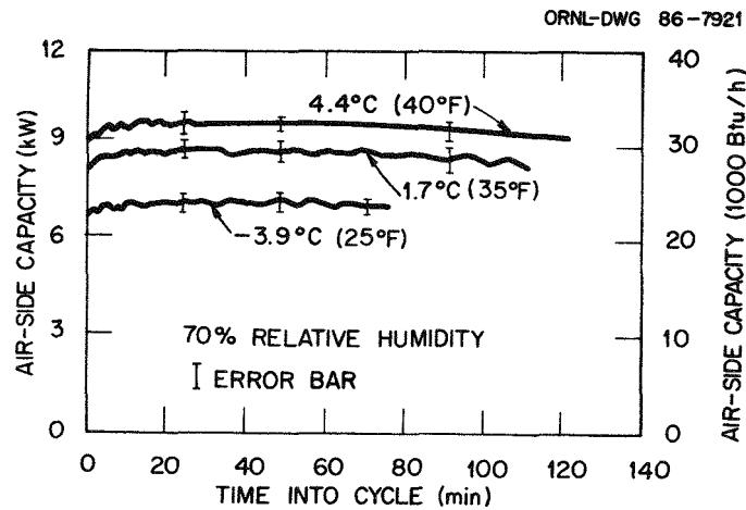
Fig. 6.14. Air-side capacity measured under frosting conditions at various outdoor temperatures with relative humidity fixed at 70%.
