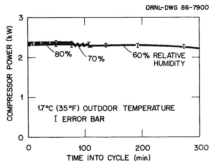
Fig. 6.6. Compressor power consumption observed for frosting tests conducted at 1.7°C (35°F) outdoor air temperature.
