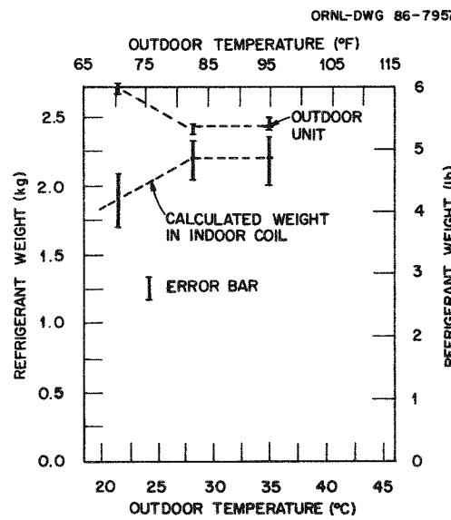
Fig. 7.4. Refrigerant weight distribution during steady state cooling mode operation.
