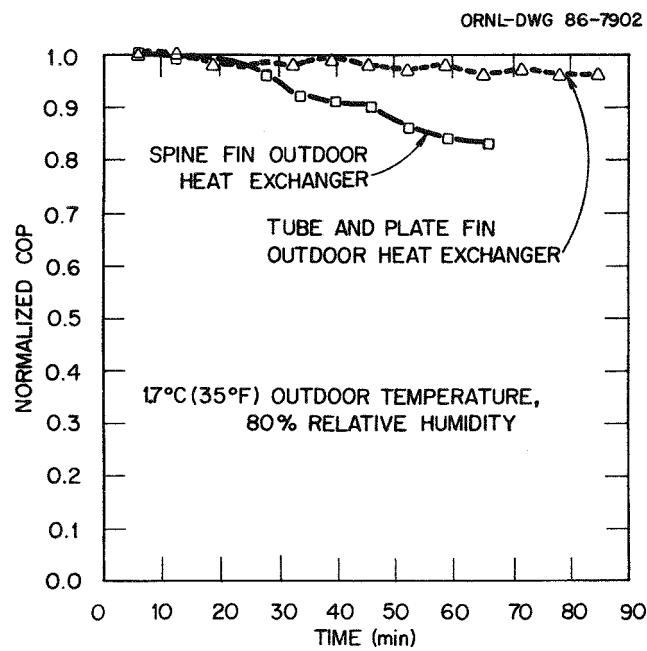
Fig. 6.7. Normalized COP for two heat pumps, one having a spine fin outdoor coil and the other having a tube and plate fin outdoor coil.
