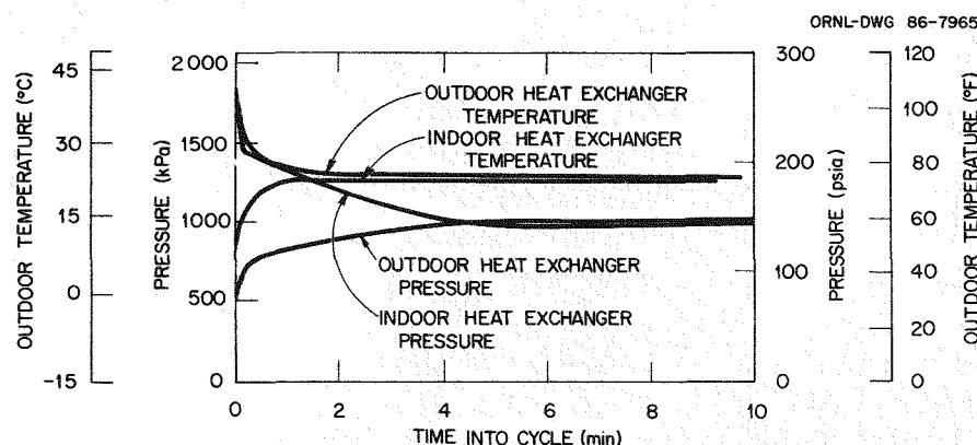
Fig. 7.5. Condenser and evaporator refrigerant temperatures and pressures observed during the off cycle of a 10-min-on and 20-min-off cooling mode cycling test conducted at 28°C (82°F) outdoor air temperature.
