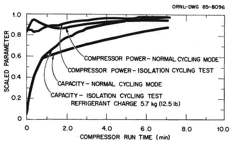
Fig. 5.14. Capacity and compressor power, normalized to steady state, for comparison of normal mode cycling to cycling with off-cycle isolation of refrigerant in the indoor coil.
