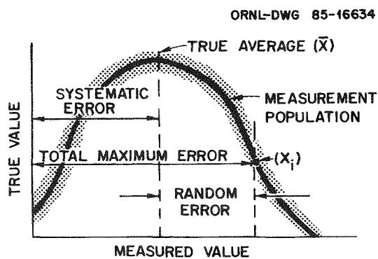
Fig. 4.1. Measurement errors.
