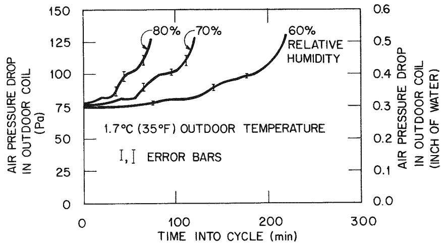
Fig. 6.3. Air total pressure drop measured across the outdoor coil under frosting conditions at 1.7°C (35°F) outdoor air temperature.
