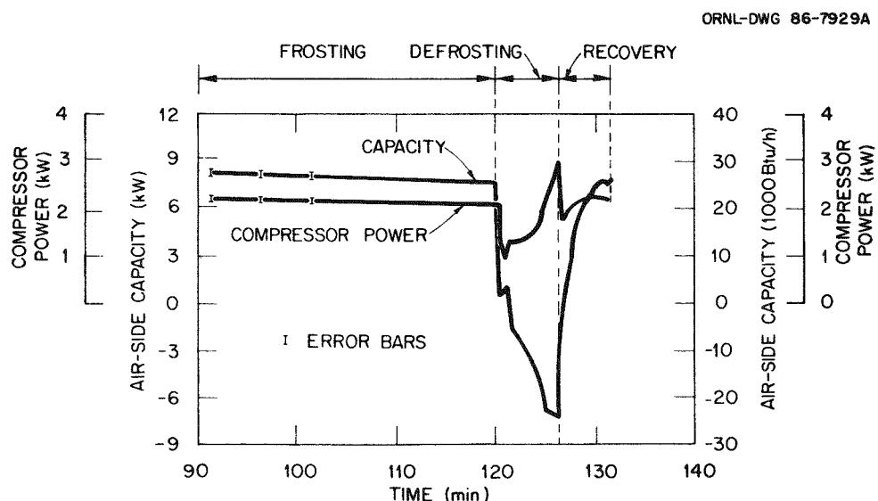
Fig. 6.19. Frosting-defrosting-recovery test conducted at  $1.7^{\circ}\text{C}$  ( $35^{\circ}\text{F}$ ) outdoor air temperature and 70% relative humidity.
