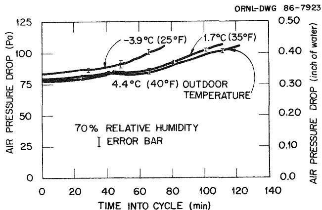
Fig. 6.16. Air total pressure drop measured across the outdoor coil for frosting tests with 70% outdoor relative humidity.
