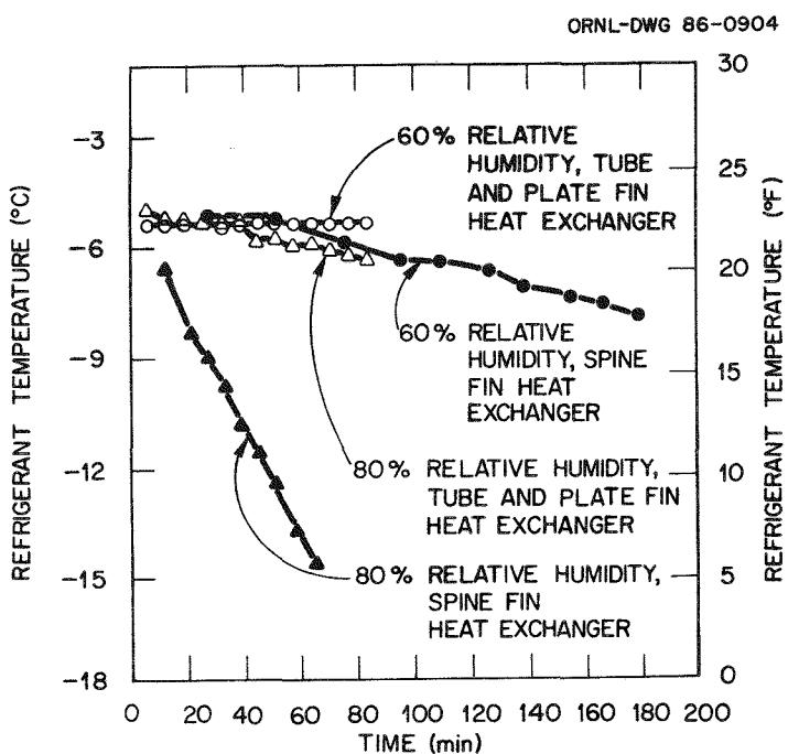
Fig. 6.9. Refrigerant temperature measured within the outdoor coils of the spine fin and the tube and plate fin heat exchangers for tests conducted at 1.7°C (35°F) outdoor temperature with 60 and 80% relative humidity.
