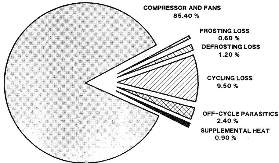
Fig. 8.4. Portions of energy as a percentage of total yearly energy for the test heat pump (with demand defrost initiator) operating in Fort Worth, Texas.
