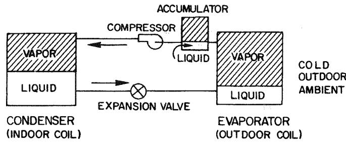
Fig. 6.20. Refrigerant inventory during defrost and recovery.
