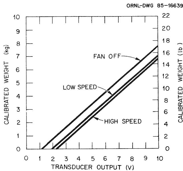
Fig. 3.6. Refrigerant weight scale calibration.
