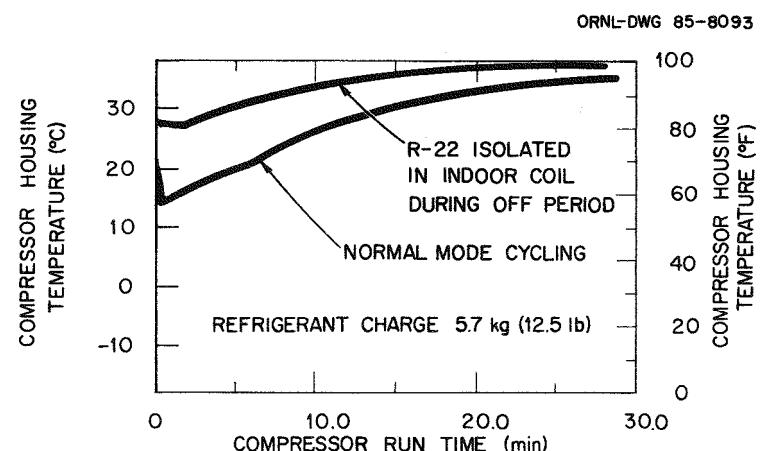
Fig. 5.15. Compressor housing temperature, measured at compressor oil level, for cycling tests having off-cycle refrigerant migration control and normal mode control [uncertainty in housing temperature  $\pm 0.3^{\circ}\text{C}$  ( $0.5^{\circ}\text{F}$ ) at 20:1 odds].
