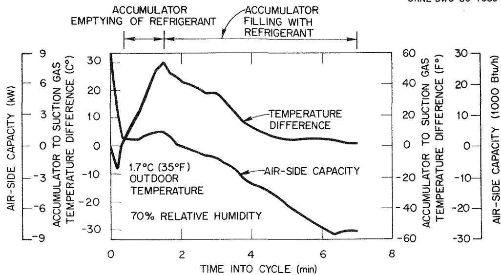
Fig. 6.24. Air-side capacity during defrost as affected by the time required to pump refrigerant from the accumulator.
