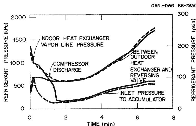
Fig. 6.21. High-side and low-side refrigerant pressures and temperatures measured during defrost with 1.7°C (35°F) outdoor air temperature and 70% relative humidity.
