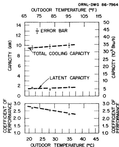
Fig. 7.1. Steady state cooling mode performance.
