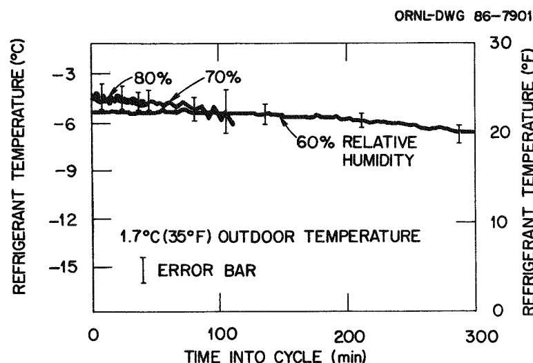
Fig. 6.5. Saturated refrigerant temperature in the outdoor coil for frosting tests conducted at 1.7°C (35°F) outdoor air temperature.
