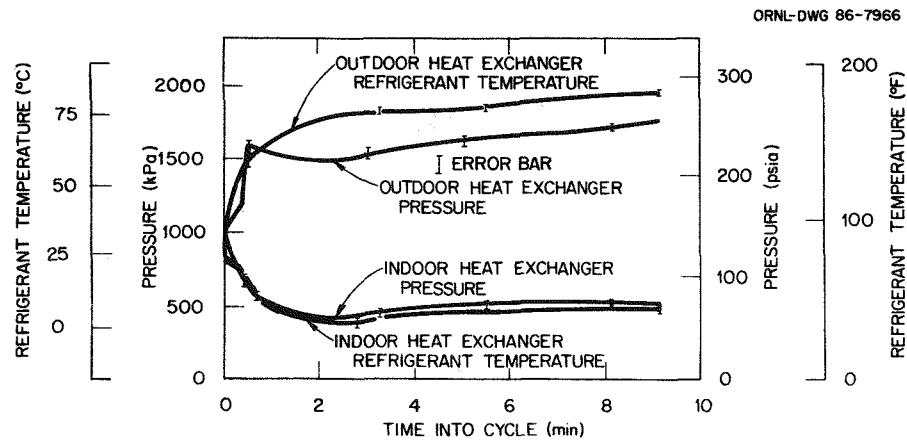
Fig. 7.8. Condenser and evaporator refrigerant temperatures and pressures observed during the on cycle of a 10-min-on and 20-min-off cooling mode cycling test conducted at 28°C (82°F) outdoor air temperature.
