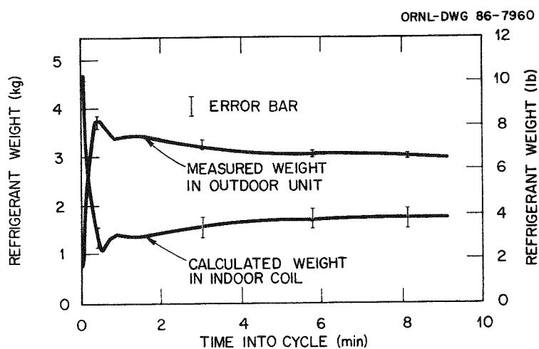
Fig. 7.9. Refrigerant weight distribution observed during the on cycle of a 10-min-on and 20-min-off cooling mode cycling test conducted at 28°C (82°F) outdoor air temperature.
