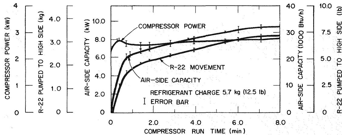
Fig. 5.8. Capacity, compressor power, and refrigerant pumped to the high side during the on period of an 8-min-on and 30-min-off cycling test conducted at 10°C (50°F) outdoor temperature.
