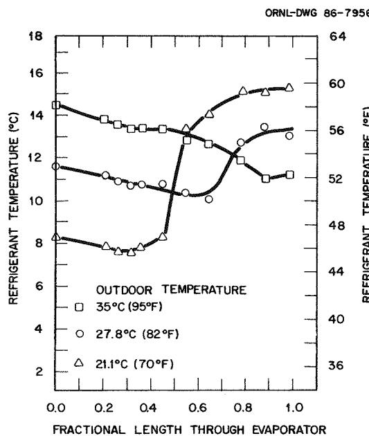
Fig. 7.2. Refrigerant temperature profile through the evaporator.
