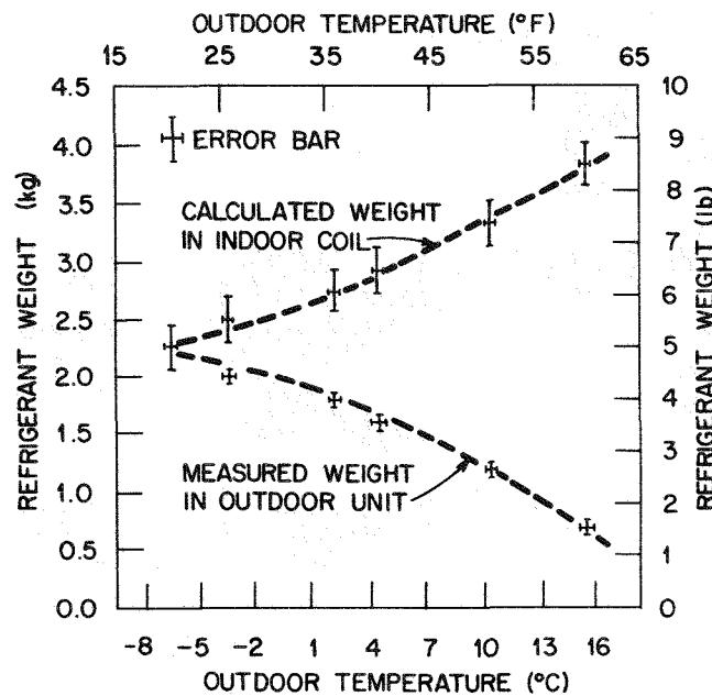
Fig. 5.5. Heat pump refrigerant charge distribution.
