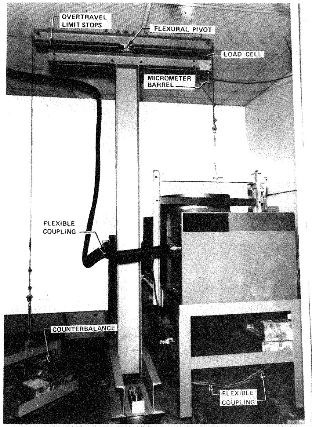
Fig. 3.5. Weighing system for measurement of refrigerant weight in the outdoor unit.
