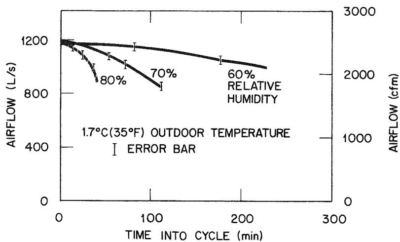
Fig. 6.4. Outdoor airflow measured under frosting conditions at 1.7°C (35°F) outdoor air temperature.
