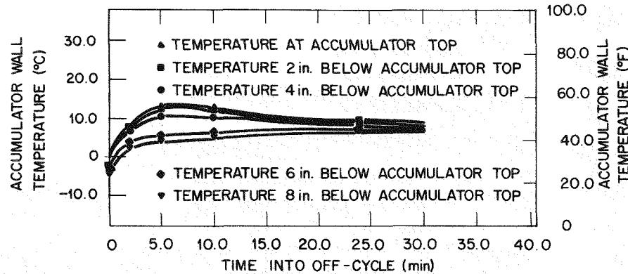
Fig. 5.7. Accumulator wall temperatures observed during the off cycle of an 8-min-on and 30-min-off cycling test conducted at 10°C (50°F) outdoor temperature [uncertainty in wall temperature  $\pm 0.3^\circ\text{C}$  (0.5°F) at 20:1 odds].
