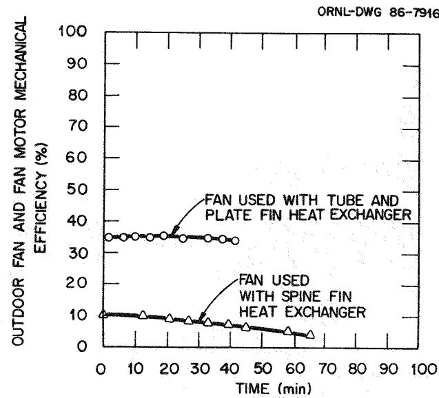
Fig. 6.11. Outdoor fan and motor efficiency measured for the two heat pumps operating under 1.7°C (35°F) outdoor temperature with 80% relative humidity.
