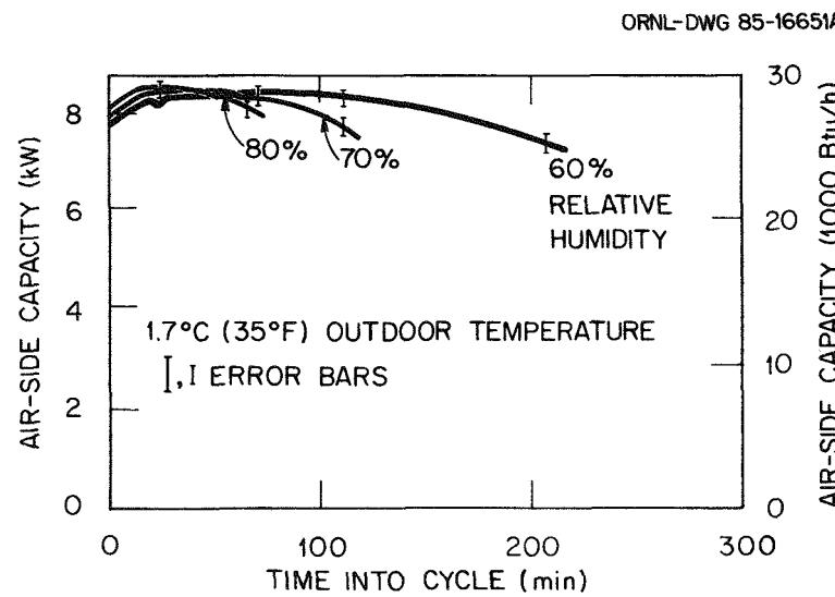
Fig. 6.2. Air-side capacity measured during frosting tests conducted at 1.7°C (35°F) outdoor air temperature.
