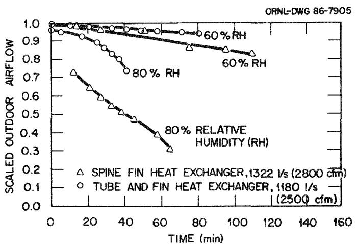
Fig. 6.10. Outdoor airflow, scaled to respective freeflow value for each heat pump for tests conducted at 1.7°C (35°F) outdoor temperature with 60 and 80% relative humidity.
