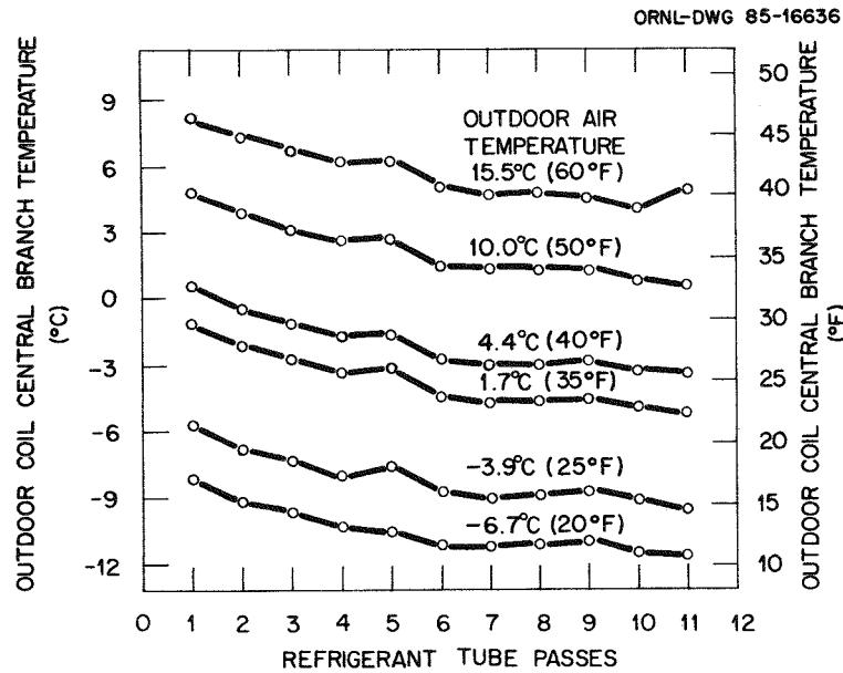
Fig. 5.3. Outdoor heat exchanger refrigerant temperature profile.
