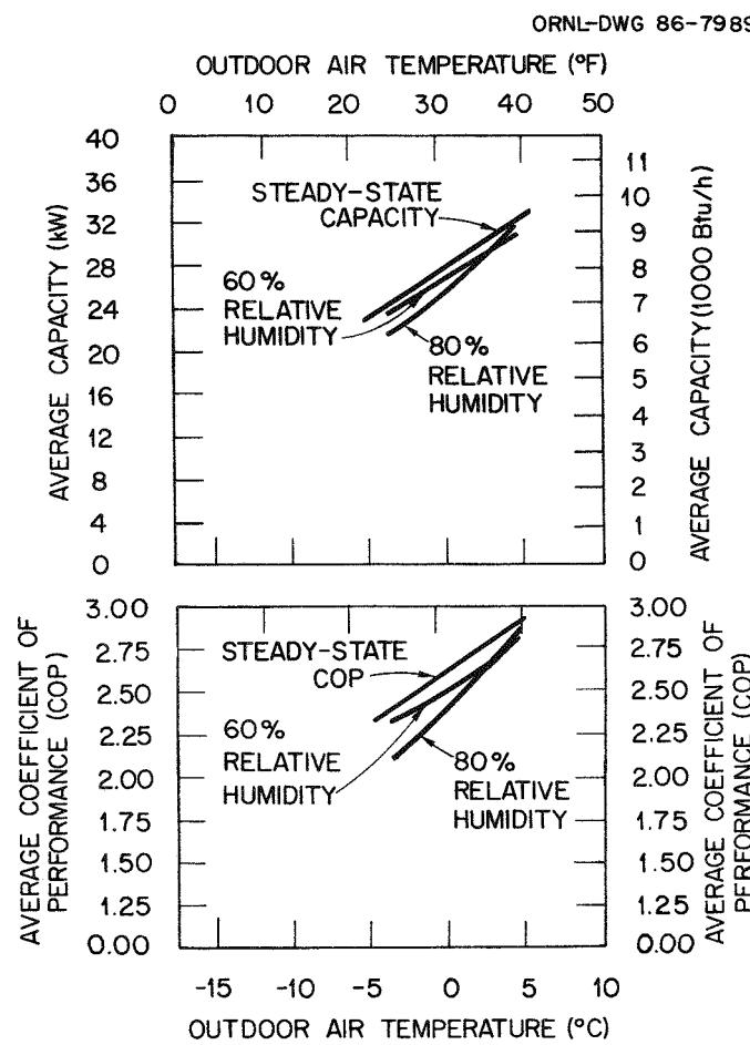
Fig. 8.3. Average frosting COP and capacity integrated over the frosting and recovery intervals.
