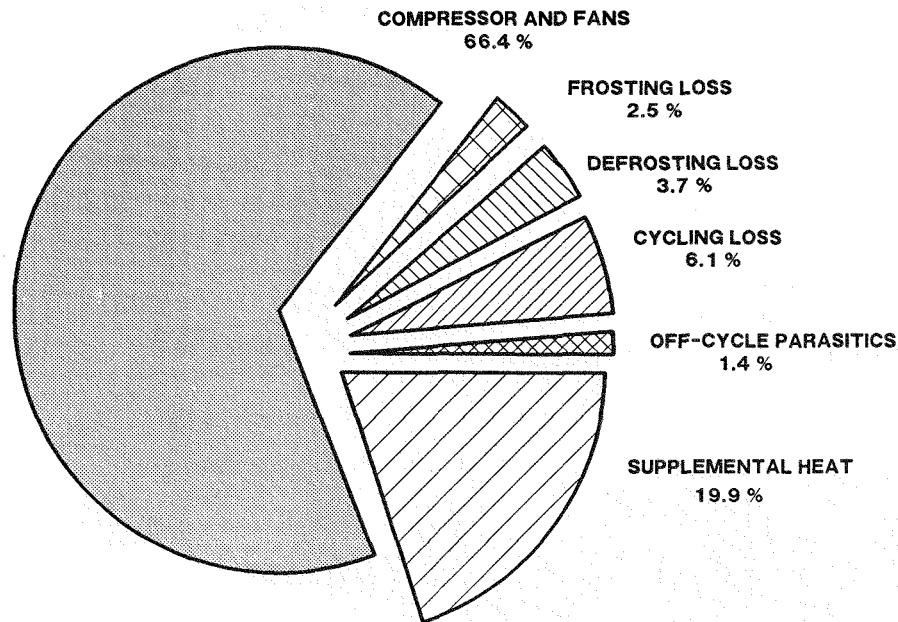
Fig. 8.5. Portions of energy as a percentage of total yearly energy for the test heat pump (with demand defrost initiator) operating in Syracuse, New York.
