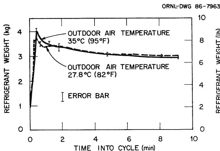
Fig. 7.11. Refrigerant weight measured in the outdoor unit for cycling tests conducted at  $28^{\circ}\text{C}$  ( $82^{\circ}\text{F}$ ) and  $35^{\circ}\text{C}$  ( $95^{\circ}\text{F}$ ) outdoor temperatures.
