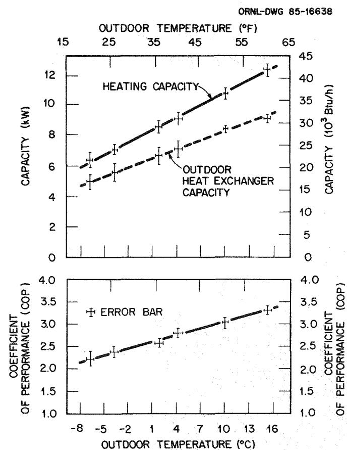
Fig. 5.1. Steady state system performance measured at a constant indoor temperature of  $21.1^{\circ}\text{C}$  ( $70^{\circ}\text{F}$ ).
