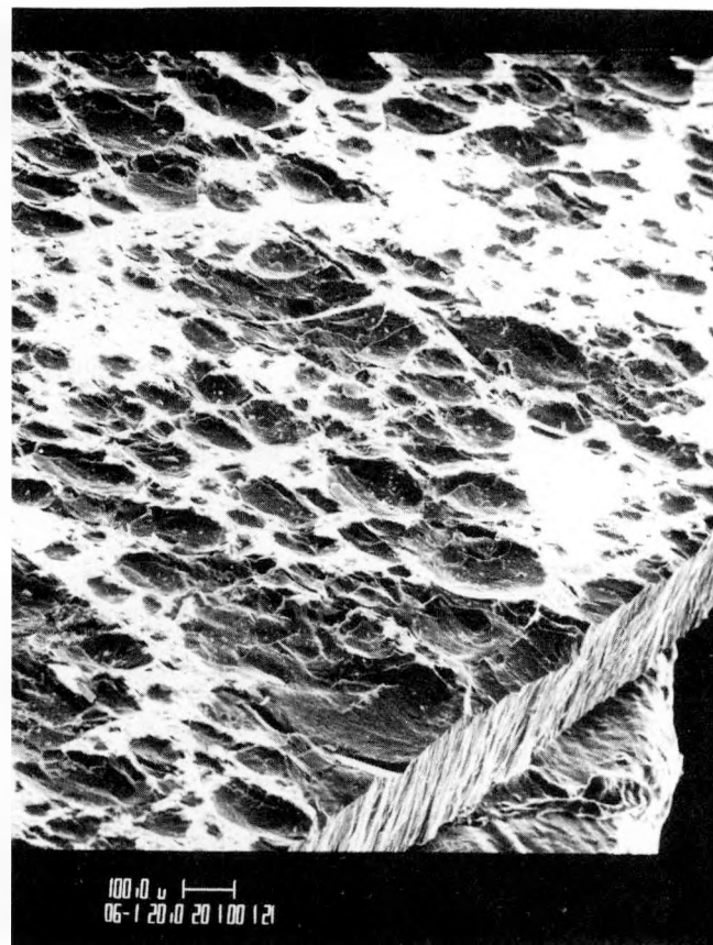
Sheared surface of silicon ribbon 60X
