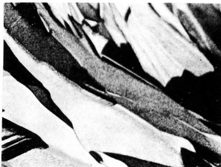
FIGURE 44: MICROSTRUCTURE NEAR THE RIGID EDGES IN THE RIBBON SHOWN IN FIGURE 43. 200X
