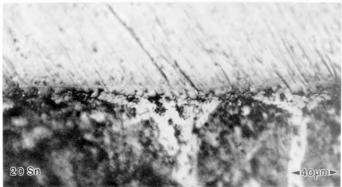
Figure 3.28. Double \text{Cu}_6\text{Sn}_5 ( \eta ) and \text{Cu}_3\text{Sn} ( \epsilon ) intermetallic layers in a) 40Sn-60Pb and b) 20Sn-80Pb double shear specimen solder joint interfaces. The dark, thin layer more easily seen in (a) adjacent to the Cu is \epsilon while the elongated whiskers growing into the solder are \eta .
