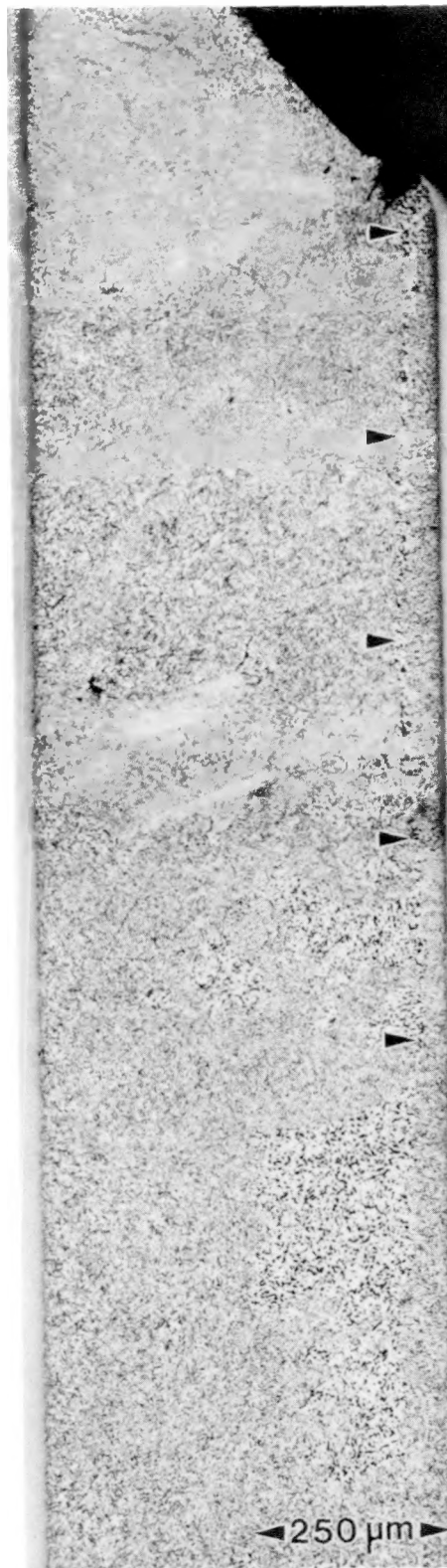
Figure 3.15. Coarsened band running along a 6-month old 63Sn-37Pb solder joint fatigued at 75°C with a 10% strain range to 30% load drop. XBB 898-6545B
