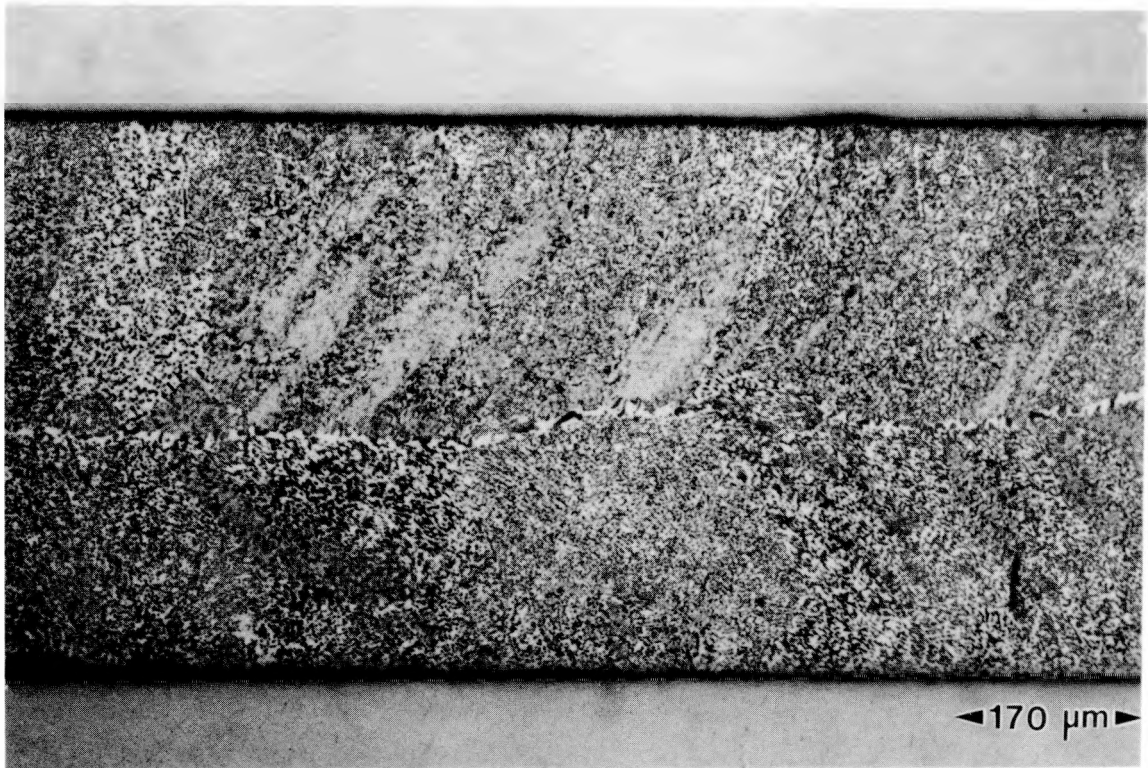
Figure 2.16. Coarsened band which formed along colony boundaries in a eutectic Sn-Pb solder joint isothermally fatigued with a 10% strain range at 75°C.
