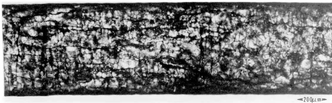
Figure 3.30. Deformation patterns formed in the Pb-rich a) 20Sn-80Pb and b) 5Sn-95Pb alloys. The double shear specimens were polished to 0.05\mu\text{m} , fatigued with approximately a 10% strain range at 75^\circ\text{C} and observed optically with no post-fatigue surface preparation.
