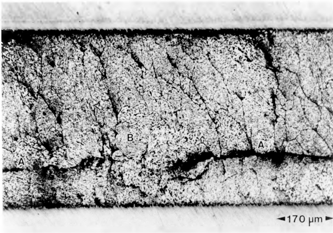
Figure 2.11. Surface relief showing nonuniform deformation following creep of a 63Sn-37Pb solder joint. In some regions of the joint (A), long straight shear bands form allowing a great amount of deformation to concentrate there. In other regions (B), no colony boundaries line up to form fairly straight paths parallel to the direction of the applied shear strain.
