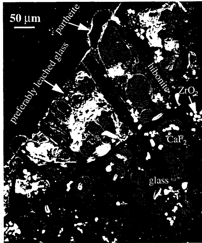
Figure 3.65. A Cross-Section SEM Micrograph Showing the Surface Layer Structure of LVC-14 After Vapor Hydration Testing
