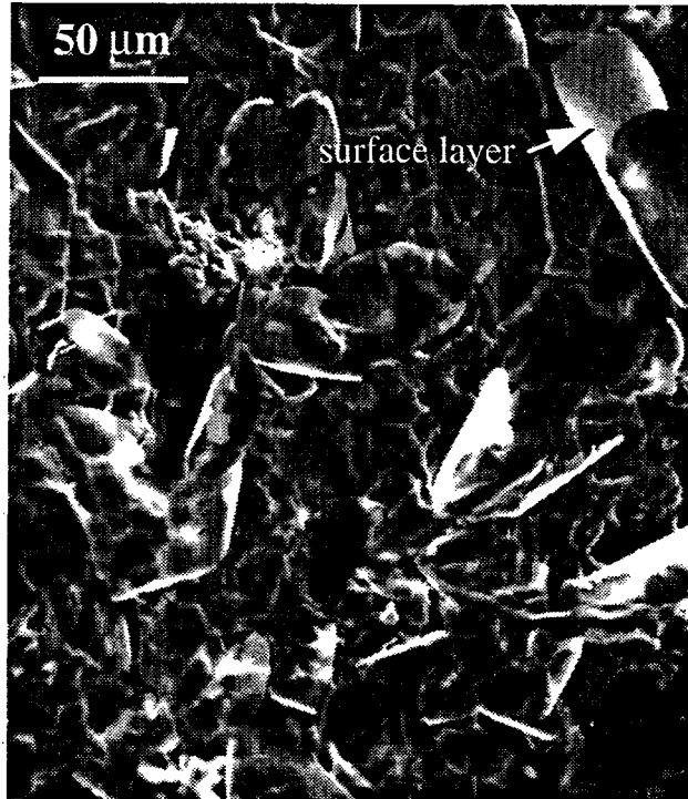
Figure 3.60. SEM Micrograph Shows a Thin Crust Developed on LVC-7 After Vapor Hydration Testing
