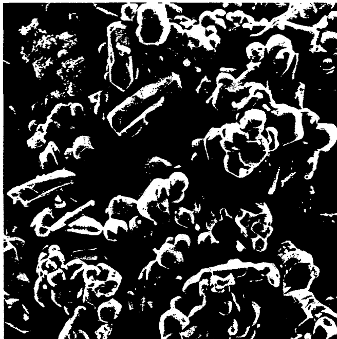
Fig. 3. SEM of \beta -Si 3 N 4 seed material E3/Pwd.
