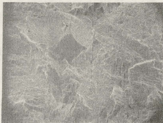
Figure 9. Typical Fracture Surface of a Martensitic Specimen After Fatigue in Air.
