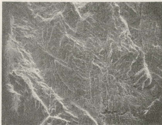
Figure 7. Herringbone Transgranular Failure of Bainitic Specimen After Air Fatigue.
