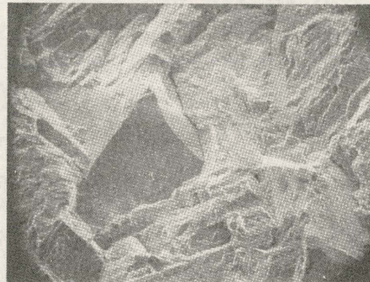
Figure 10. Fracture Surface of a Martensitic Specimen Fatigued in 6.9 MPa H 2 .
