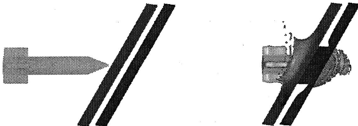
Figure 6. Simulation of a finned tungsten projectile obliquely impacting a stainless steel plate (hydrodynamic constitutive model).
