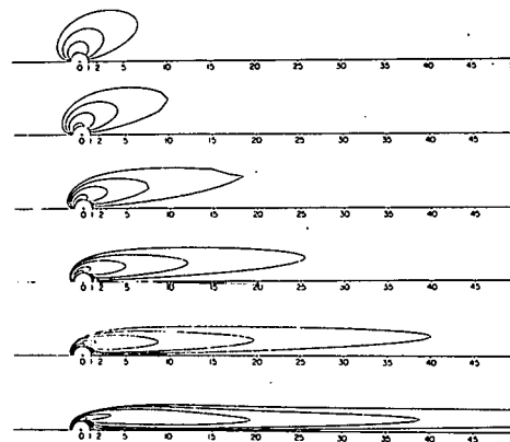
Fig. 6. Lines of equal vorticity at Re = 2, 4, 10, 20, 40 and 100 . (The first three cases were obtained by a different method).
