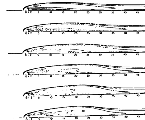
Fig. 7. Lines of equal vorticity at Re = 200, 230, 260, 290, 295 and 300 .
