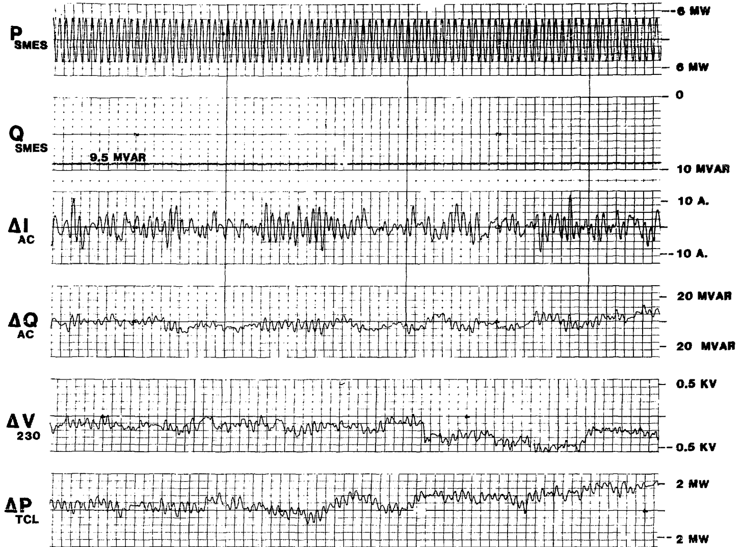
Fig. 4. Response of ac system to SMES unit modulation.
